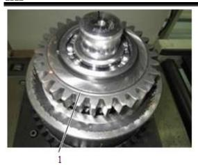
3. Use a crowbar to separate gear from the clutch.
