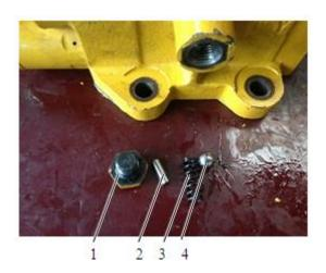
3. Successively remove O-ring, locating guide rod, spring and steel ball.
