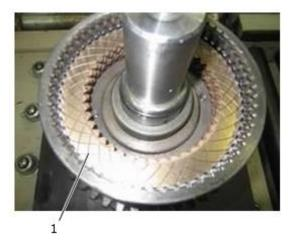
7. Successively remove the outer friction lining, and then the inner friction lining.
