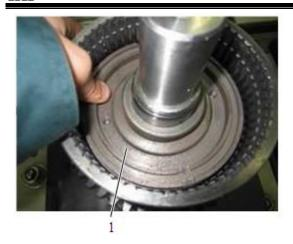
2. Put the piston into the clutch.
