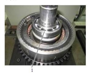
4. Remove the bearing with a crowbar.
