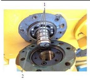
Fig. 3-6 1. Seal ring 2. Gasket
