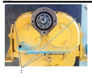
Remove the mounting bolt of transmission big end cap. Install the jackscrew into the mounting hole of housing end cap to eject the big end cap out.
