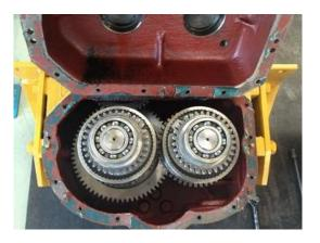
10. Remove the transmission big end cap and paper gasket.
