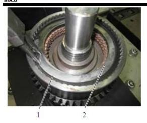
Remove the retainer ring with a pair of snap ring pliers. Remove the bearing plate of clutch friction lining.
