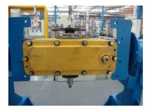
16. Remove bolts, and take off the oil sump and the gasket.
