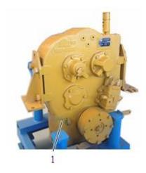
1. Place the transmission on the maintenance support.
