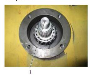
25. Remove the output shaft assembly from the front side of transmission.
