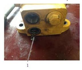
7. Take out the shut-off valve spring and the valve core.
