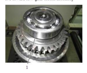
1. Remove the bearing with a crowbar.
