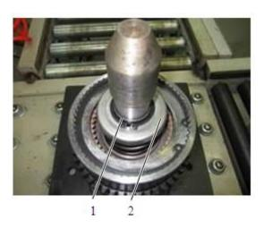
5. Press the spring shield with a crowbar, and remove the retainer ring with a pair of snap ring pliers. Remove the spring shield and the spring.
