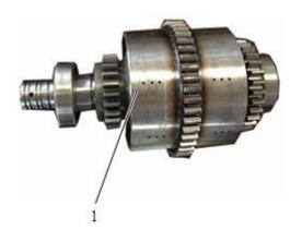
Fig. 3-271. Forward low-gear clutch assembly
