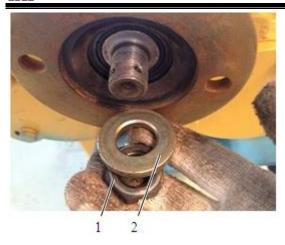
3. Remove the cotter pin from the tightening nut of input flange with a pair of pliers. Remove the tightening nut of input flange, and take off the pressure plate.
