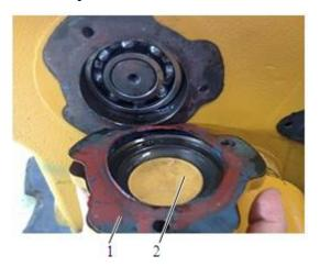
13. Remove the bolts from the countershaft pressure cap, slightly strike the pressure cap with a recoilless hammer, remove it and the gasket, and place them aside.
