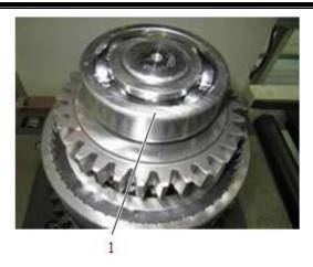
11. Install the bearing onto the clutch shaft in position.
