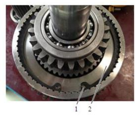
Fig. 4-12 1. Retainer ring 2. Bearing plate
