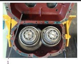
7. Install the housing big end cap and the gasket.
