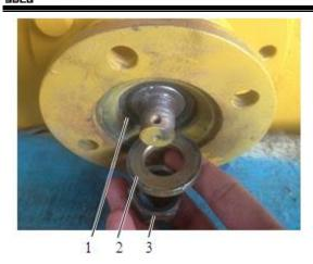
4. Fit the cotter pin to the fixing nut onto the output shaft front output flange.
