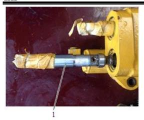
4. Take out the forward & reverse control valve core.
