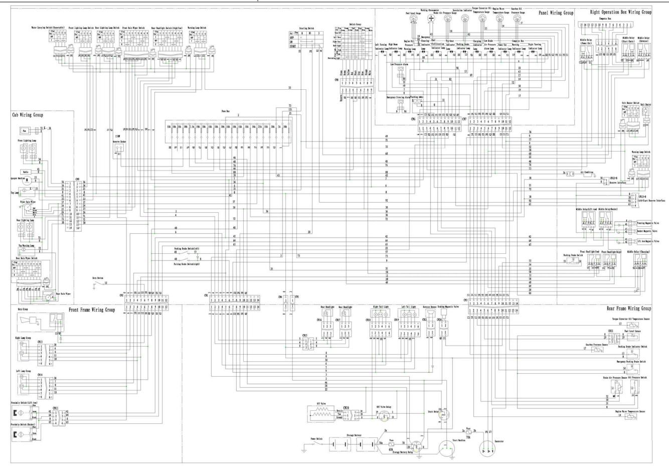
Figure 5-8 LG958L Electric System Principle Diagram with Shangchai Engine
