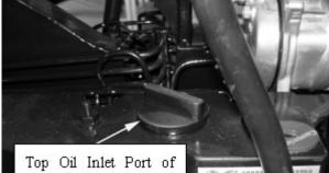
• Then put back the oil dipstick and close the profile door of the engine. For choosing the appropriate oil please refer to **CHAPTER IV 2.2 Oil Selection.**
