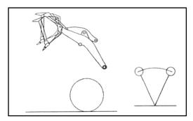
dumped by the lever control. Act slowly and gently during dumping to prevent the bucket from striking the ground.
