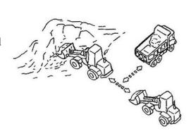
after digging a full load and lets the auto-unload truck move into the position between material and the loader. This method costs the minimum time and can reduce the cycle time most effectively.
