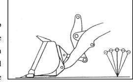
the lever at the raising or lowering position to ensure pushing the bucket smoothly.
