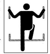
• **Never** hold any tools or other items when climbing up and down the loader; lift the tools needed to the operation flat roof by rope.
