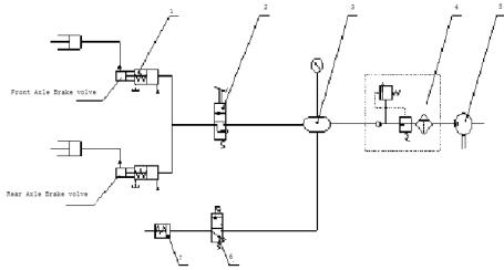
1. Air Booster Pump 2. Air Brake Valve 3. Air Tank
