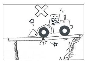
Don't use the machine for any work other than what the machine is designed for. It may damage the parts or cause an accident when using the head of the working equipment for other fuctions, such as hook, grasp, draw, push, or tow.
