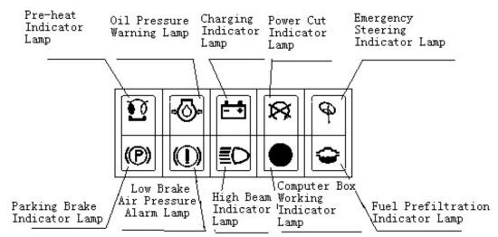
**Pre-heat Indicator Lamp:** The lamp will come on if start switch is turned to preheat position when machine is equipped with cold start equipment; the lamp will be off if start switch is turned to other position.
