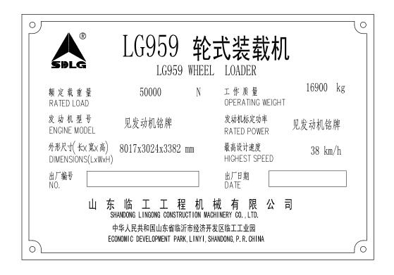
Figure 2-8 Nameplate of LG959 basic configuration loader
