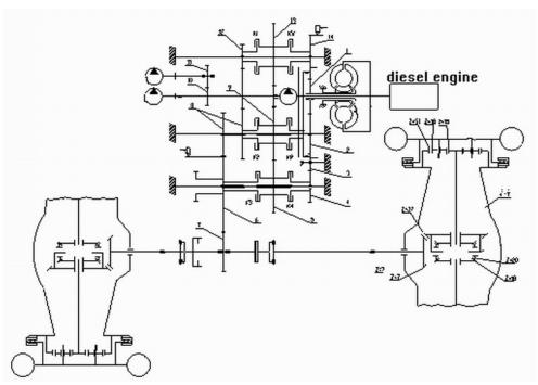
1.Input Gear 2. KR Reversing Gear 3.Mid-Axle Gear 4. 4<sup>th</sup> Gear 5. K34 Gear Ring 6. 3<sup>rd</sup> Gear 7. Output Gear 8. 2<sup>nd</sup> Gear Group 9. KR2 Gear 10. Working Pump Driving Gear 11. Steering Pump Driving Gear 12. 1<sup>st</sup> Gear 13. KV1 Gear 14. KV Reversing Gear Figure 5-1 Transmission System Diagram
