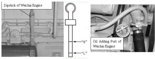
■ Shangchai C6121ZG50. It is a suitable oil level if it is between the adding oil graduation line and the oil static full graduation line. If the oil level is lower than the adding oil graduation line, oil should be added by the oil adding port.
