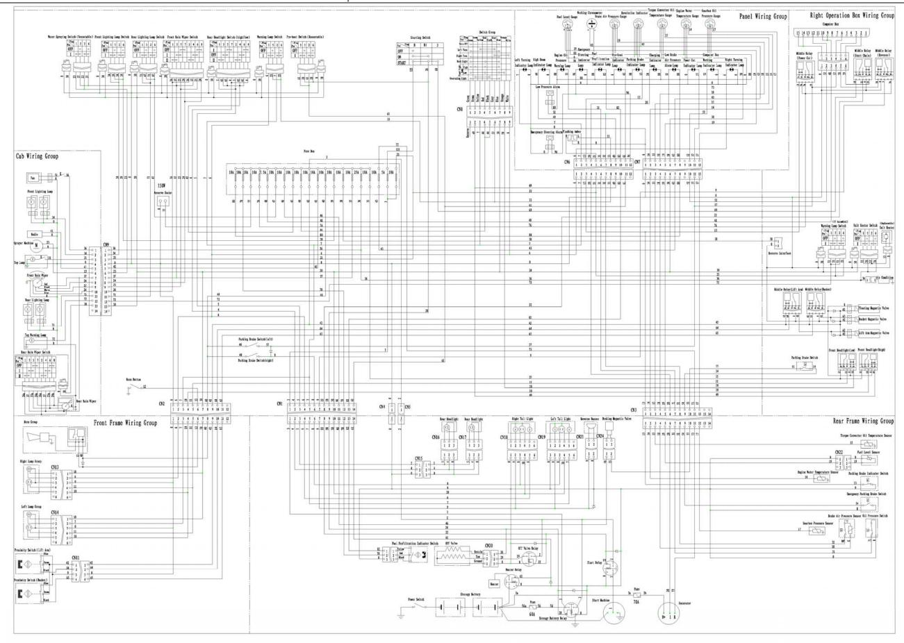
Figure 5-7 Electric System Principle Diagram with Cummins Engine
