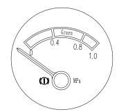
❖ If the pressure index lies in the range of (4~8)×100kPa or (5.8~11.6)×10PSI, the oil pressure is normal. Be sure to stop the machine for inspection if the index moves outside this range.
