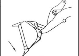
ground, put the lift arm control lever in the float position; for soft ground, put the lift arm control lever in the neutral position.
