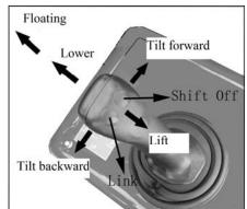
is in the bucketing position in order to realize the set level automatically function and increase the efficient of the whole vehicle.
