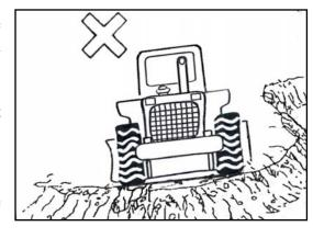
• Never drive the machine near hanging things or close to a deep ravine. The machine weight or
