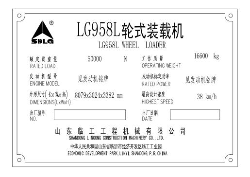
Figure 2-4 Nameplate of LG958L basic configuration loader
