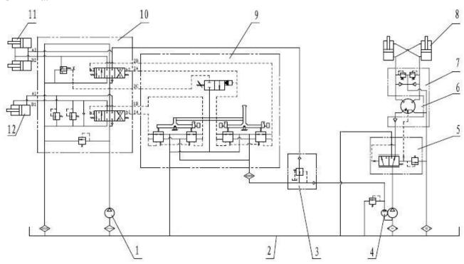
Work Pump 2. Hydraulic Oil Tank 3. Pressure Oil Tank 4. Pair Pump 5. Priority Valve
