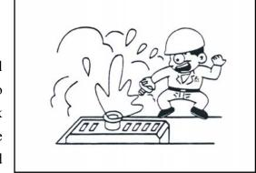
water in the engine, the oil and water in the radiator may be still very high after just finishing the work. Wait for the temperature falling down and follow the procedures to do the operations above.
