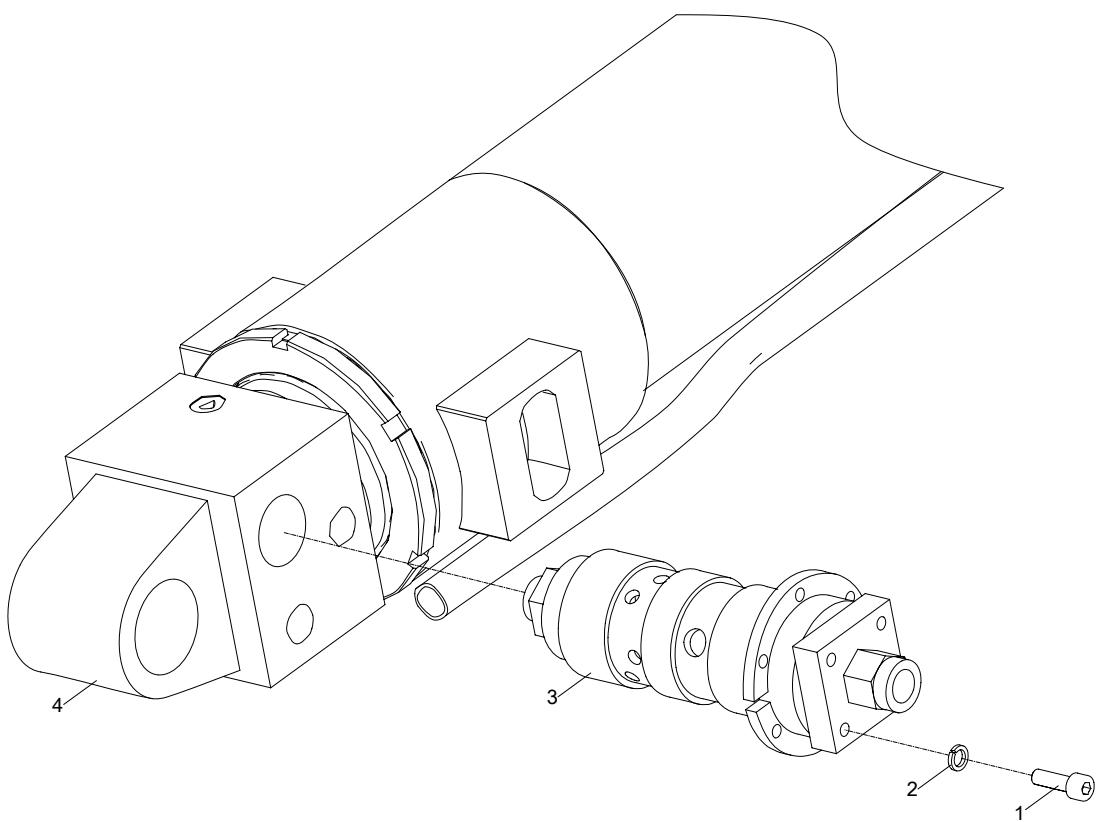
**TELESCOPING BALANCE VALVE INSTALLATION
