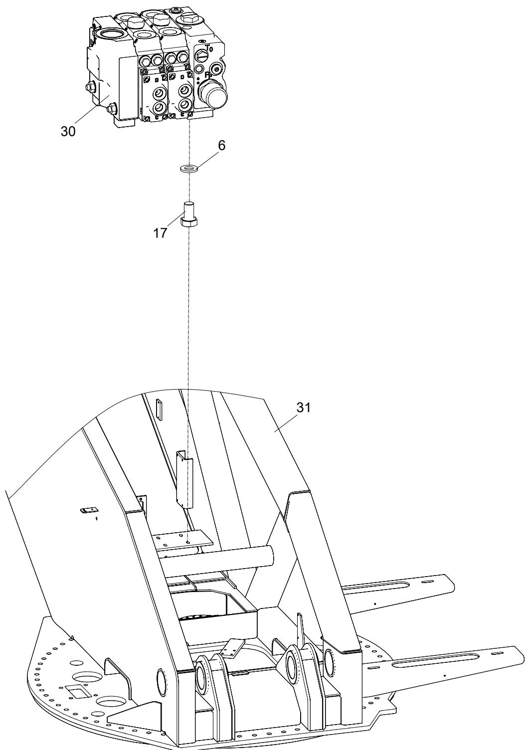
**TURNTABLE VALVE INSTALLATION(WINCH VALVE INSTALLATION)
