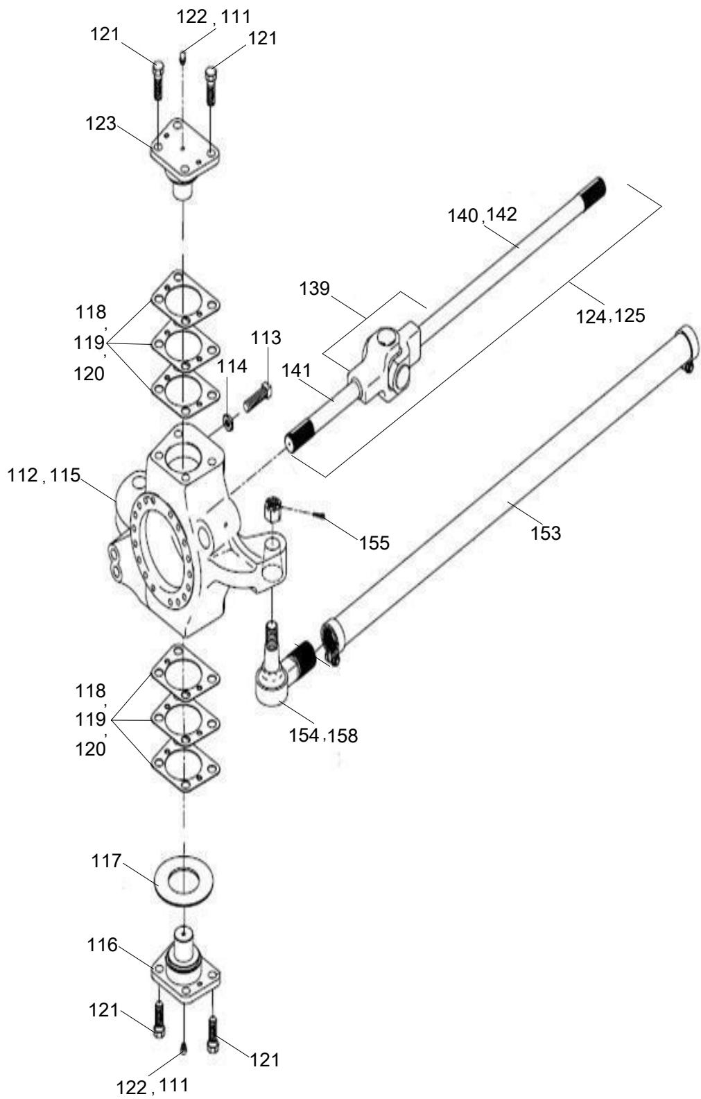
**FRONT AXLE(HUB REDUCER ASSY. EXPLODED VIEW II)**
