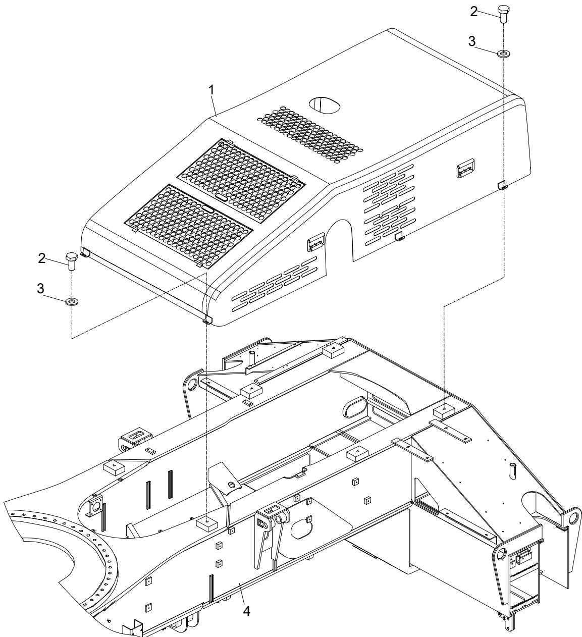
**ENGINE HOUSING AND ITS INSTALLATION
