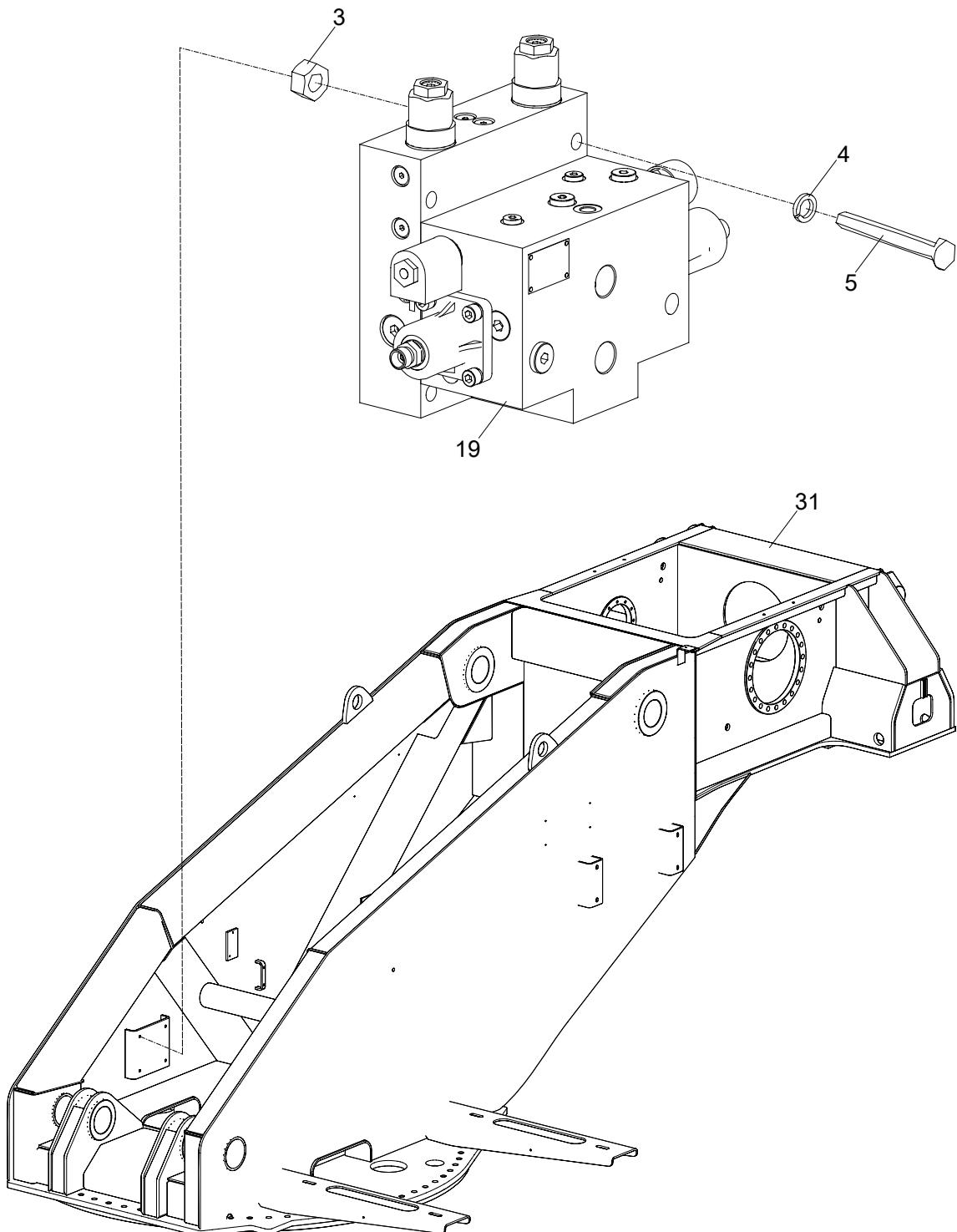
**TURNTABLE VALVE INSTALLATION(SLEWING CUSHION VALVE INSTALLATION)
