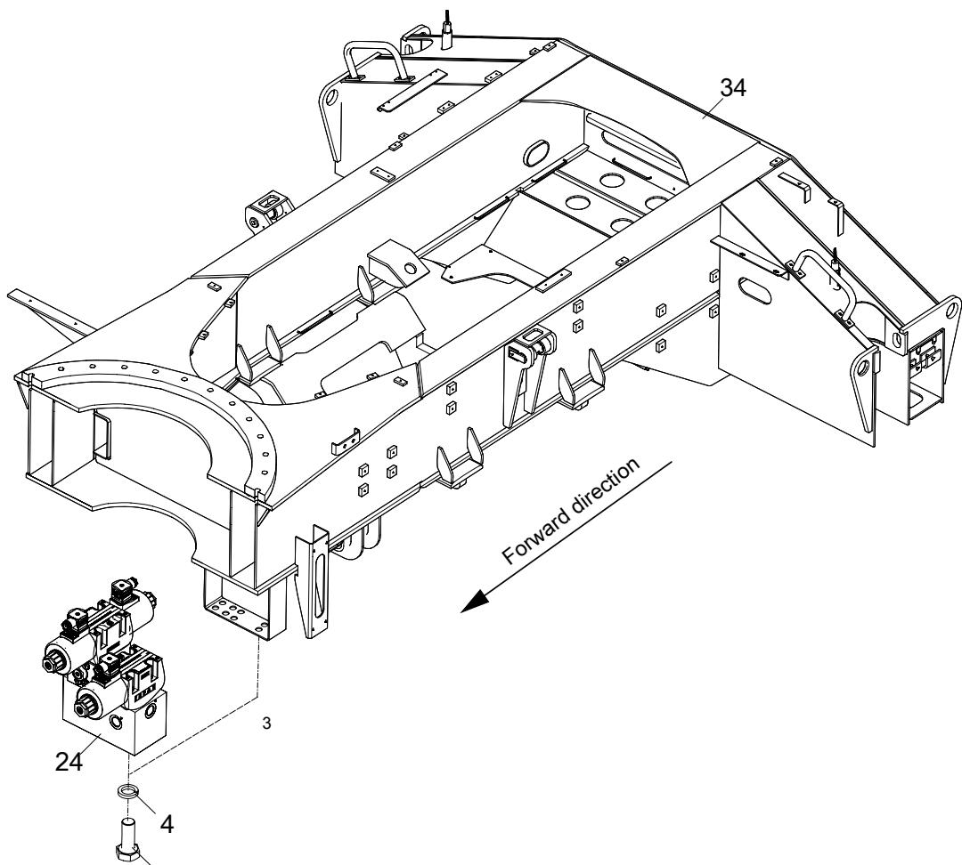
**CHASSIS FRAME VALVE INSTALLATION(STEERING CONTROL VALVE
