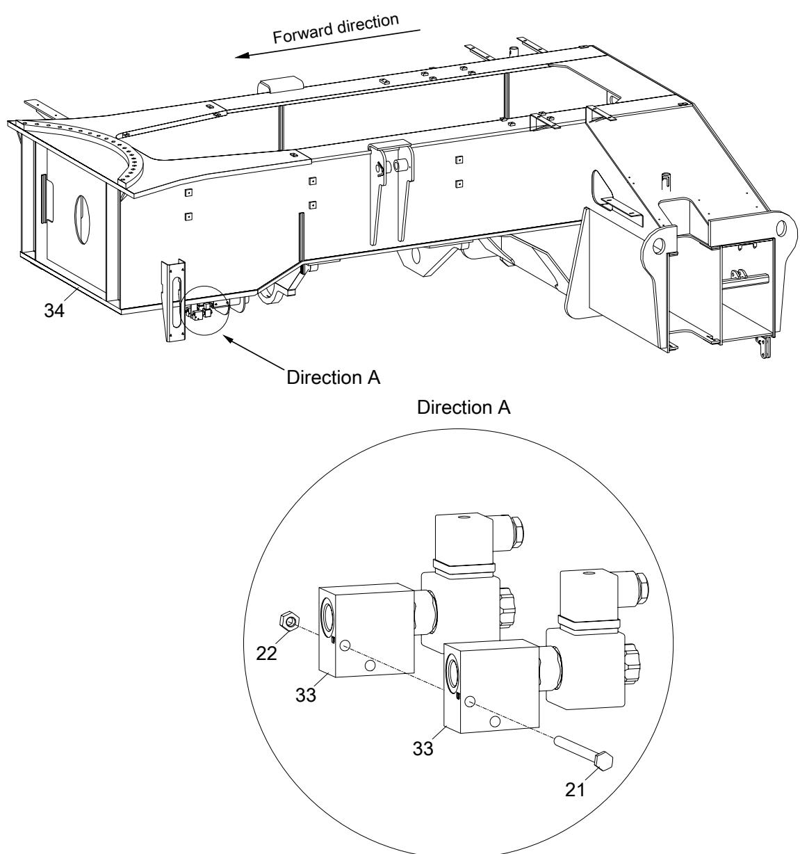
**CHASSIS FRAME VALVE INSTALLATION(LOCKING SOLENOID VALVE
