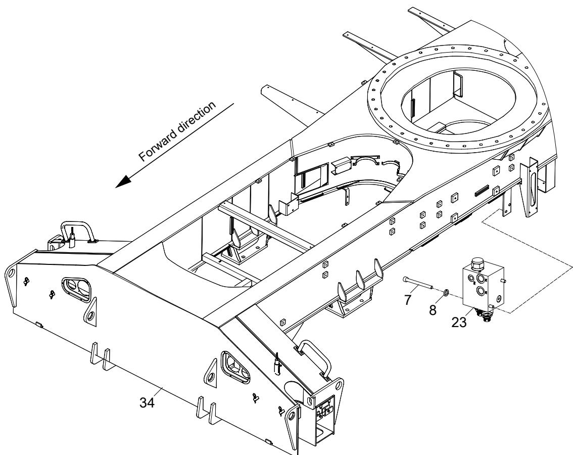
**CHASSIS FRAME VALVE INSTALLATION(RELIEF CONTROL VALVE
