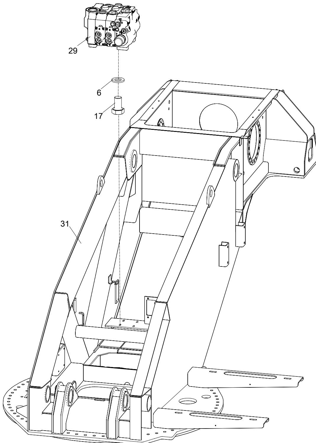
**TURNTABLE VALVE INSTALLATION(TELESCOPING DERRICKING VALVE
