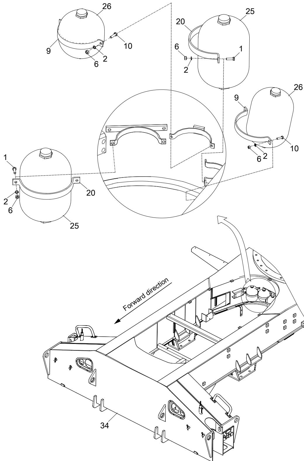
**CHASSIS FRAME VALVE INSTALLATION(ACCUMULATOR INSTALLATION)**
