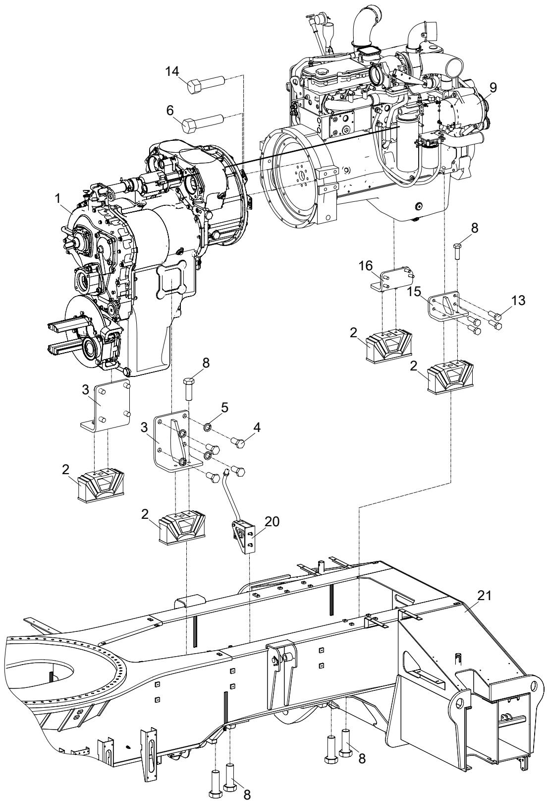
**ENGINE AND TRANSMISSION INSTALLATION**
