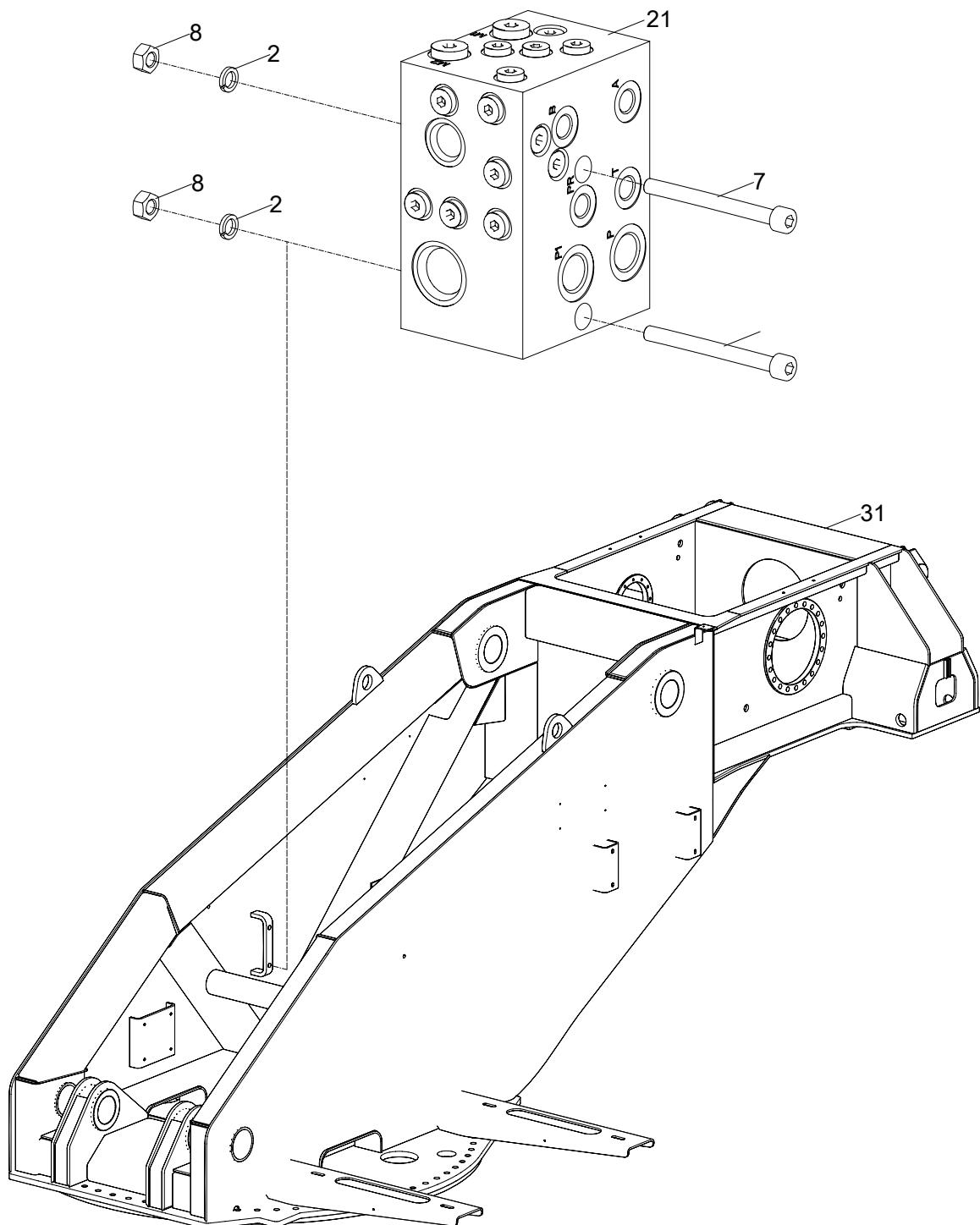
**TURNTABLE VALVE INSTALLATION(SOLENOID CONTROL VALVE INSTALLATION)
