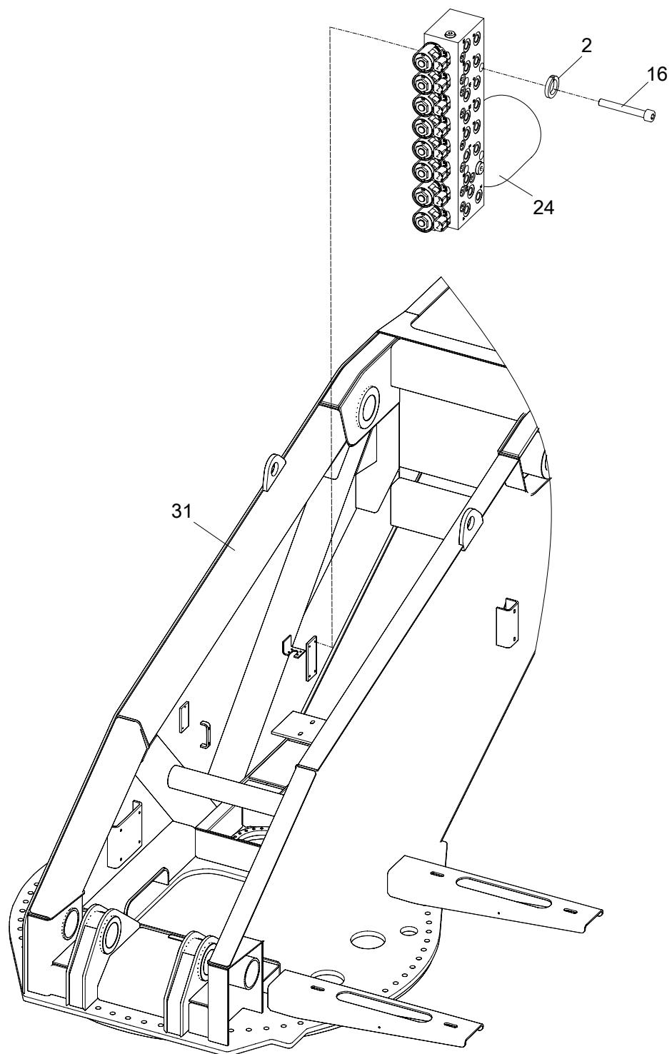
**TURNTABLE VALVE INSTALLATION(PILOT-OPERATED CONTROL VALVE BLOCK INSTALLATION)D00756304811000000Y**
