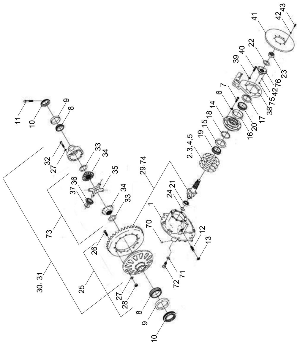
**FRONT AXLE(MAIN REDUCER ASSY. EXPLODED VIEWI)**
