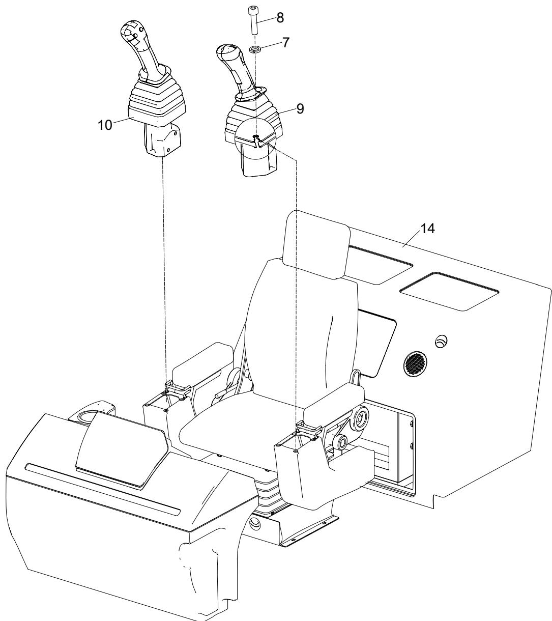
**CAB VALVE INSTALLATION(PILOT-OPERATED CONTROL JOYS INSTALLATION)
