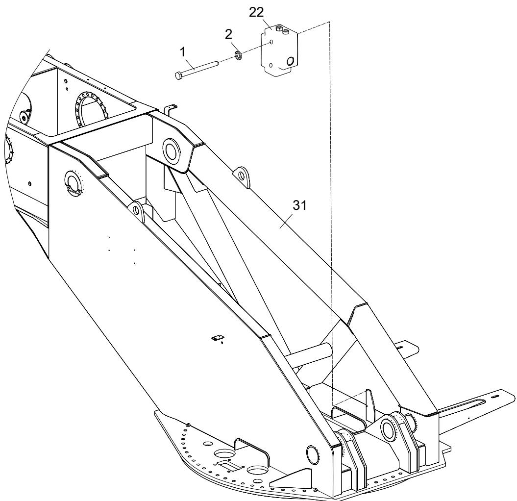
**TURNTABLE VALVE INSTALLATION(PRIORITY VALVE INSTALLATION)
