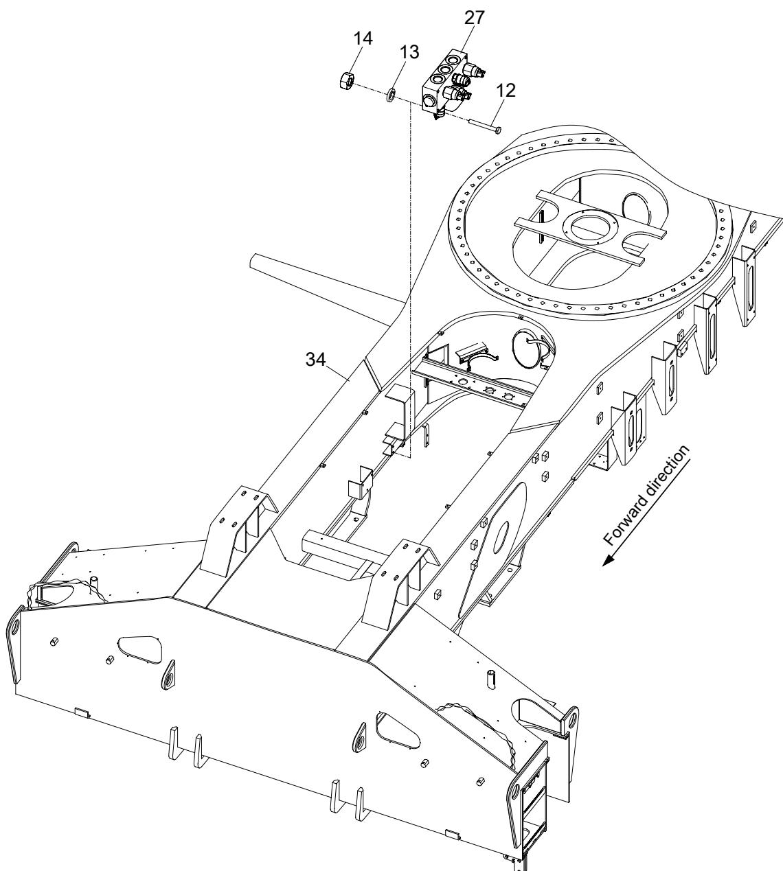
**CHASSIS FRAME VALVE INSTALLATION(BRAKE VALVE ASSY. INSTALLATION)
