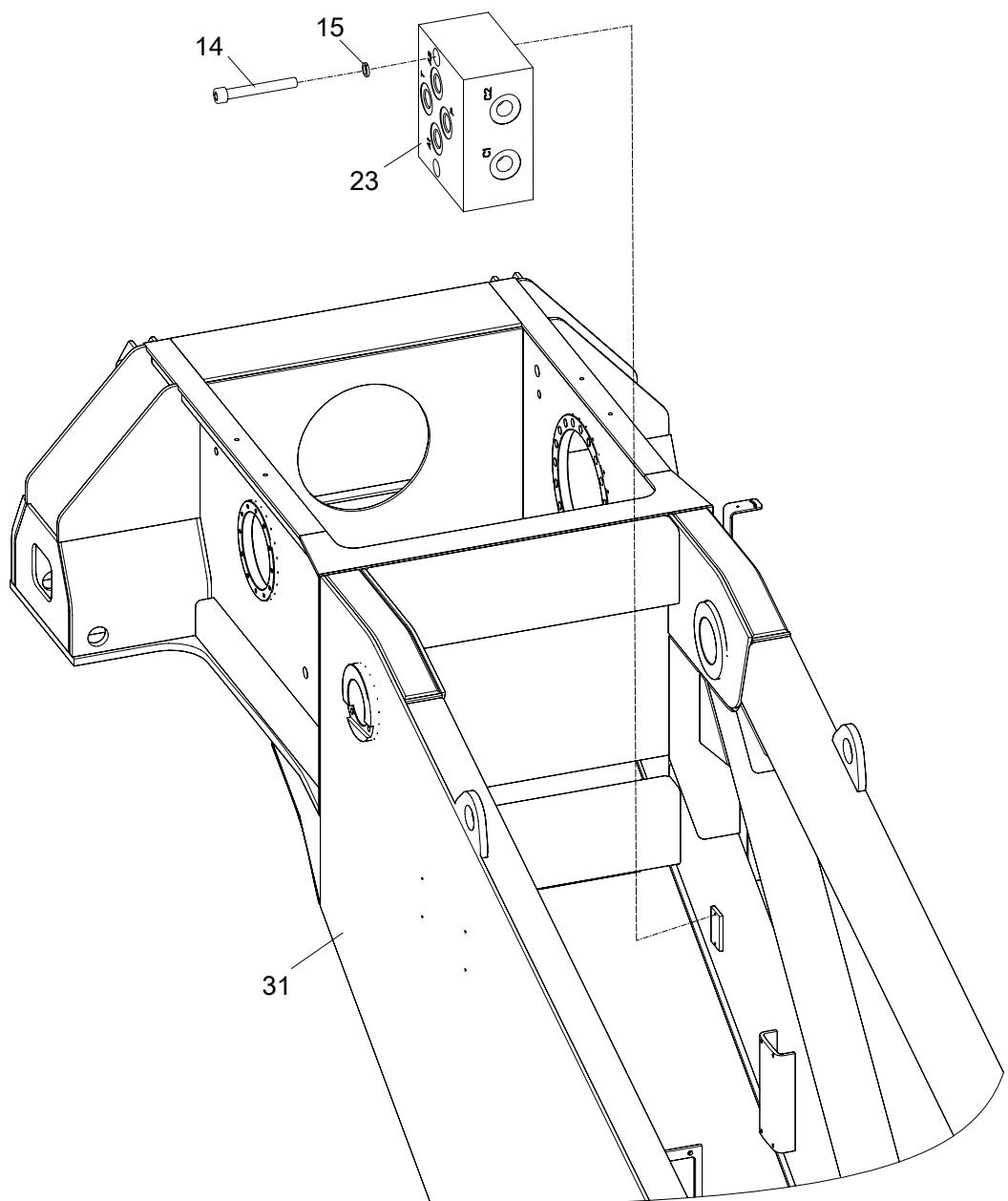
**TURNTABLE VALVE INSTALLATION(PILOT-OPERATED VALVE INSTLLATION)**
