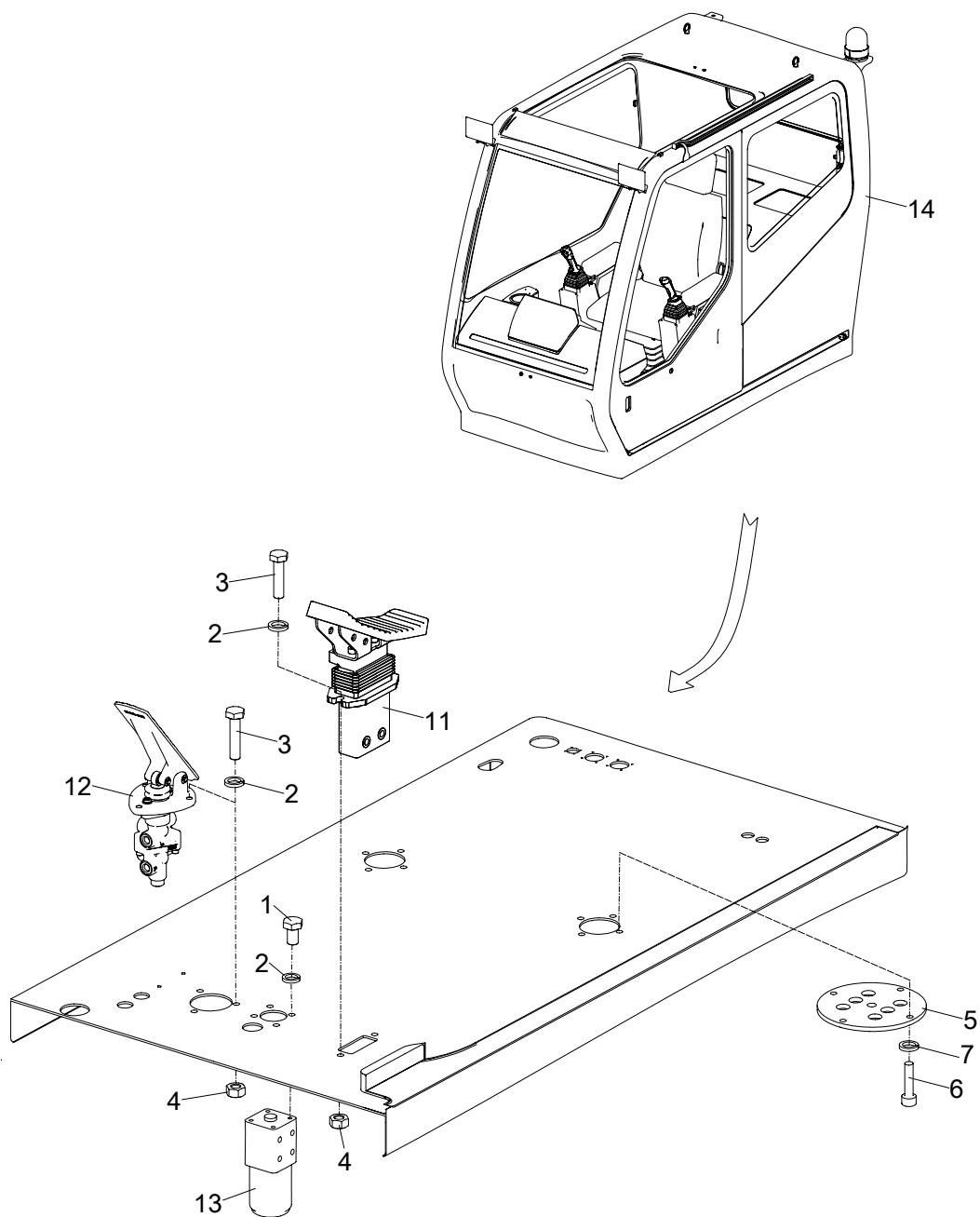
**CAB VALVE INSTALLATION(FOOT-OPERATED INSTALLATION)**
