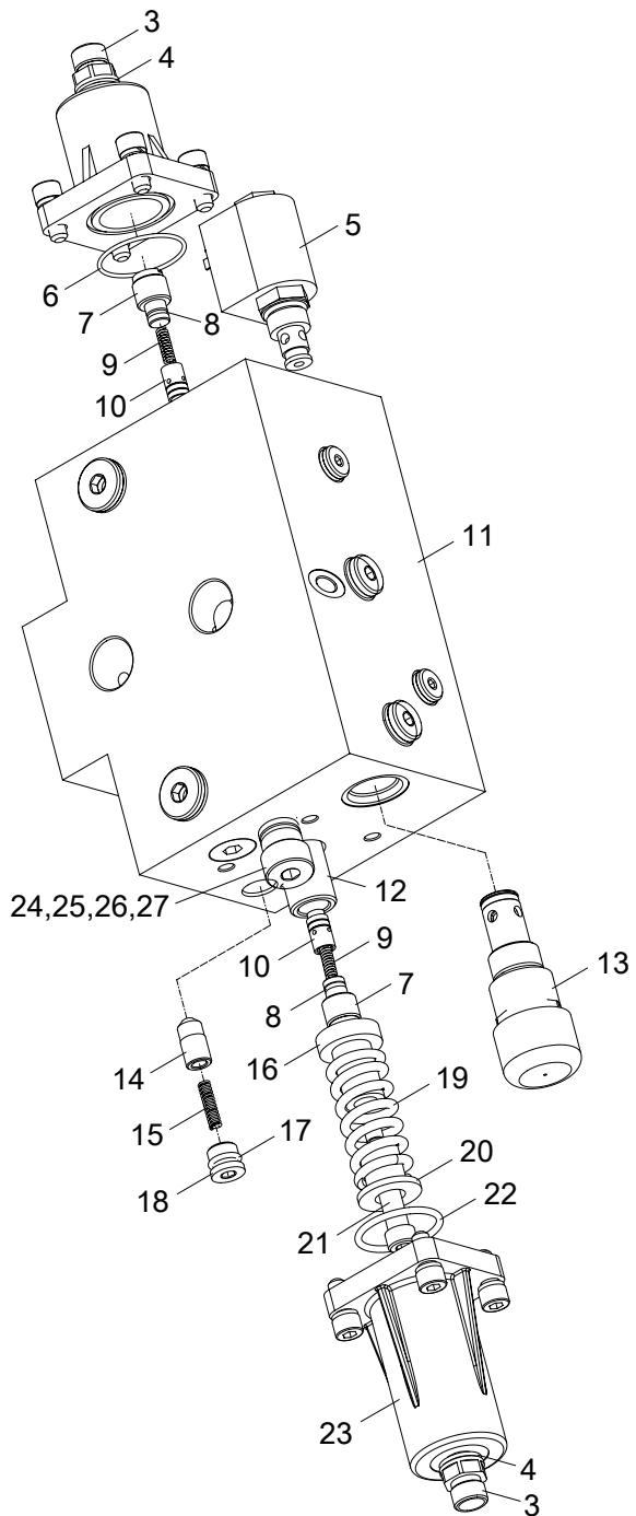
**SLEWING CUSHION VALVE(PILOT-OPERATED DIRECTIONAL CONTROL VALVE)**
