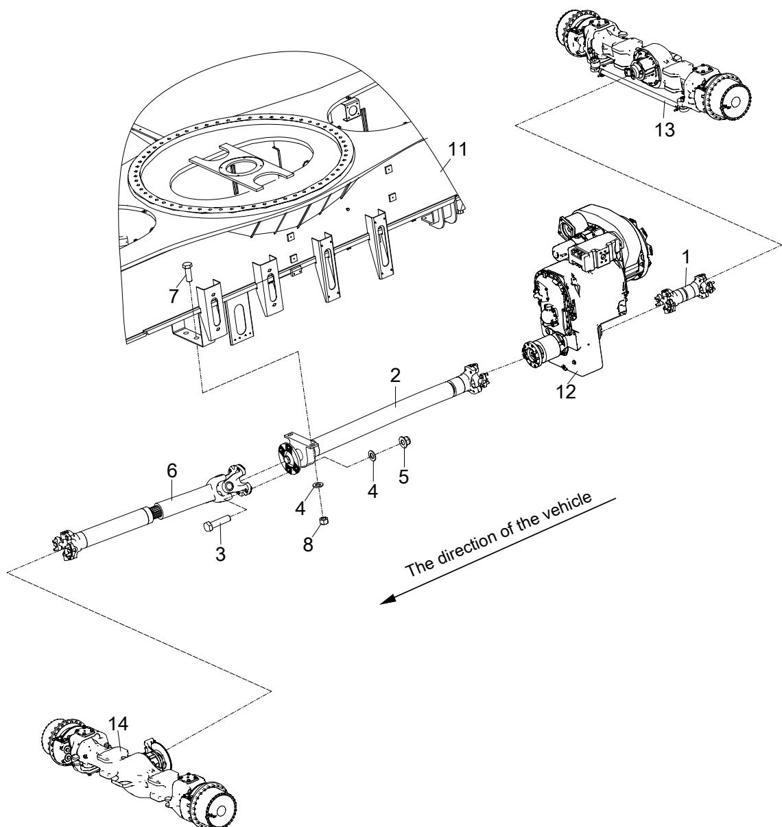
**PROPELLER SHAFT ASSEMBLY
