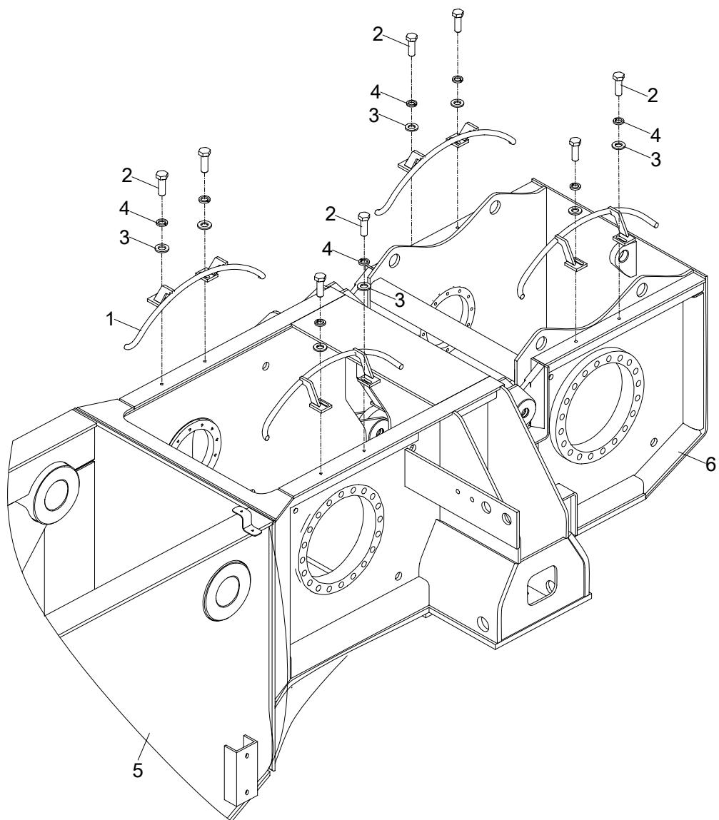
**ROPE GUARD BRACKET INSTALLATION
