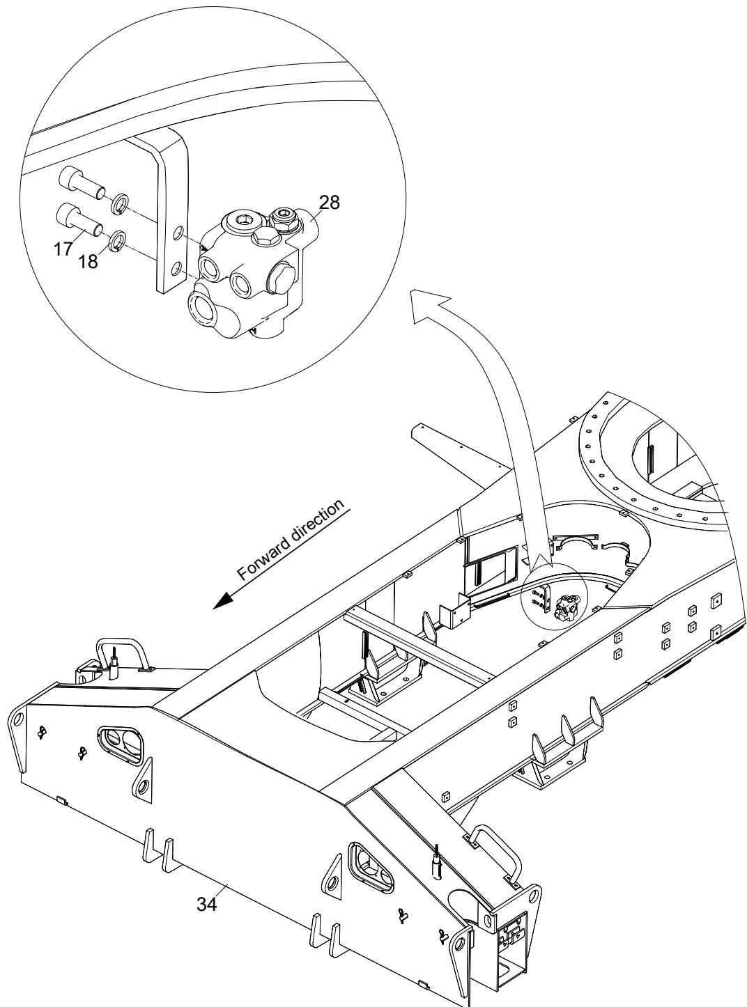
**CHASSIS FRAME VALVE INSTALLATION(FLUID FILLING VALVE INSTALLATION)
