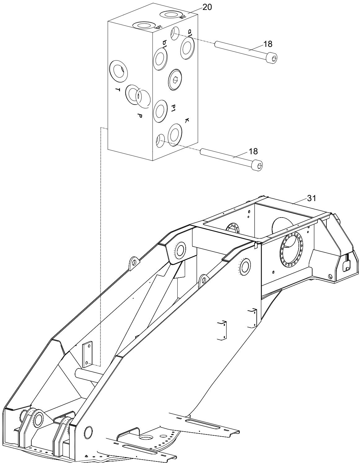
**TURNTABLE VALVE INSTALLATION(SLEWING BRAKE VALVE INSTALLATION)
