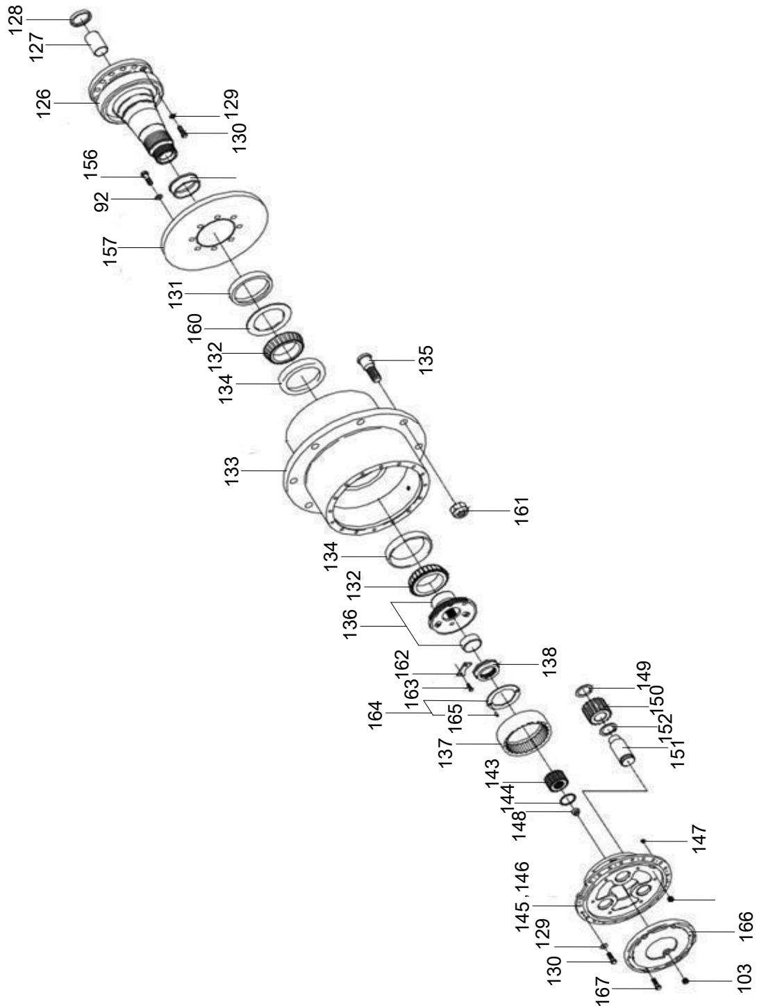
**FRONT AXLE(HUB REDUCER ASSY. EXPLODED VIEW I)**
