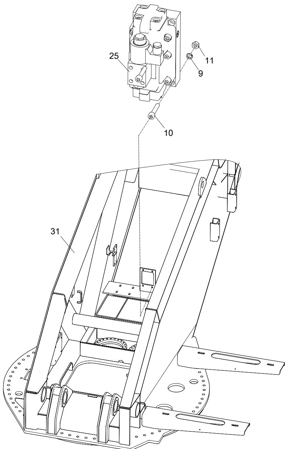
**TURNTABLE VALVE INSTALLATION(ELECTRO-HYDRAULIC DIRECTIONAL
