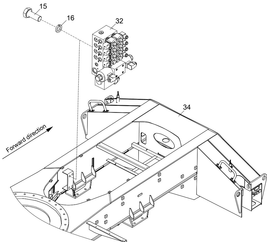
**CHASSIS FRAME VALVE INSTALLATION(OUTRIGGER CONTROL VALVE BLOCK INSTALLATION) D00756304810800000Y**
