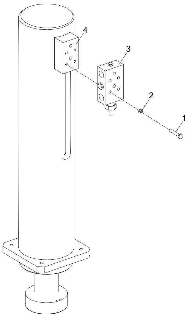
**COUNTERWEIGHT BALANCE VALVE INSTALLATION
