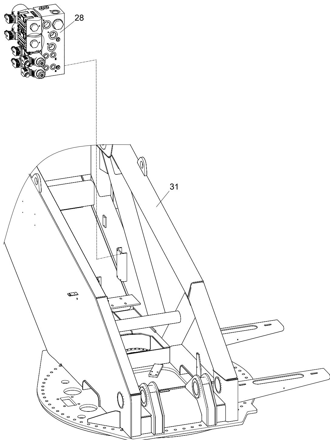
**TURNTABLE VALVE INSTALLATION(SOLENOID VALVE BLOCK INSTLLATION)
