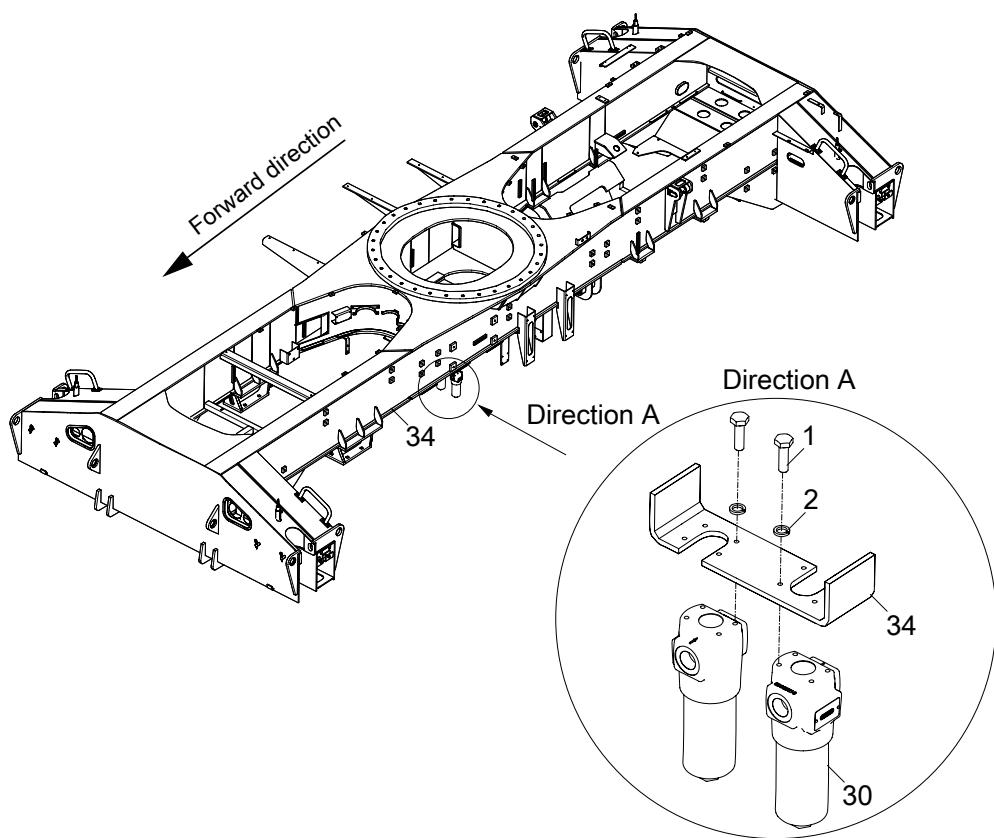
**CHASSIS FRAME VALVE INSTALLATION(HIGH-PRESSURE OIL FILTER INSTALLATION) D00756304810800000Y**
