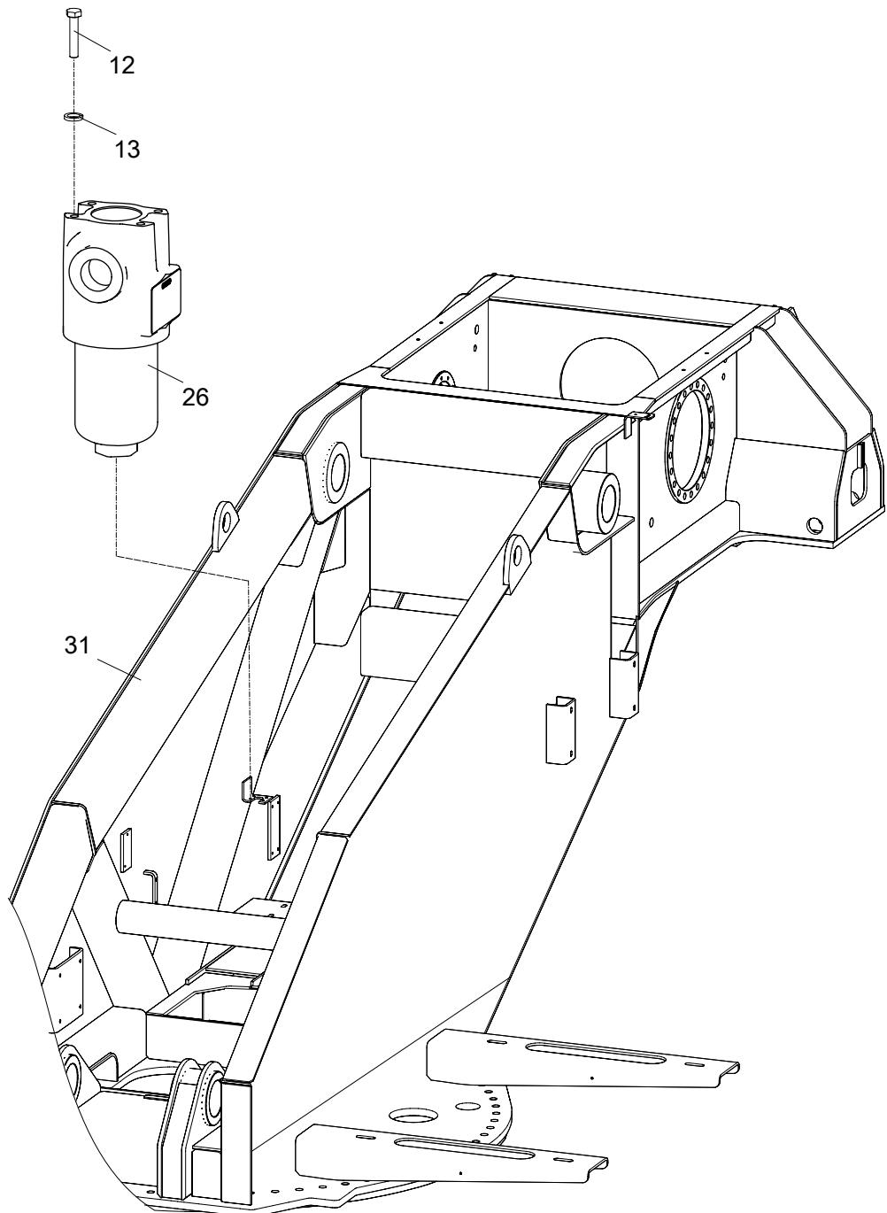
**TURNTABLE VALVE INSTALLATION(PIPE FILTER INSTALLATION)**
