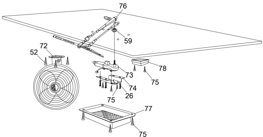
**DRIVER'S CAB(ROOF WIPER SYSTEM AND FAN)**
