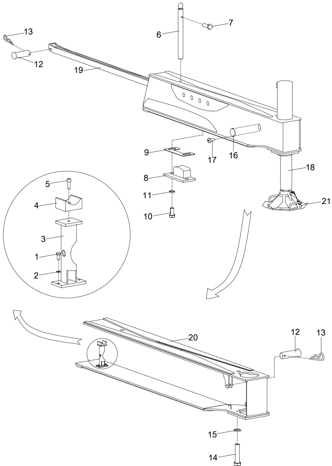
**OUTRIGGER AND ITS CYLINDER INSTALLATION
