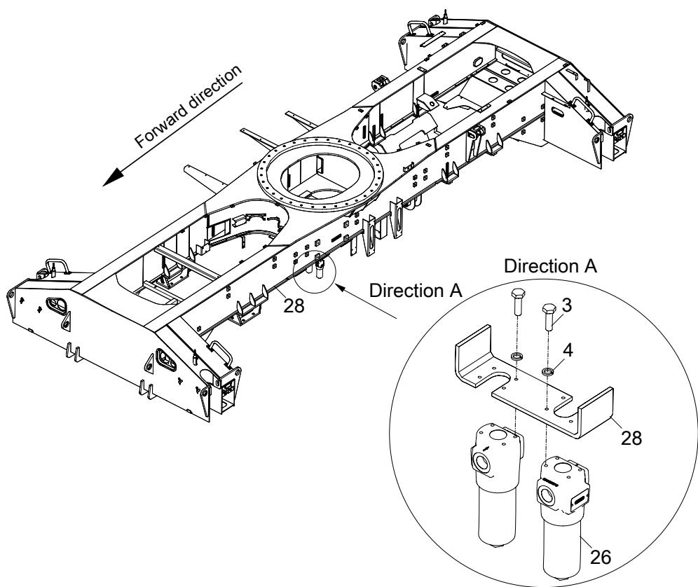
**CHASSIS FRAME VALVE INSTALLATION(HIGH-PRESSURE OIL FILTER
