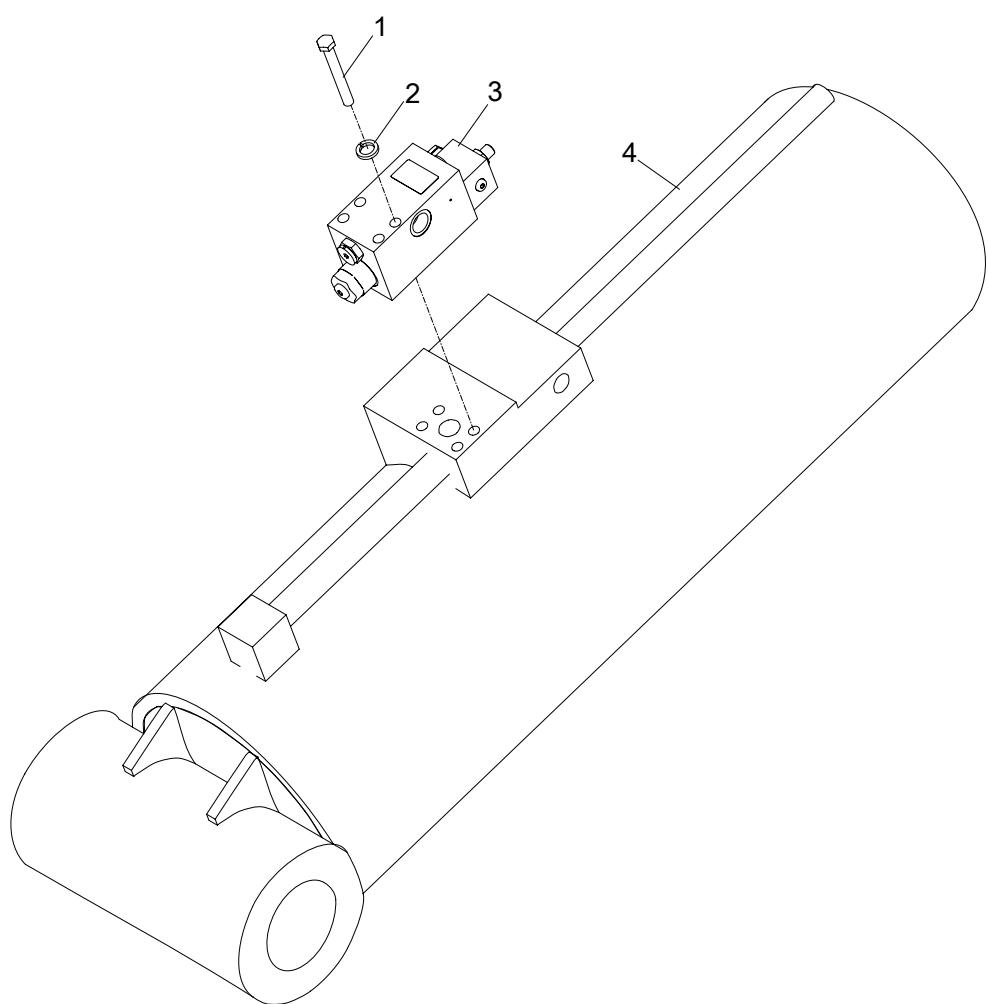
**DERRICKING BALANCE VALVE INSTALLATION
