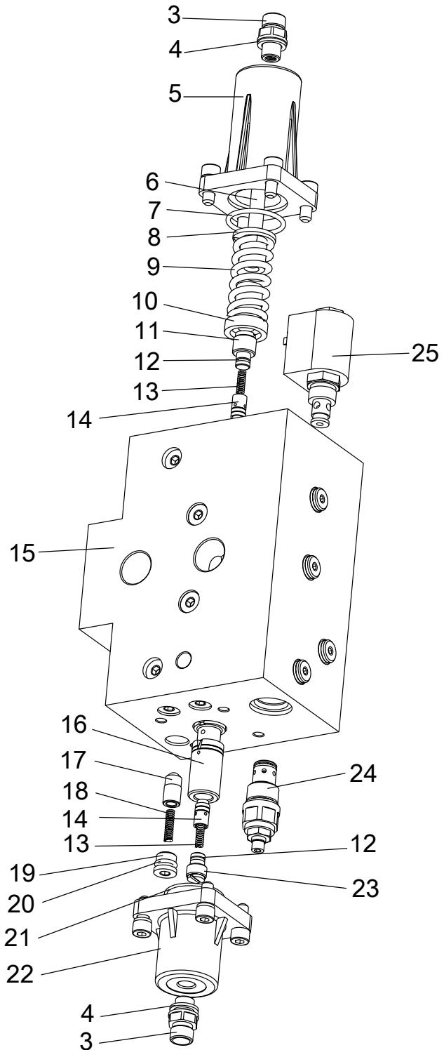
**SLEWING CUSHION VALVE(PILOT-OPERATED DIRECTIONAL CONTROL VALVE)**
