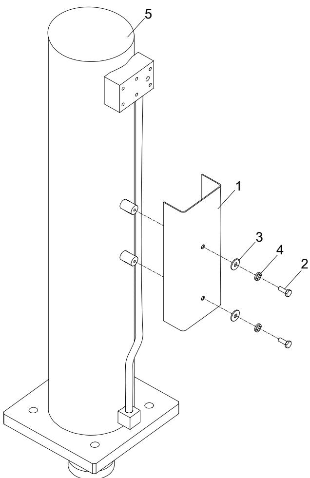
**OIL PIPE PROTECTION COVER INSTALLATION
