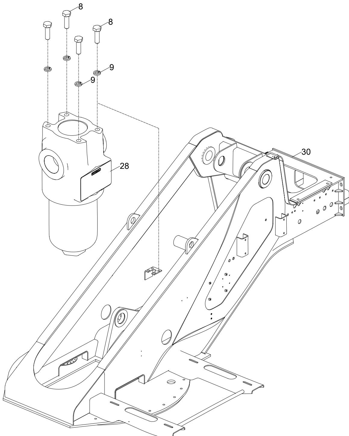
**SLEWING TABLE VALVE INSTALLATION(PIPE FILTER INSTALLATION)**
