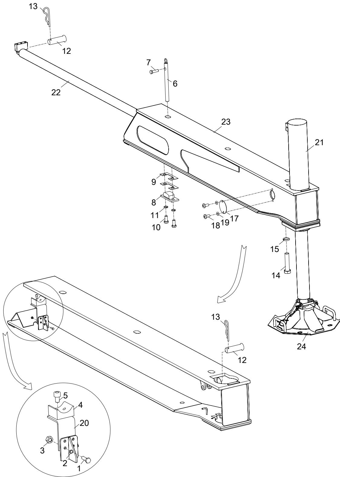
**OUTRIGGER AND ITS CYLINDER INSTALLATION
