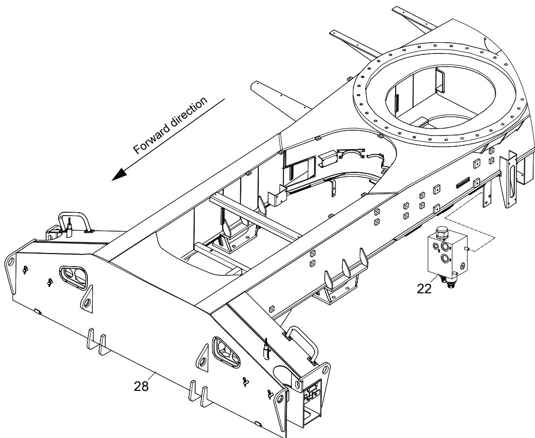
**CHASSIS FRAME VALVE INSTALLATION(RELIEF CONTROL VALVE BLOCK
