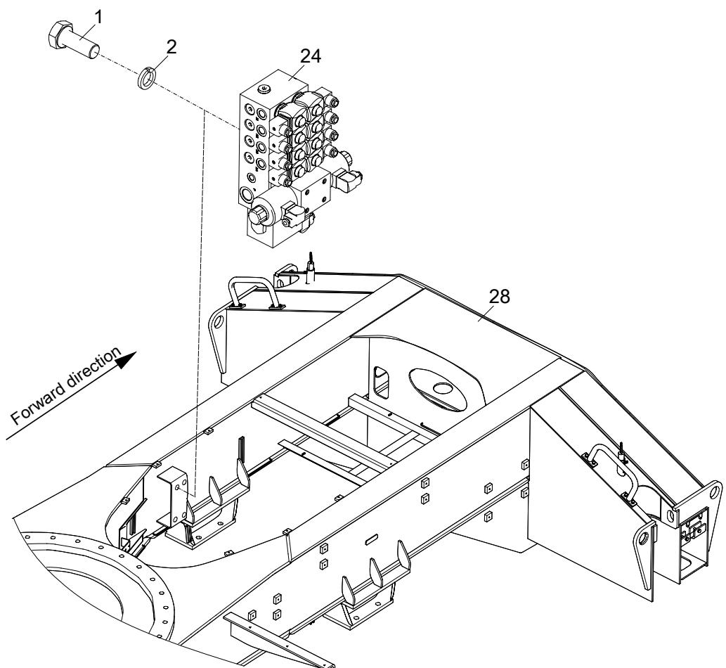
**CHASSIS FRAME VALVE INSTALLATION(OUTRIGGER CONTROL VALVE
