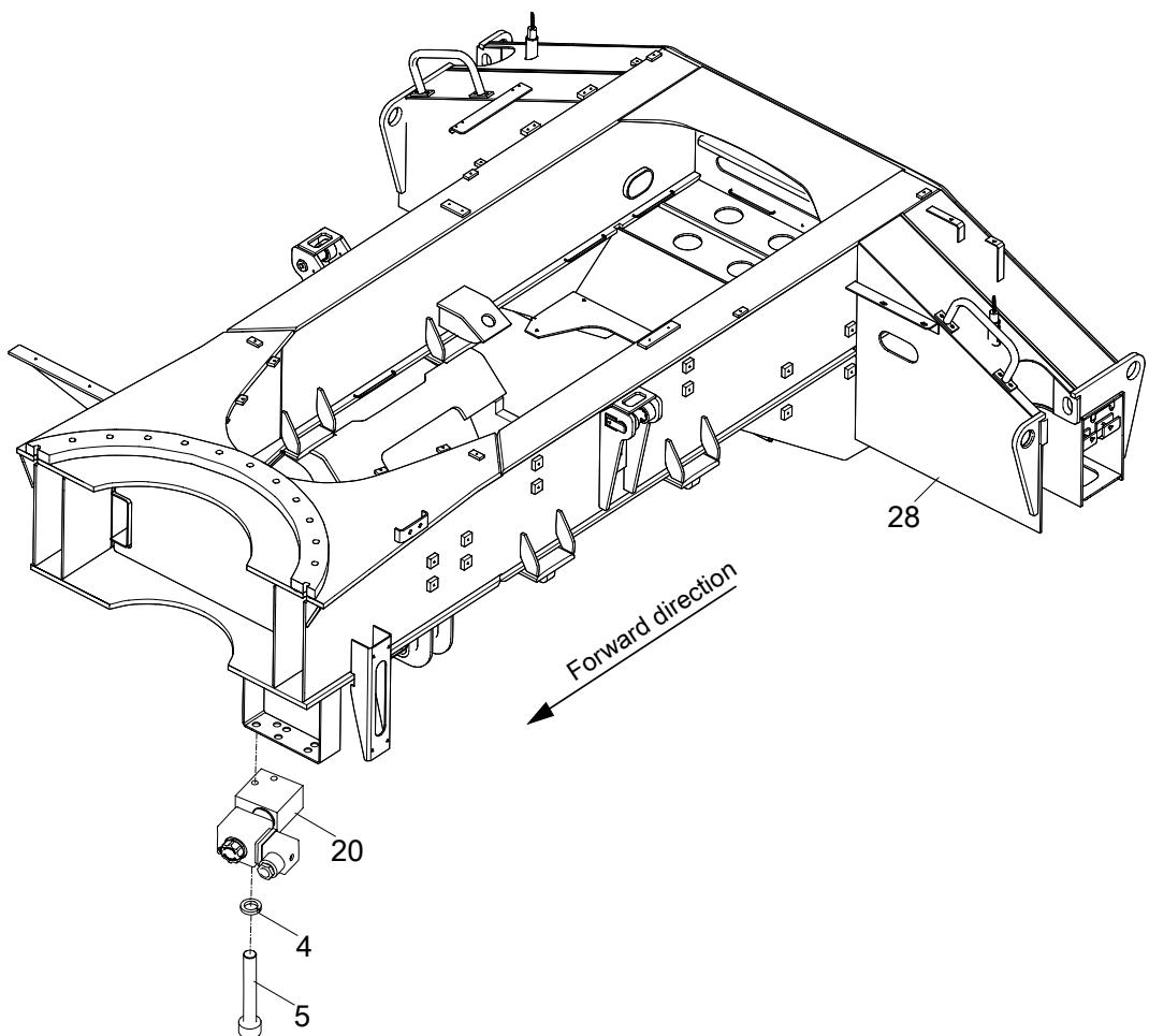
**CHASSIS FRAME VALVE INSTALLATION(LOCKING SOLENOID VALVE
