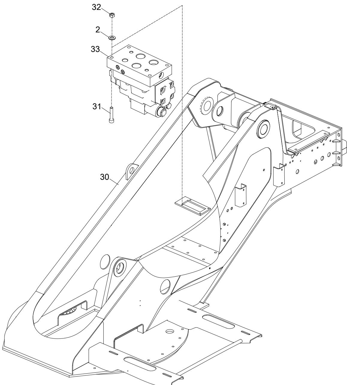
**SLEWING TABLE VALVE INSTALLATION(ELECTRO-HYDRAULIC)
