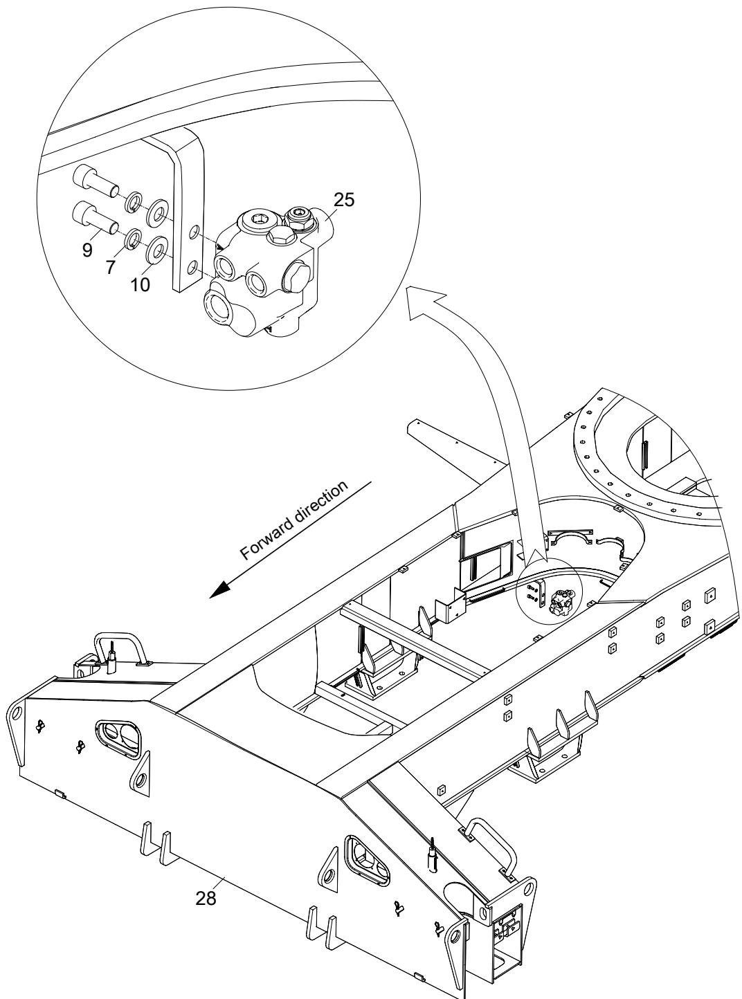
**CHASSIS FRAME VALVE INSTALLATION(FLUID FILLING VALVE INSTALLATION)
