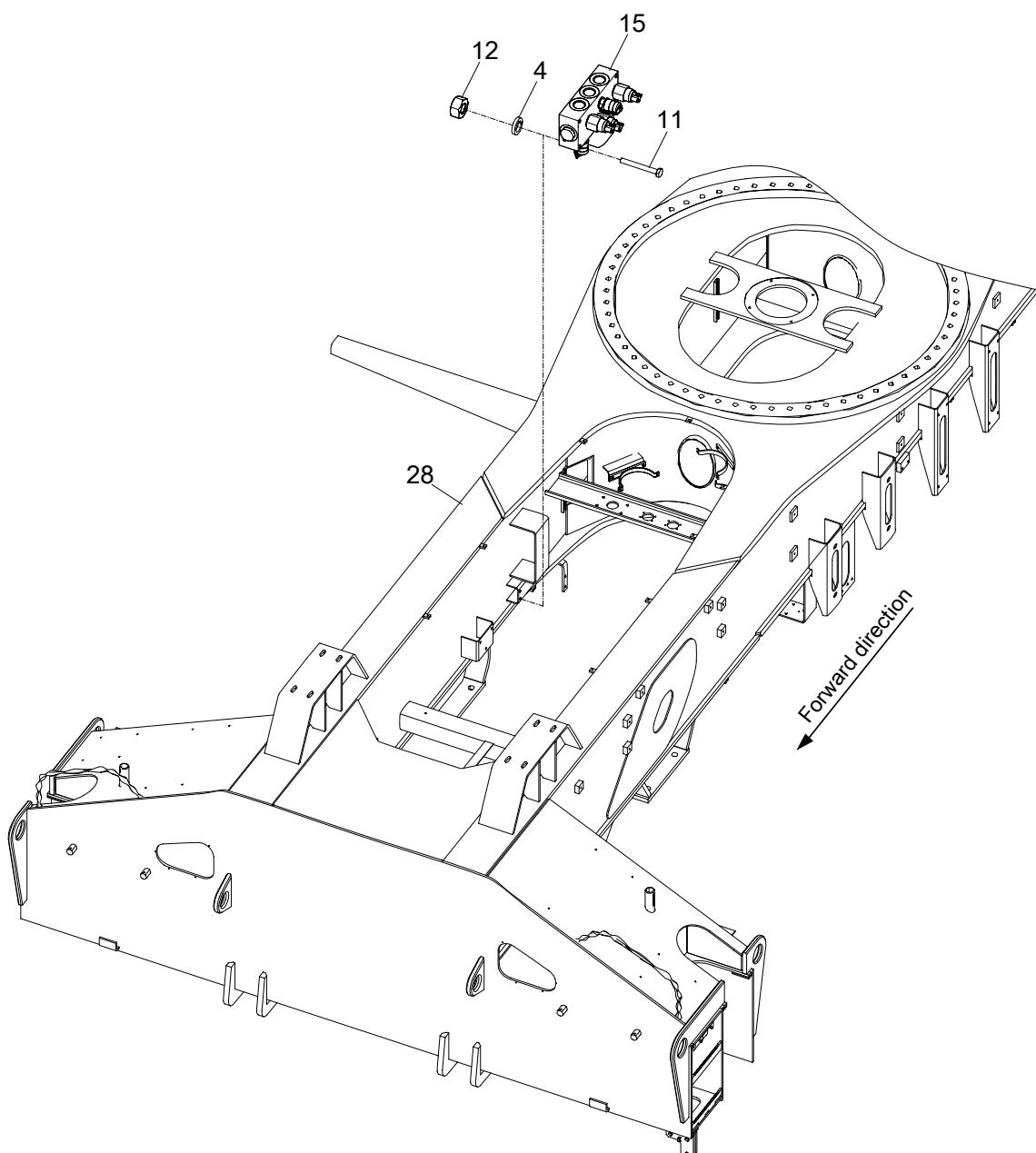
**CHASSIS FRAME VALVE INSTALLATION(BRAKE VALVE ASSY. INSTALLTION)
