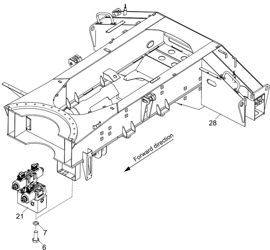
**CHASSIS FRAME VALVE INSTALLATION(STEERING CONTROL VALVE BLOCK
