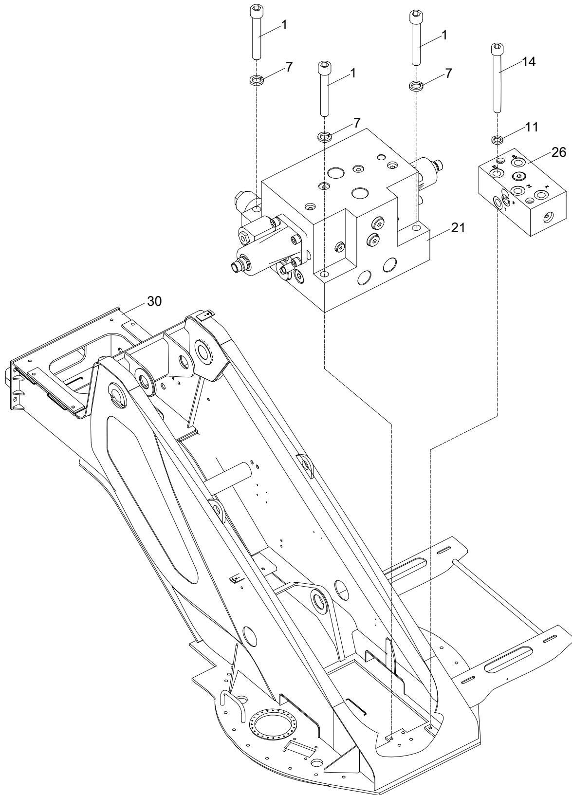
**SLEWING TABLE VALVE INSTALLATION(SLEWING CUSHION VALVE AND SLEWING BRAKE VALVE INSTALLATION)D00755914820800000Y**
