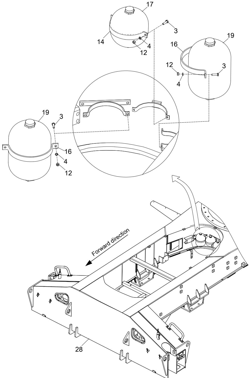
**CHASSIS FRAME VALVE INSTALLATION(ACCUMULATOR INSTALLATION)**
