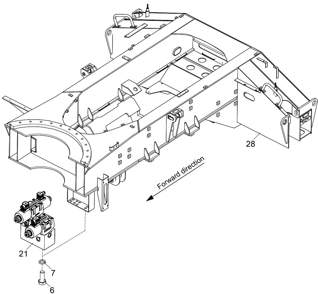
**CHASSIS FRAME VALVE INSTALLATION(STEERING CONTROL VALVE BLOCK
