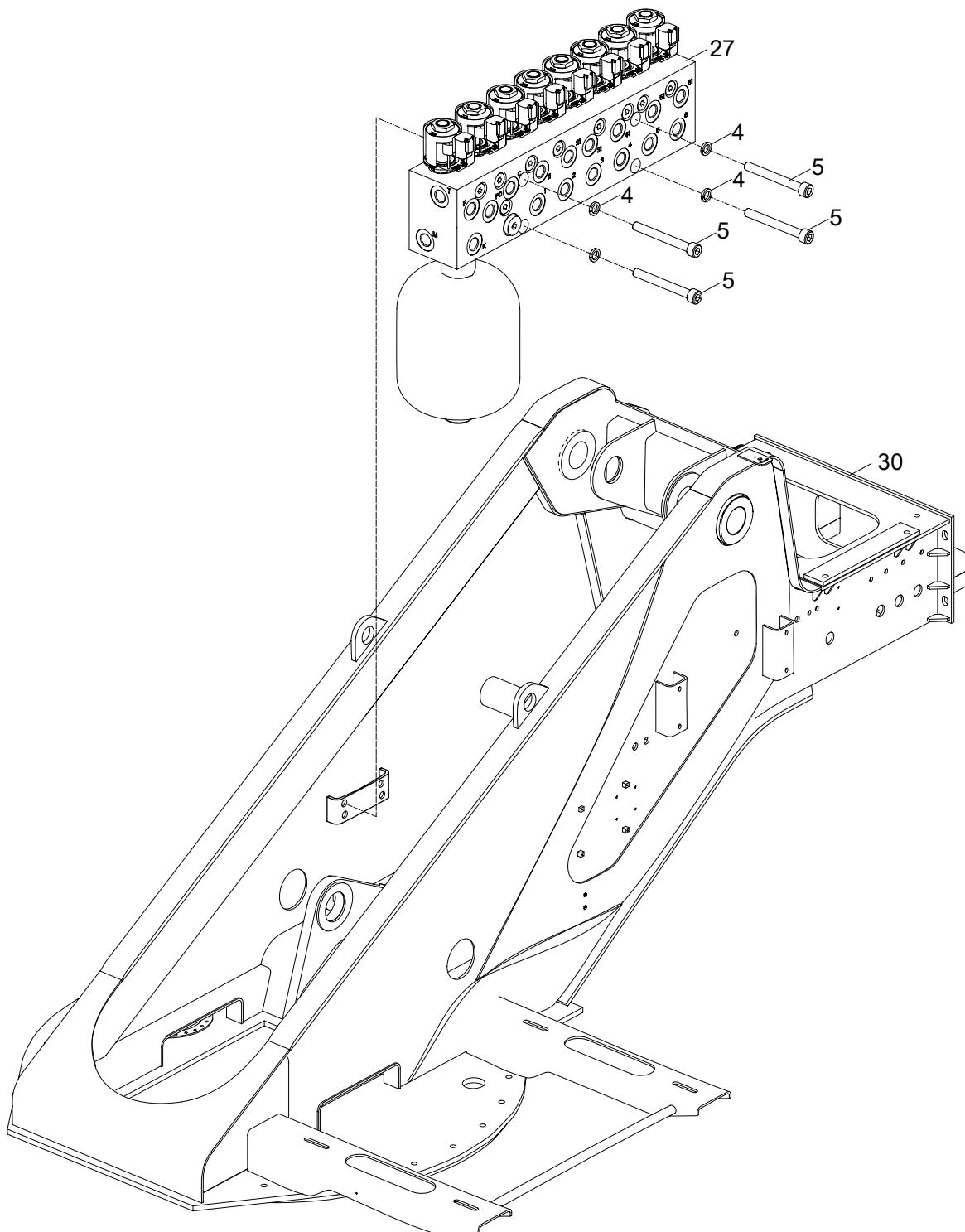
**SLEWING TABLE VALVE INSTALLATION(PILOT-OPERATED CONTROL VALVE BLOCK INSTALLATION) D00755914810600002Y**
