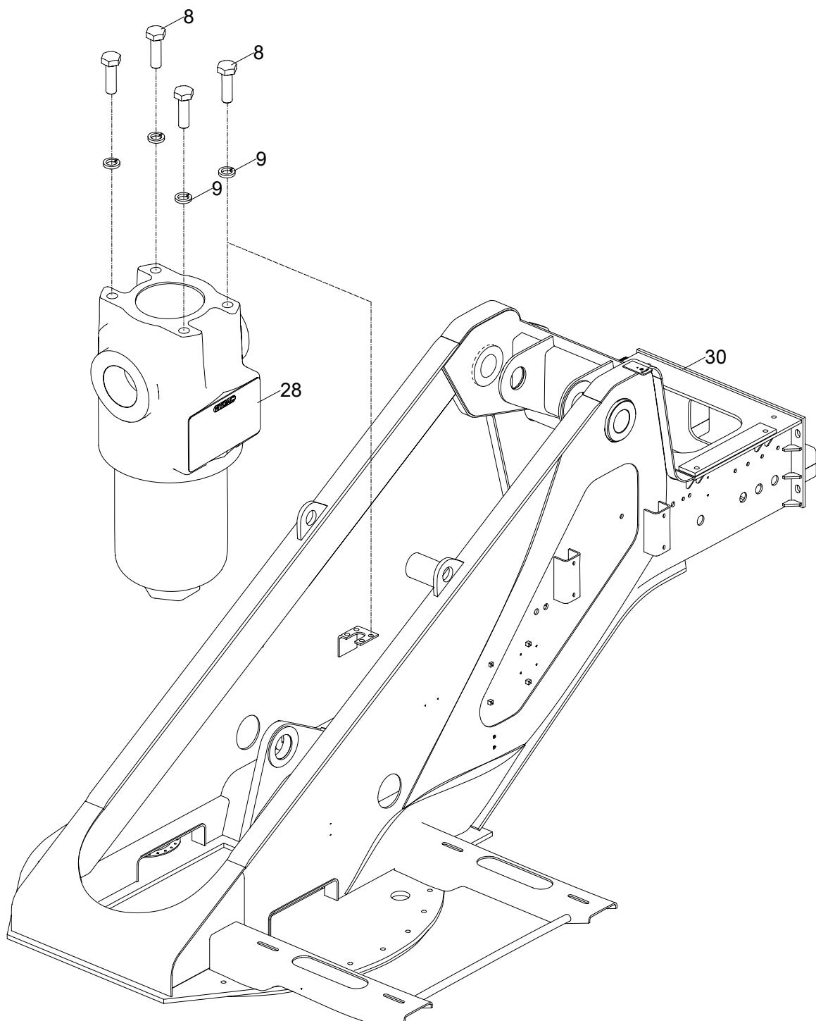
**SLEWING TABLE VALVE INSTALLATION(PIPE FILTER INSTALLATION)**
