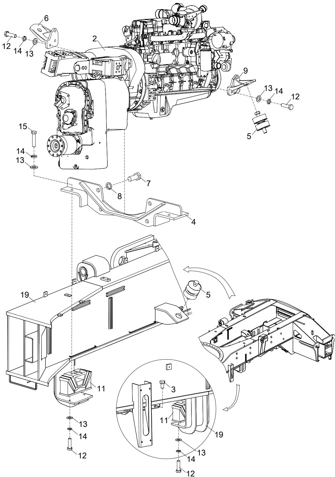
**TRANSMISSION AND ENGINE INSTALLATION
