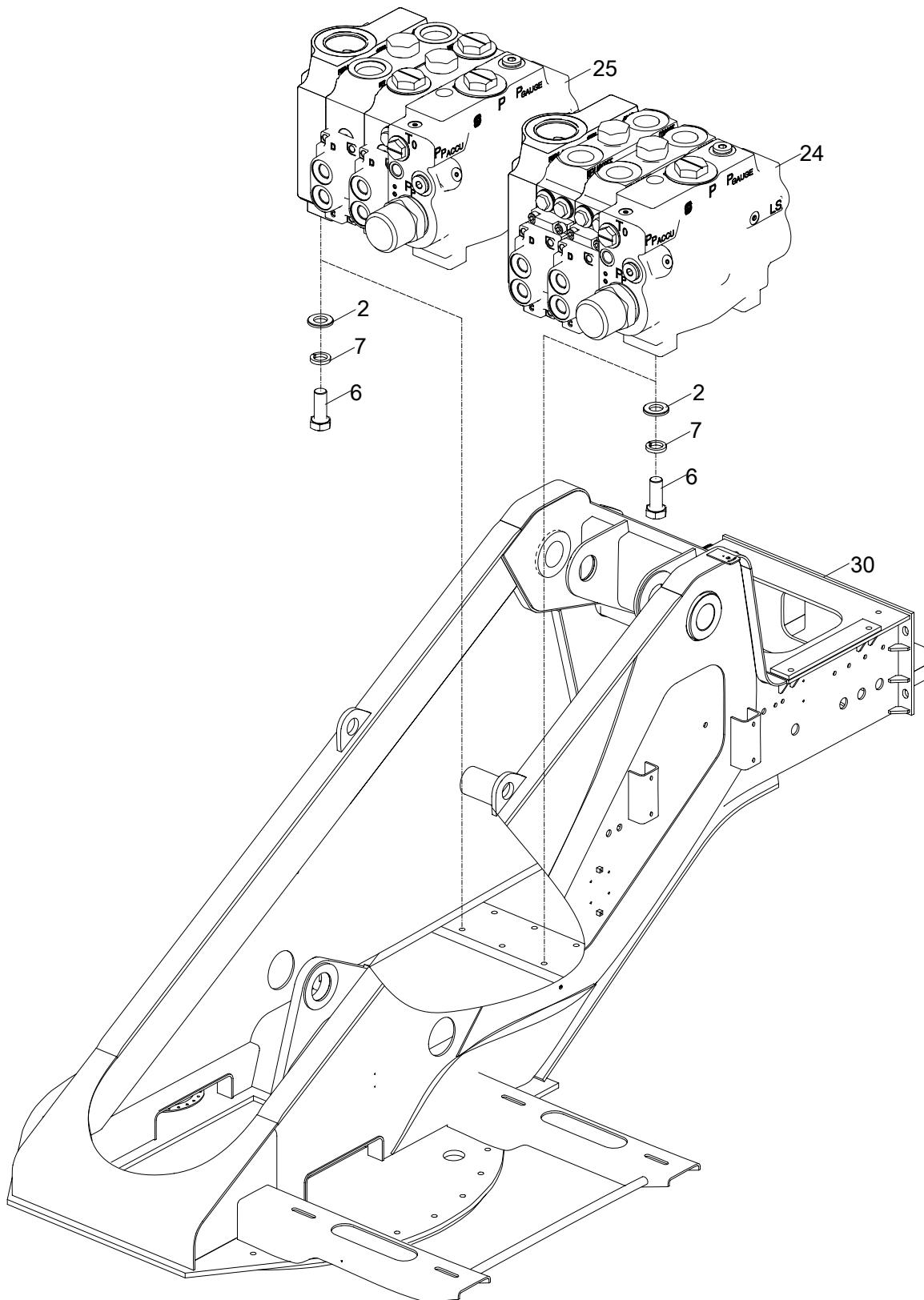
**SLEWING TABLE VALVE INSTALLATION(WINCH VALVE INSTALLATION AND
