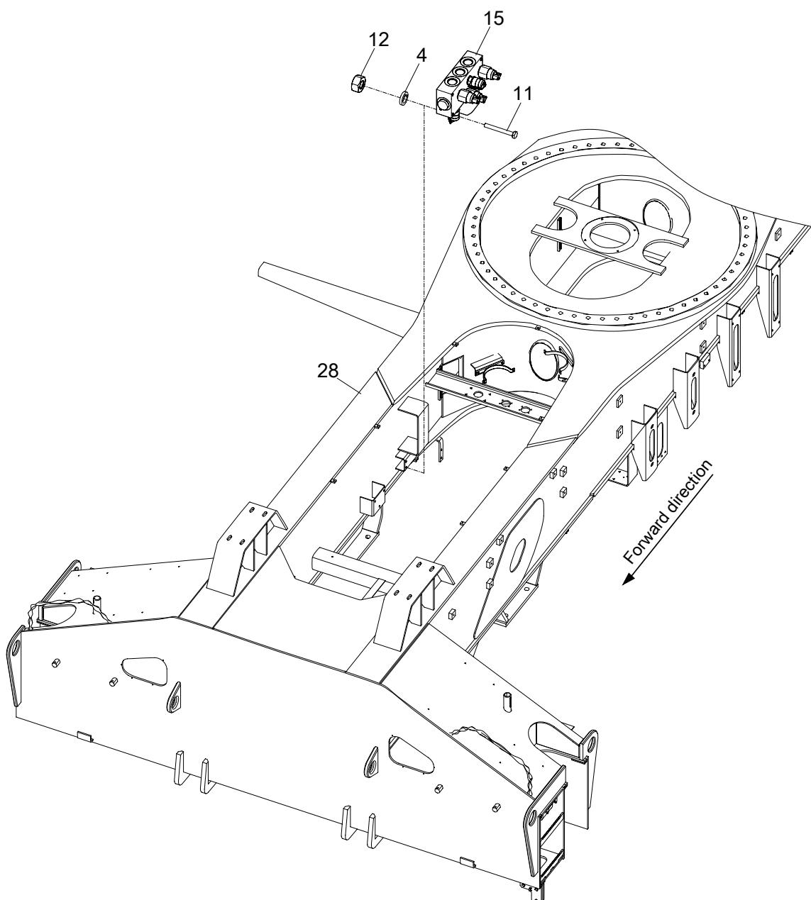
**CHASSIS FRAME VALVE INSTALLATION(BRAKE VALVE ASSY. INSTALLTION)
