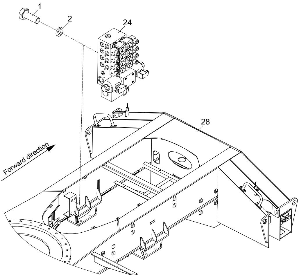
**CHASSIS FRAME VALVE INSTALLATION(OUTRIGGER CONTROL VALVE
