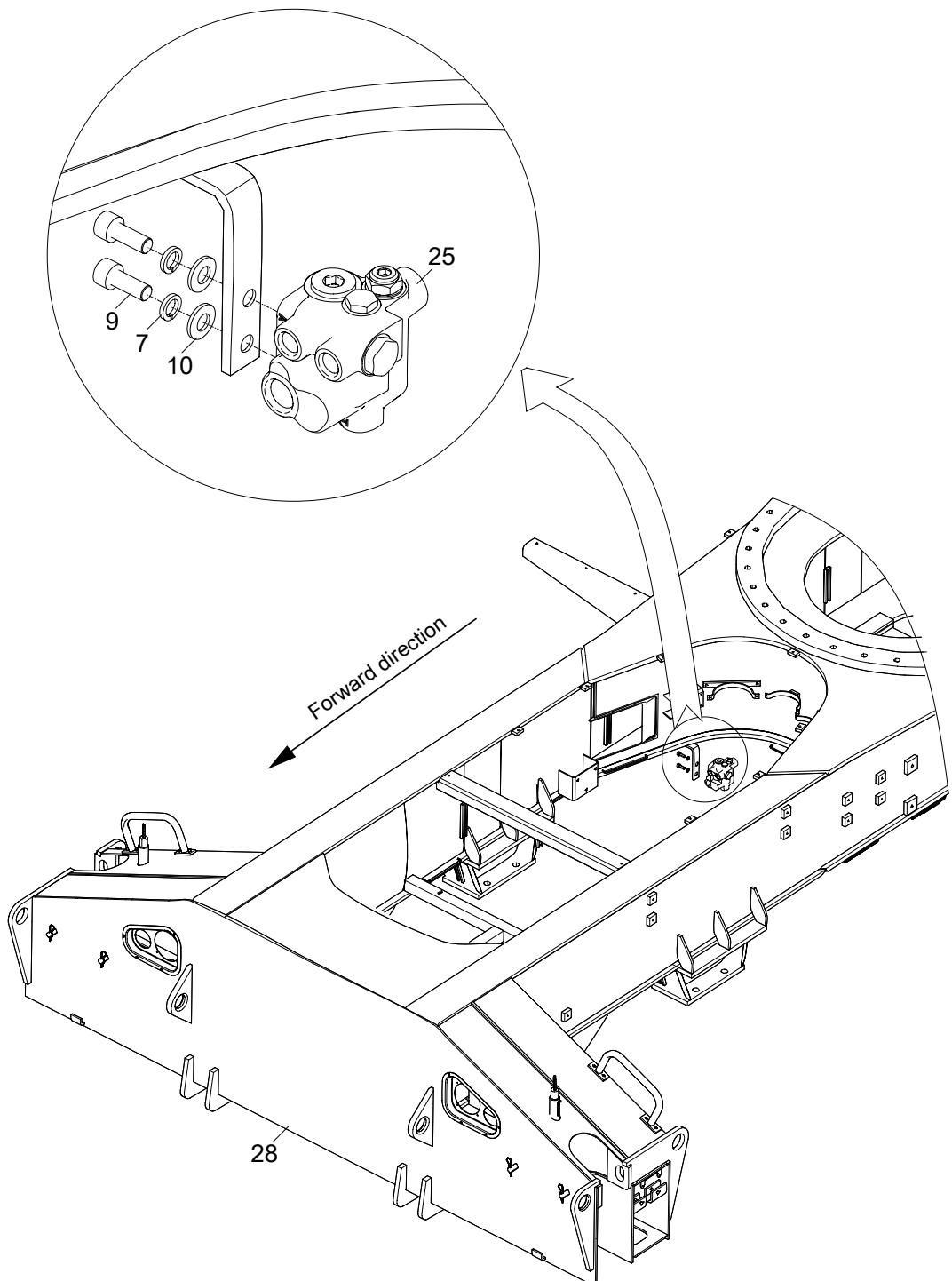
**CHASSIS FRAME VALVE INSTALLATION(FLUID FILLING VALVE INSTALLATION)
