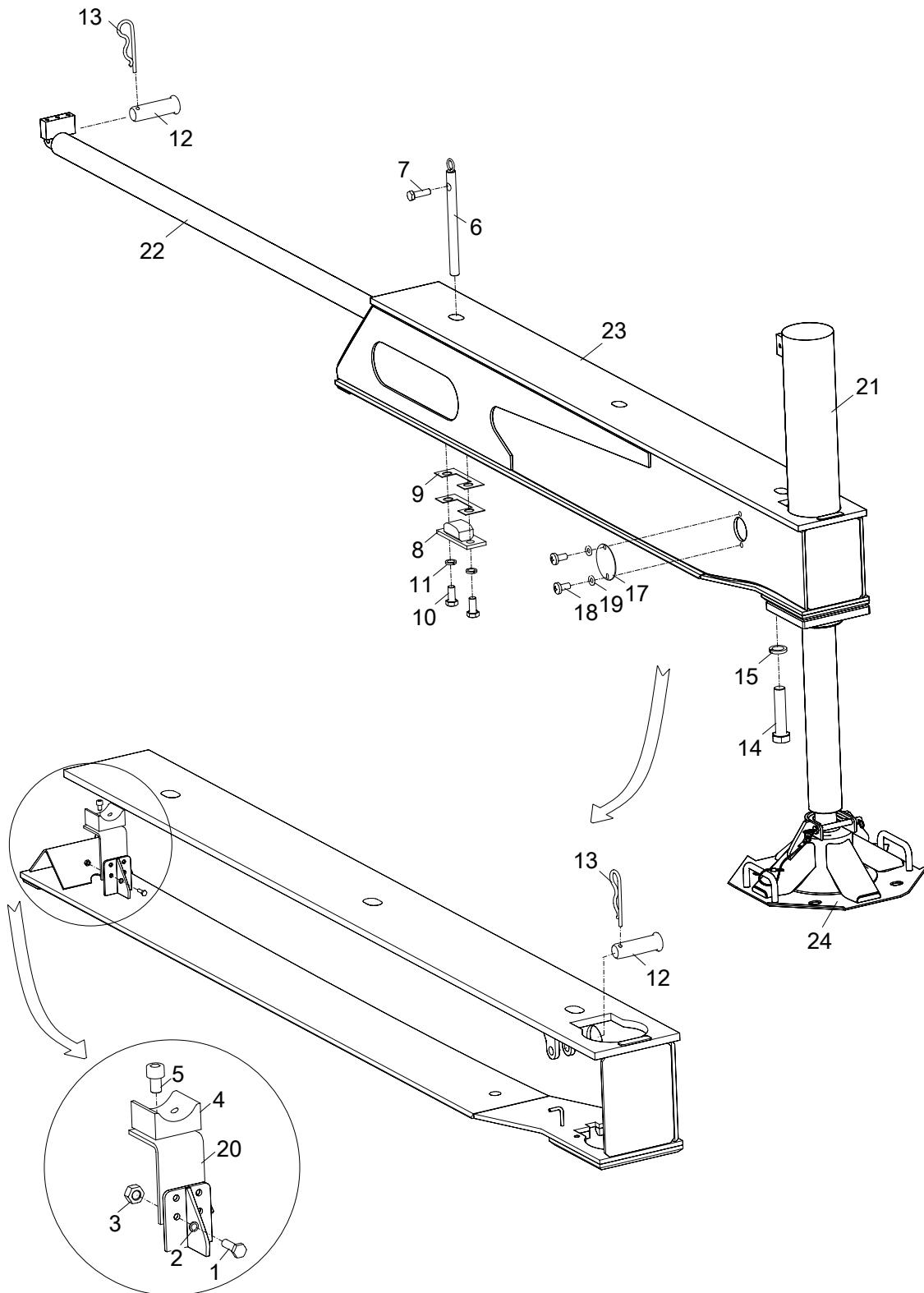
**OUTRIGGER AND ITS CYLINDER INSTALLATION
