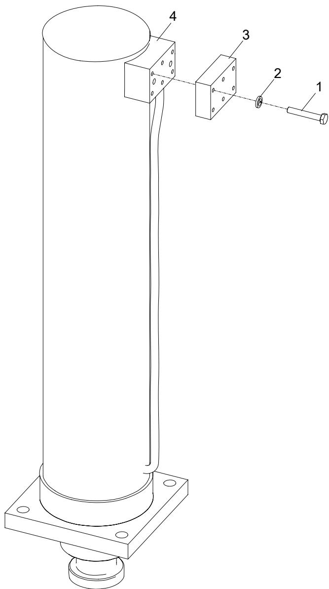
**OUTRIGGER HYDRAULIC LOCK INSTALLATION
