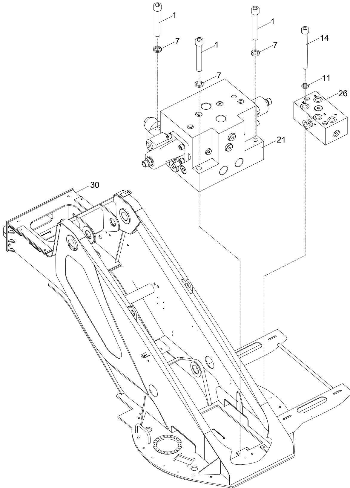
**SLEWING TABLE VALVE INSTALLATION(SLEWING CUSHION VALVE AND SLEWING BRAKE VALVE INSTALLATION)D00755914810600002Y**
