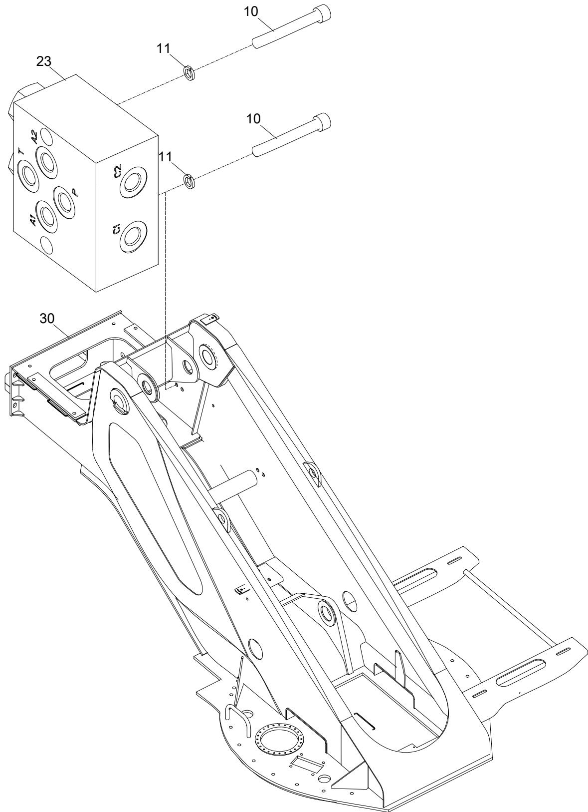
**SLEWING TABLE VALVE INSTALLATION(PILOT-OPERATED VALVE INSTALLATION)
