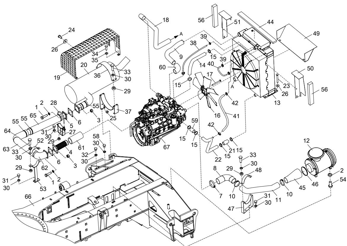
**ENGINE ATTACHMENTS INSTALLATION**
