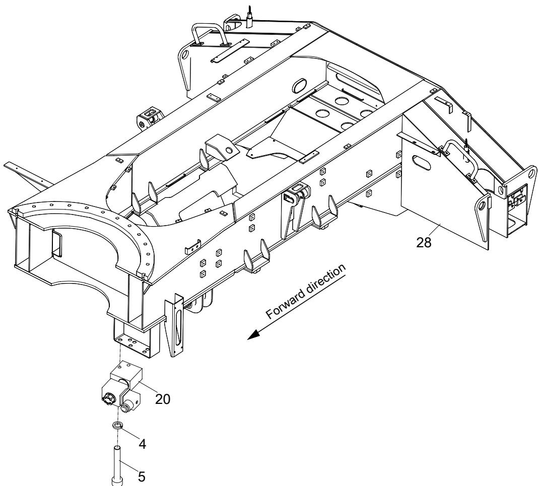
**CHASSIS FRAME VALVE INSTALLATION(LOCKING SOLENOID VALVE
