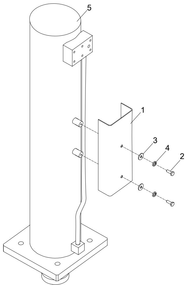
**OIL PIPE PROTECTION COVER INSTALLATION
