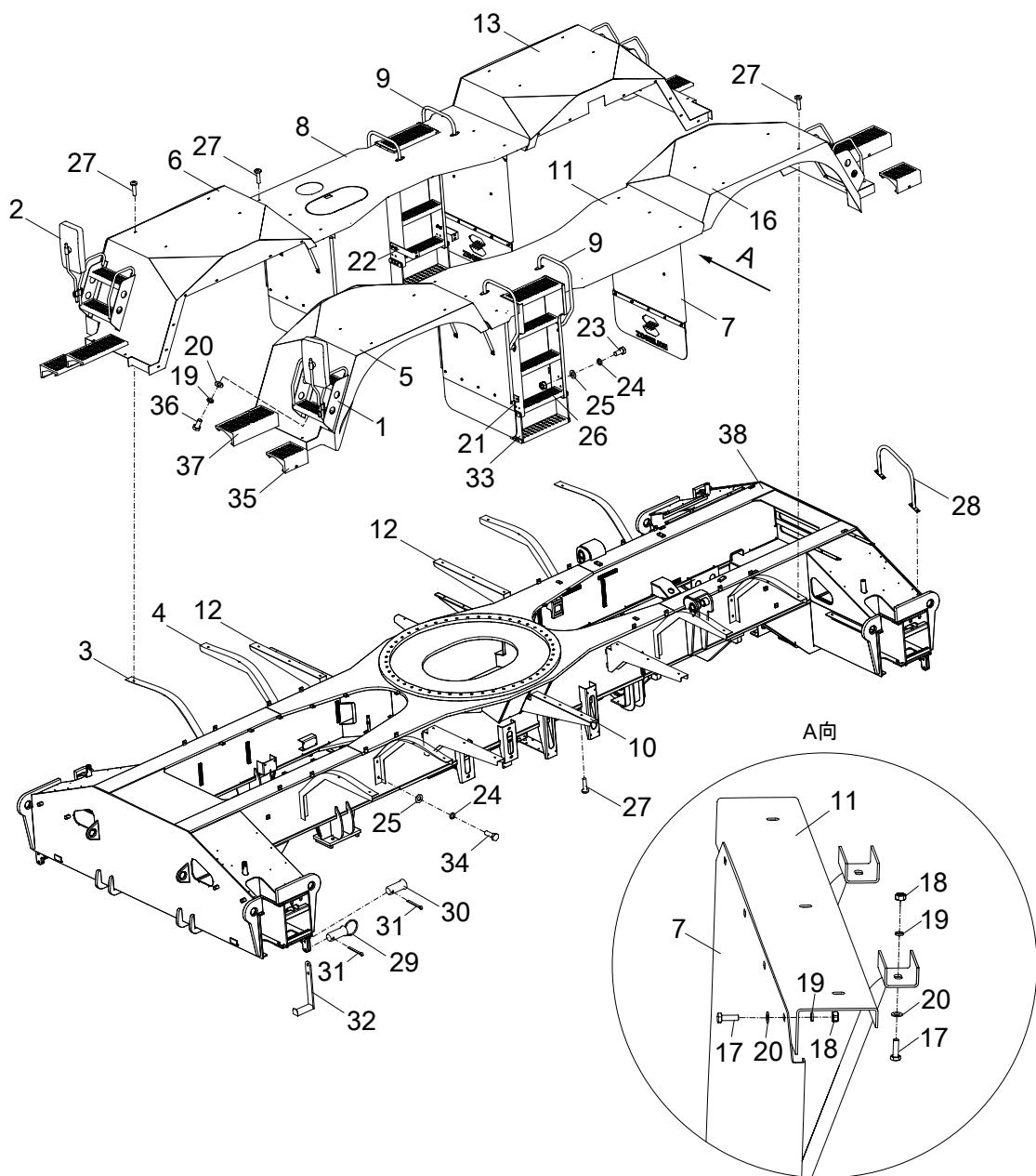
**WHEEL HOUSING AND ITS INSTALLATION
