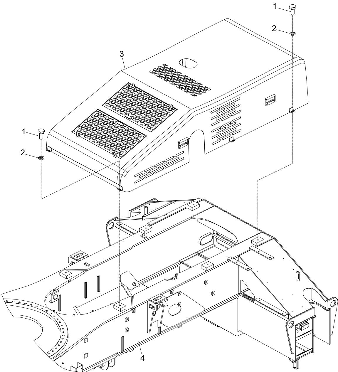
**ENGINE HOUSING AND ITS INSTALLATION
