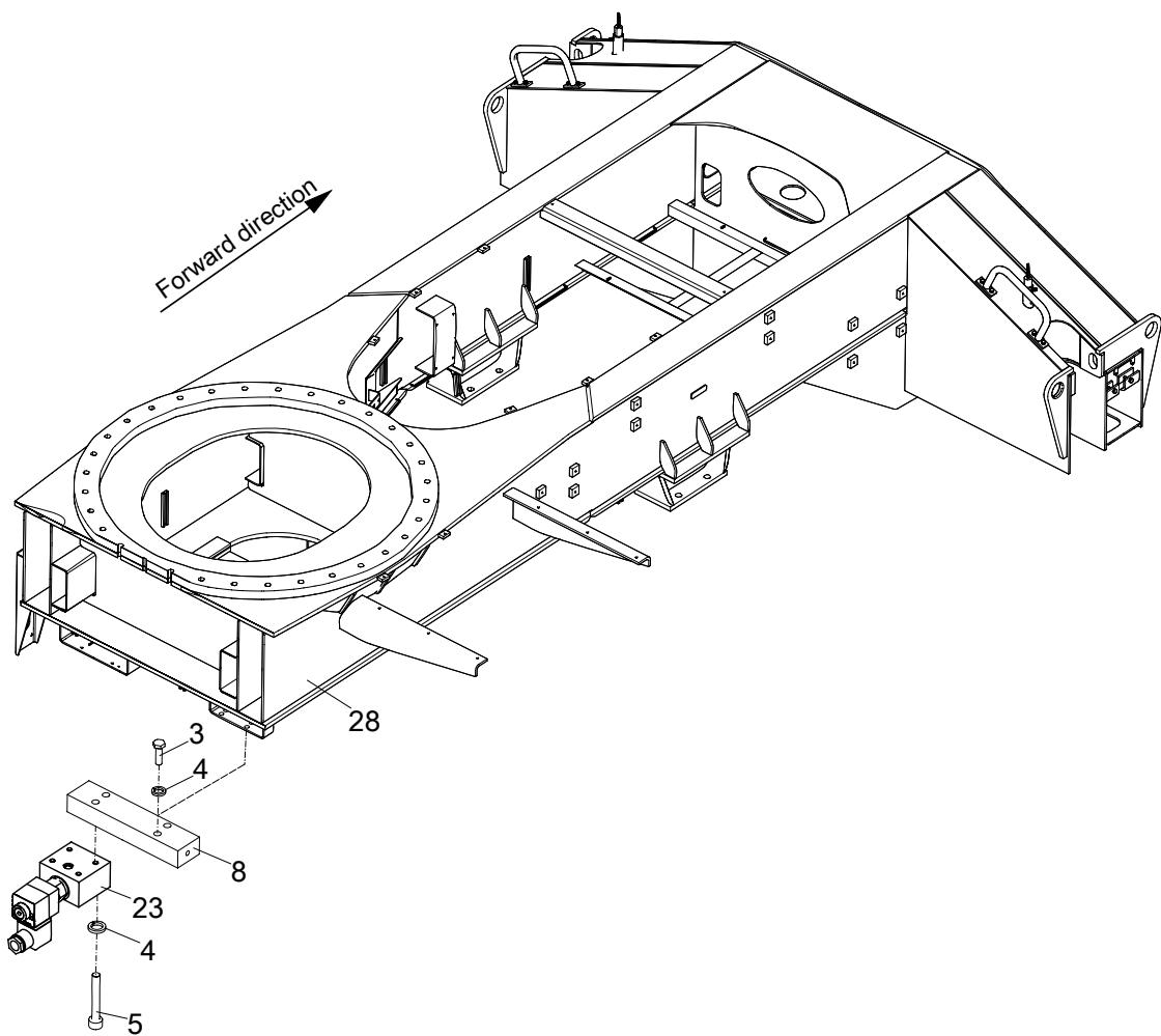
**CHASSIS FRAME VALVE INSTALLATION(SOLENOID VALVE INSTALLATION)
