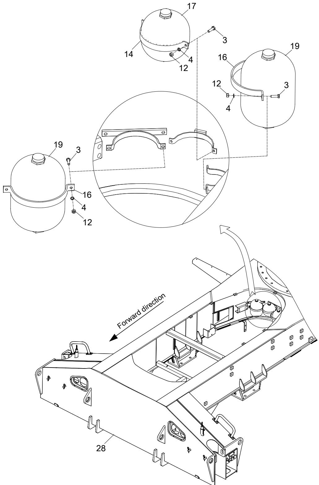
**CHASSIS FRAME VALVE INSTALLATION(ACCUMULATOR INSTALLATION)**
