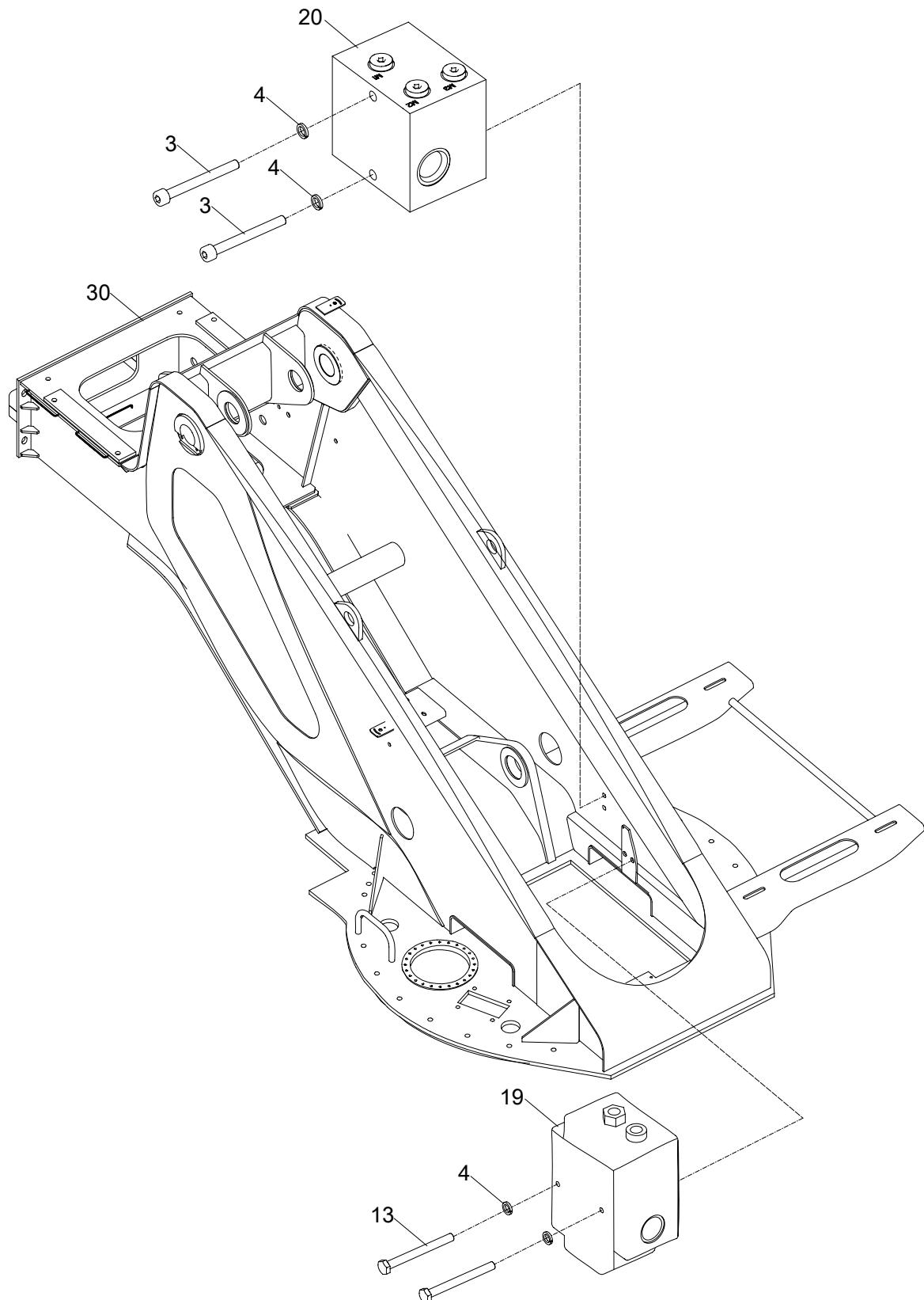
**SLEWING TABLE VALVE INSTALLATION(PRIORITY VALVE AND PILOT OIL SOURCE BLOCK INSTALLATION)D00755914810600002Y**
