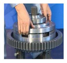
5. Take down the direct gear and three fiction plates together.
