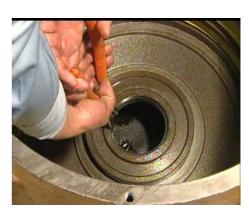
28. Loose the connection screws that fixed the shift pump.
