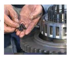
7. Take down the isolating ring and rubber band by hand.
