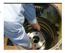
26. Take out the reverse gear piston, internal and external seal ring.
