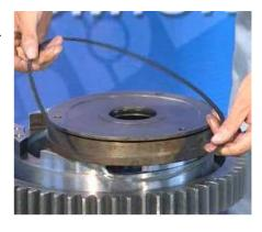
10. Take down the intermediate output gear by hand, separate the direct gear cylinder from the intermediate output gear, then take down the intermediate output gear.
