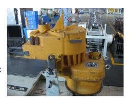
10. Disassemble the hand-brake assembly.
