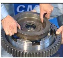
9. Take down the seal ring and rotary oil seal on the direct gear piston by hand.
