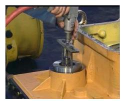
8. Take down the shield ring by axis-shield ring pliers.
