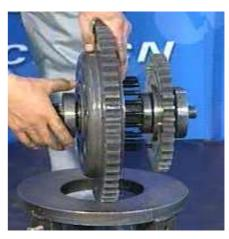
5. Bind the bolts with rubber band, and then take out the isolating ring, inner loop cam and 24 balls and bolts simultaneously.
