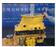
When hang the torque converter, make sure that hanging tools on the right top of it. For avoiding hurting hands, do not touch the joint surface of torque converter which is hanged away transmission in the progress of hanging.
