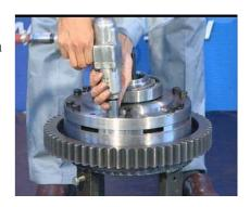
4. Take down the direct gear pressure plate by hand.
