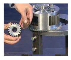
9. Take out the shield ring and needle roller in the planet gear.
