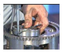
Make sure the circlip plier is clamped firmly during using to avoid bouncing off the box body and forming hidden danger.
