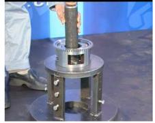
11. Take out the shield ring on the bearing with external circlip pliers.
