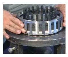
8. Take out the shield ring with circlip pliers.
