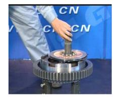
6. Take down the shield ring with external circlip pliers.
