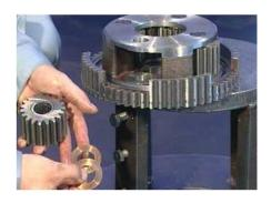
5. Take down the shield ring and needle roller in the planet gear by hand.
