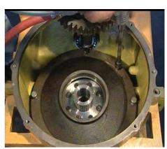
17. Disassemble First gear oil cylinder by hand. Take out the piston, the internal and external seal ring.
