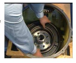
18. Take out the return spring and spring guide pin by hand.
