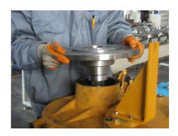
12. Disassemble the oil seal assembly with professional tools.
