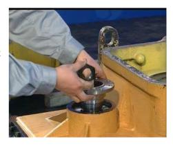
7. Disassemble the oil seal assembly with professional tools.
