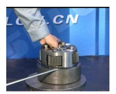
6. Separate the inner ring gear from planet gear frame, and take down the inner ring gear.
