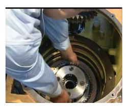
25. Take out the reverse gear planetary carrier assembly by hand.
