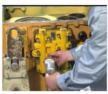
Loose the bolts by corresponding specification tools.Take down the stop-pushing gasket and back export flange.
