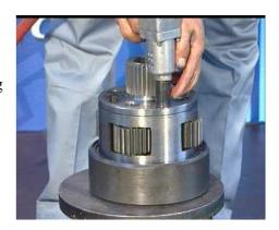
3. Take down the direct gear coupling flange by hand.
