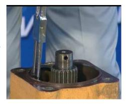
14. Loose the end cover bolts with corresponding specification tools and push end cover away from box with two pusher screws. Top screw: M10.
