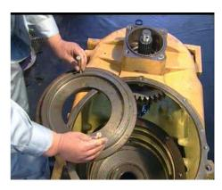
27. Detach the spring seal ring on the box four-axis with circlip pliers.
