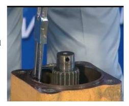
Turn the big end surface of transmission box to downward and put the transmission assembly fixed on the carrier.
