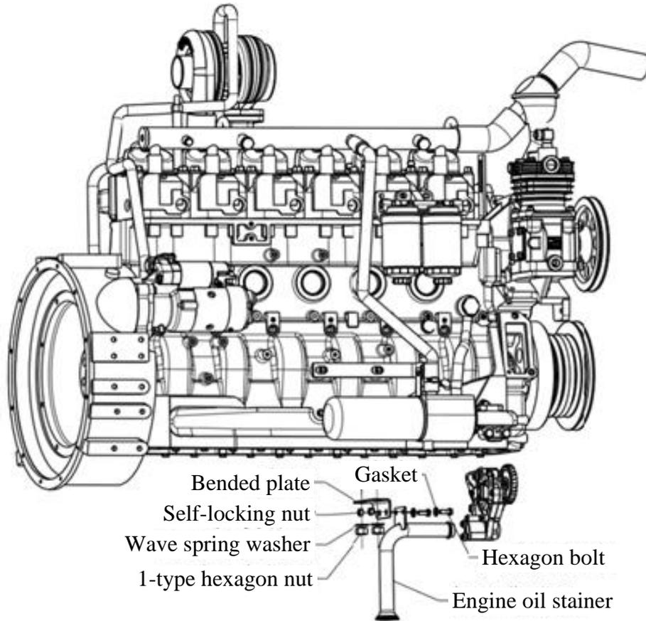
Fig. 3-57 Exploded view of engine oil strainer
