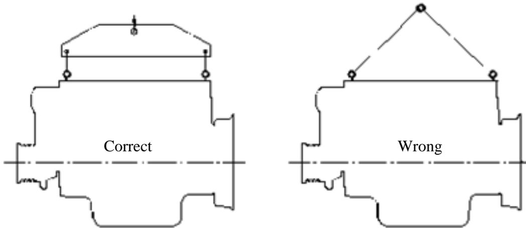
Fig. 1-5 Lifting of diesel engine
