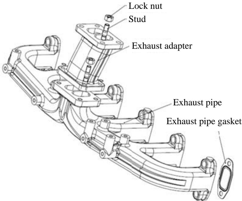
Fig. 3-41 Exploded view of exhaust pipe
