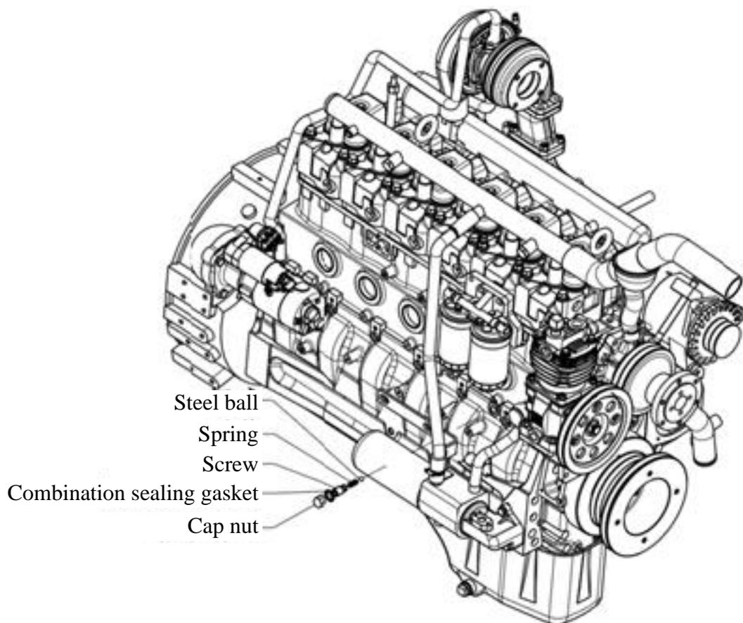
Fig. 3-56 Exploded view of main oil gallery pressure limiting valve
