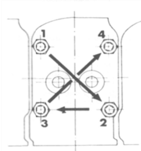
Fig. 3-11 Cylinder cover bolts tightening order
