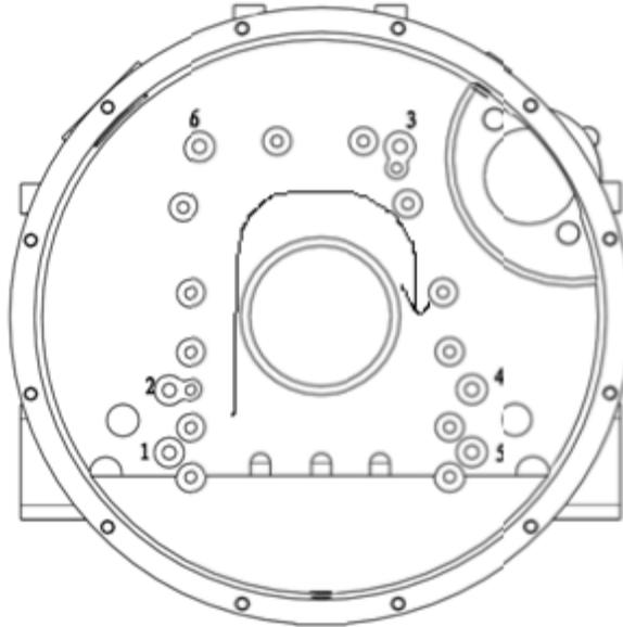
Fig. 3-20 Tightening order of flywheel housing bolts
