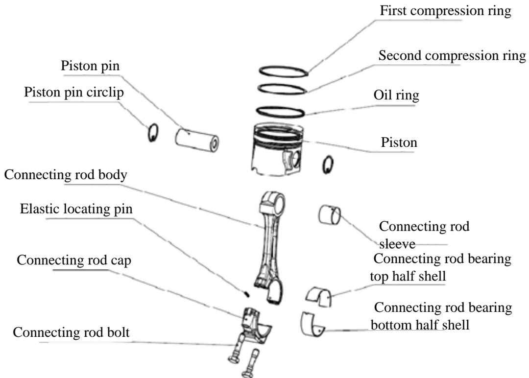
Fig. 3-27 Exploded view of piston-rod assembly
