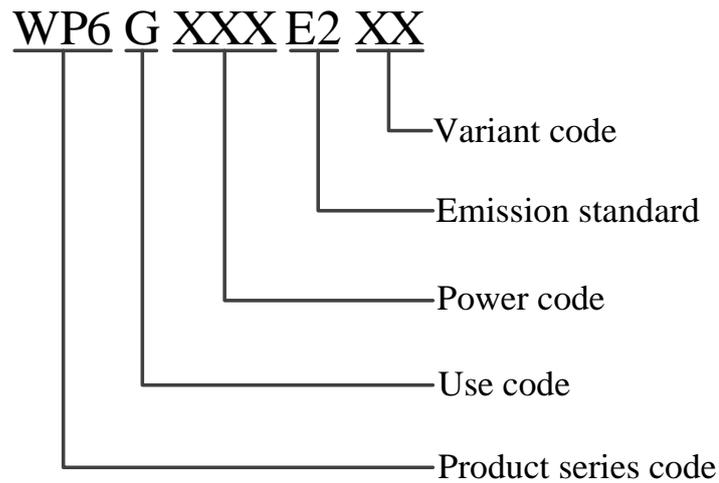
Fig. 1-4 Diesel Engine Model Composition and Significance
