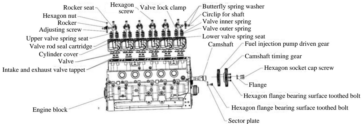
Fig. 3-34 Exploded view of valve mechanism
