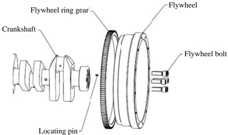
Fig. 3-31 Exploded view of flywheel and ring gear
