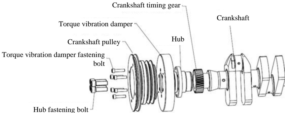
Fig. 3-32 Exploded view of torque vibration damper, crankshaft pulley and hub
