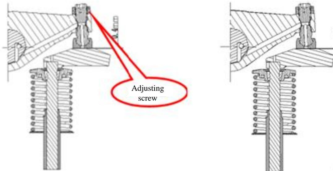
Fig. 2-13 Adjusting screw
