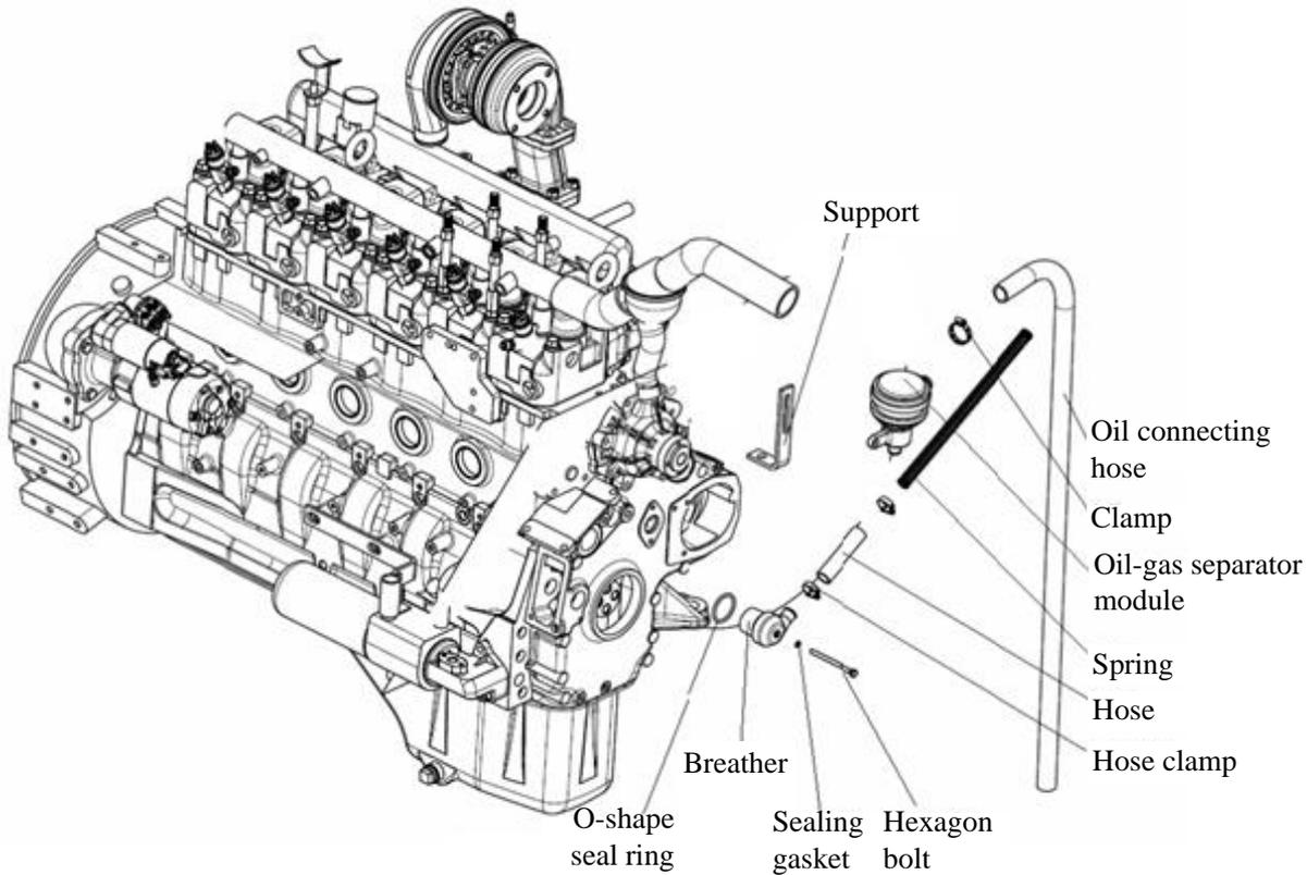
Fig. 3-8 Exploded view of oil-gas separator
