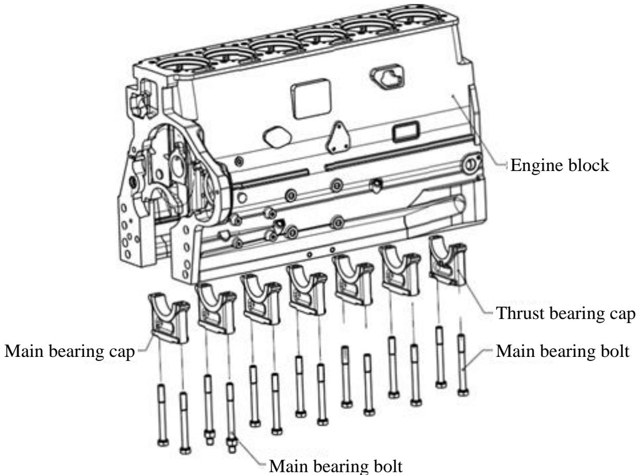
Fig. 3-12 Exploded view of engine block module
