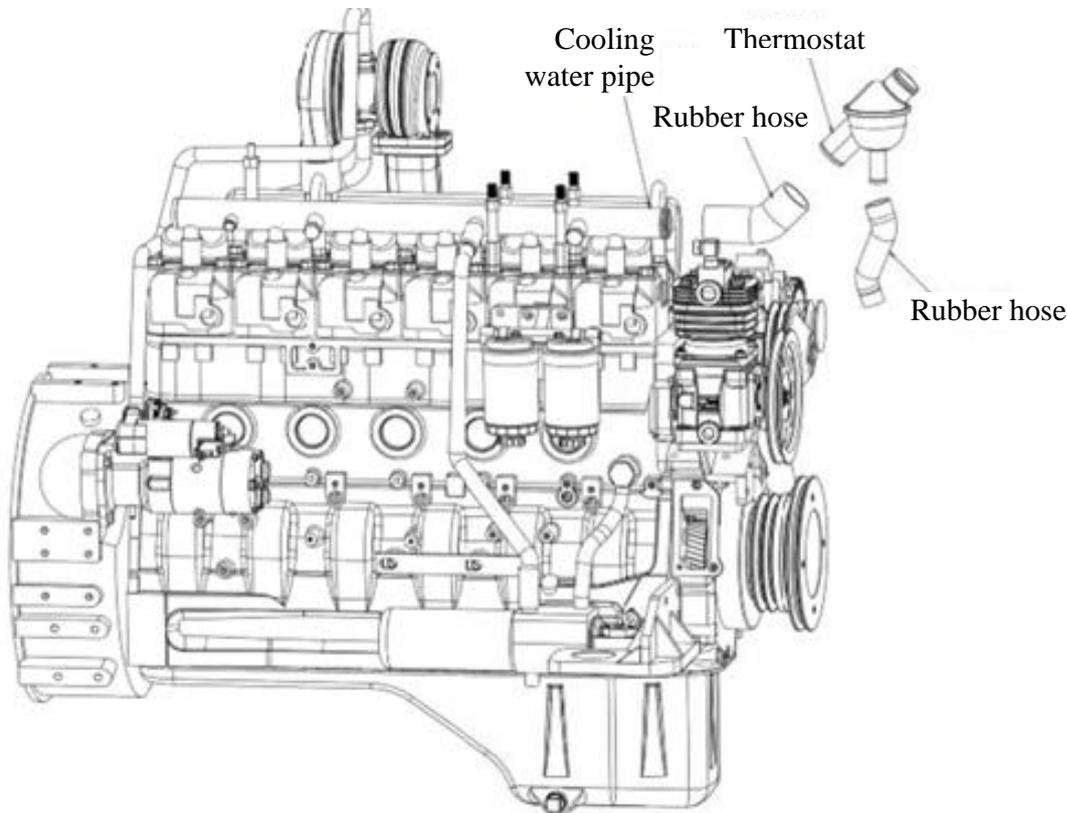
Fig. 3-51 Exploded view of thermostat
