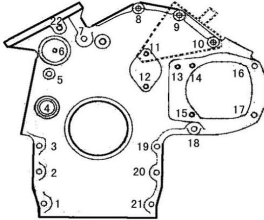
Fig. 3-18 Bolt tightening
