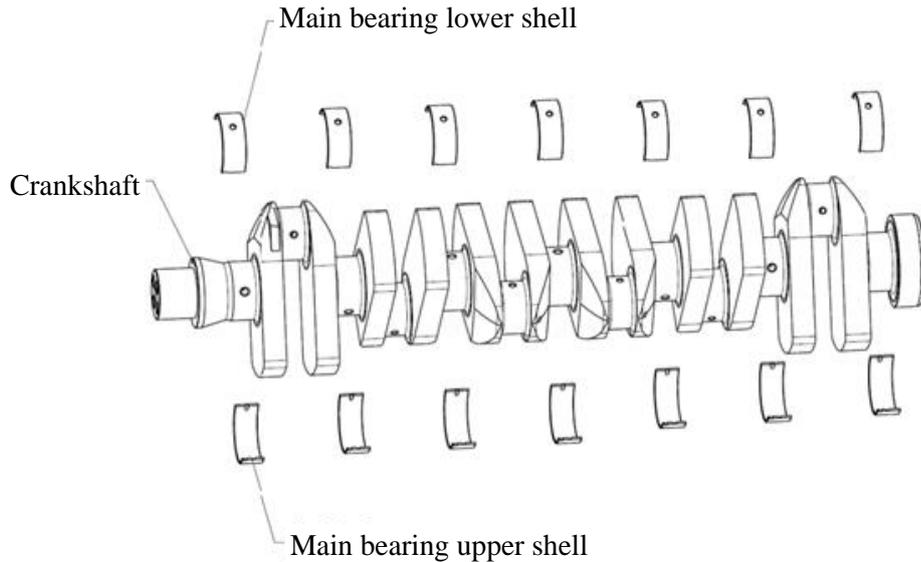
Fig. 3-33 Exploded view of crankshaft bearing shell
