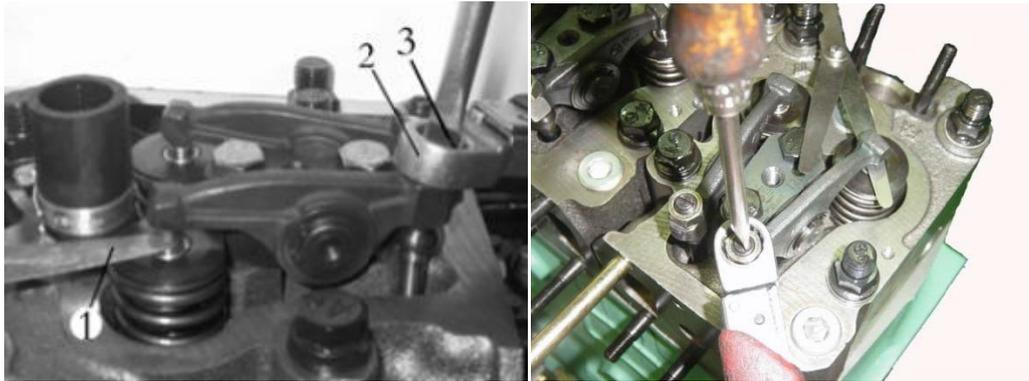
Fig. 2-12 Adjust valve clearance
