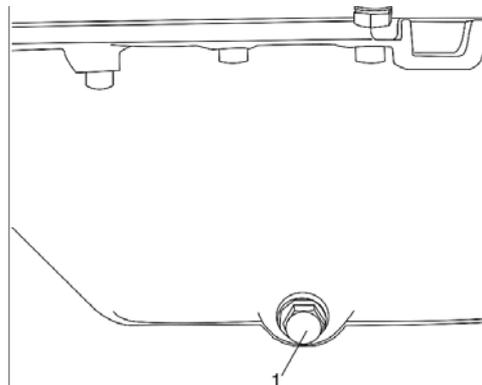
Fig. 2-9 Oil drain plug
