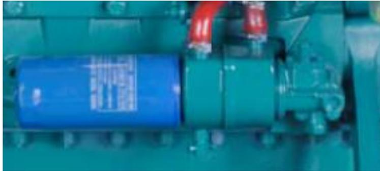
Fig. 2-10 Engine oil filter
