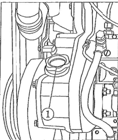
Fig. 2-8 Engine oil filling port
