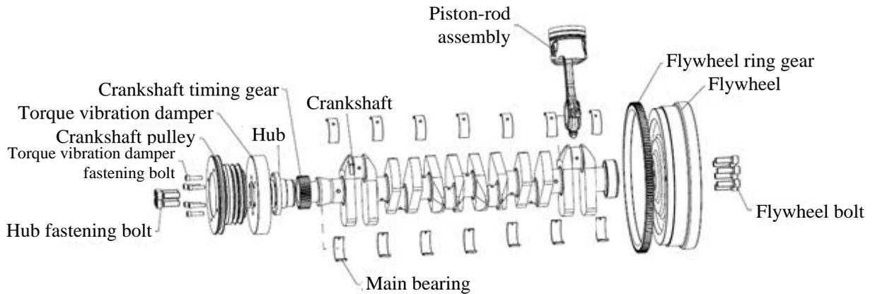
Fig. 3-25 Exploded view of crank-rod mechanism
