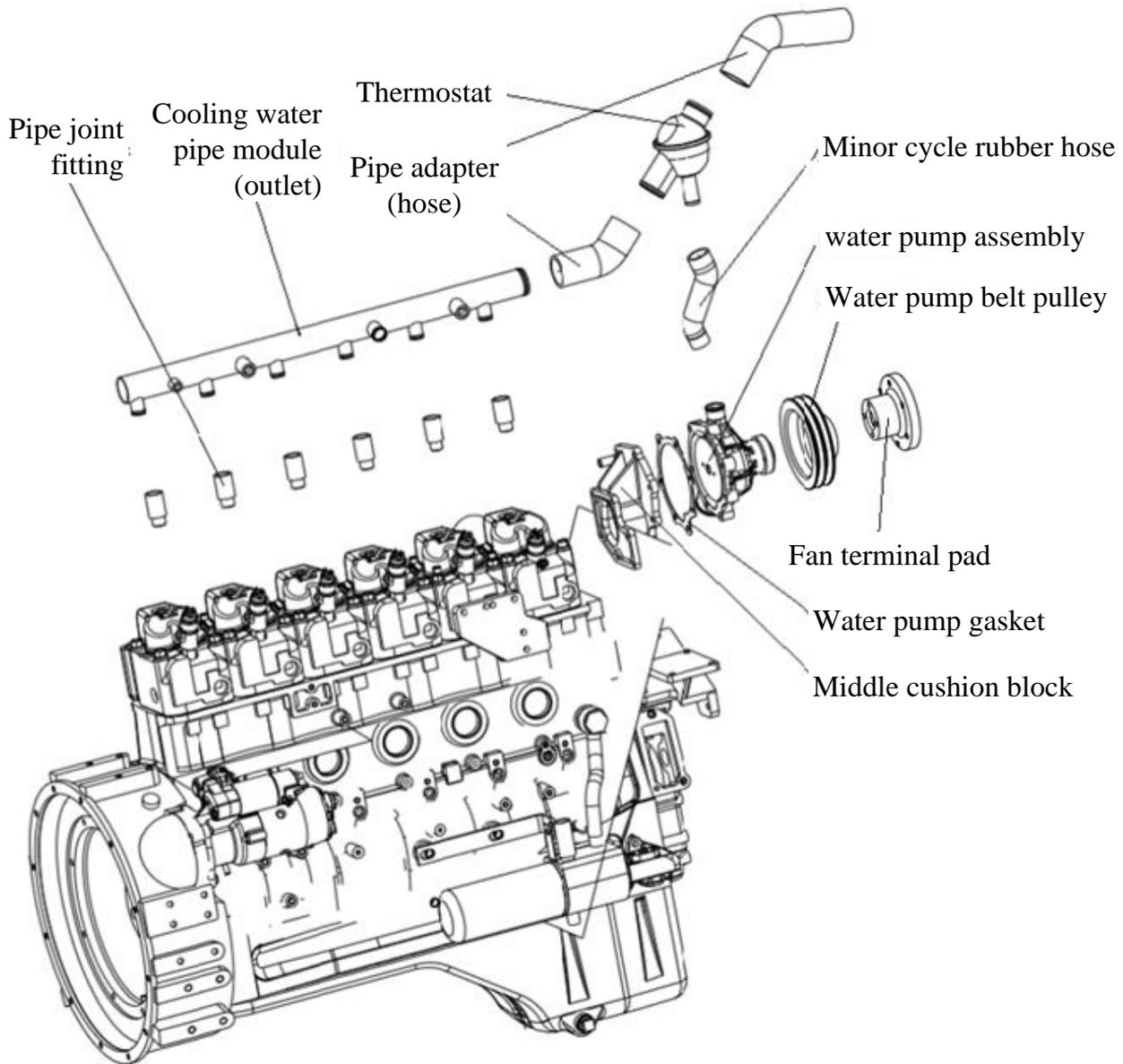
Fig. 3-7 Exploded view of water outlet pipe
