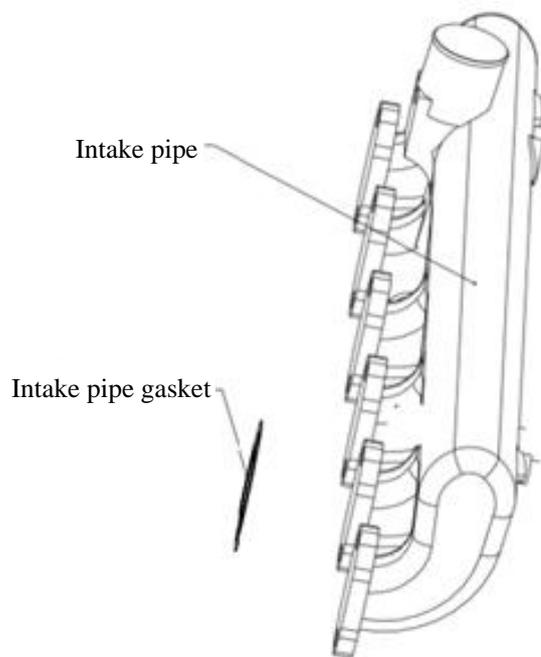
Fig. 3-40 Exploded view of intake pipe
