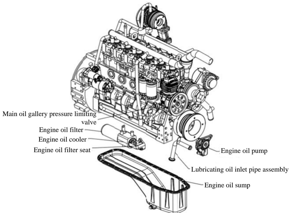
Fig. 3-52 Exploded view of lubricating system
