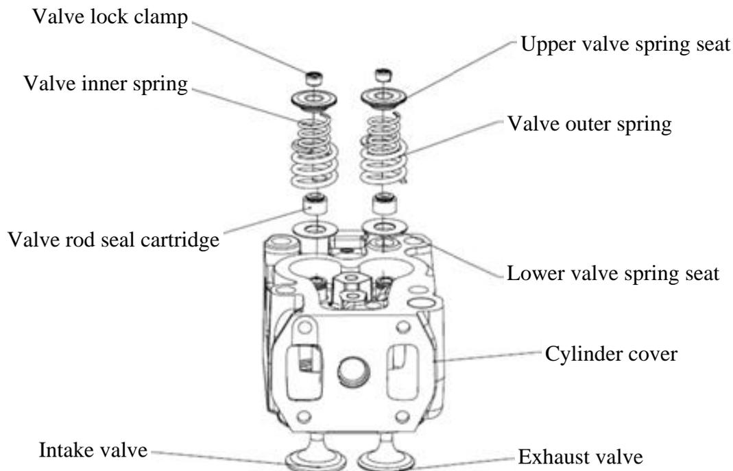
Fig. 3-38 Exploded view of valve
