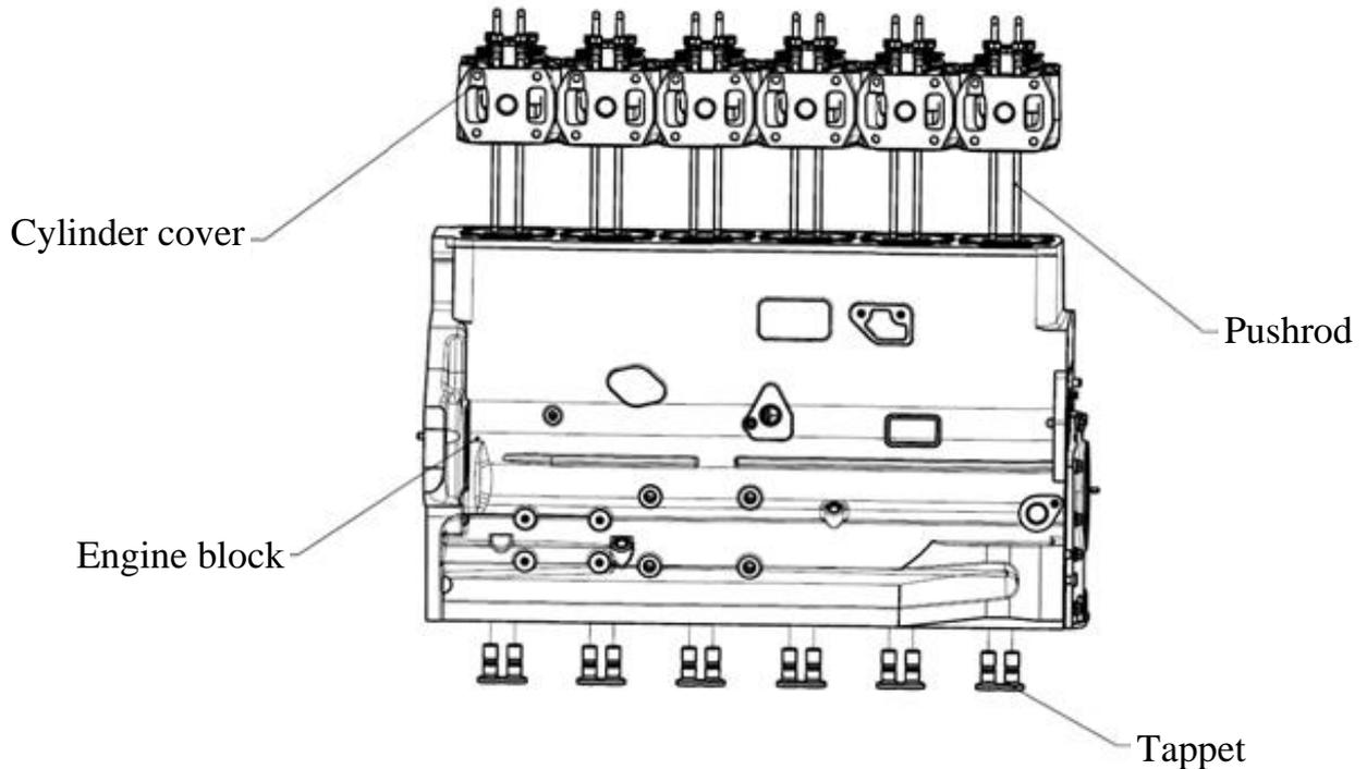
Fig. 3-37 Exploded view of valve tappet and pushrod
