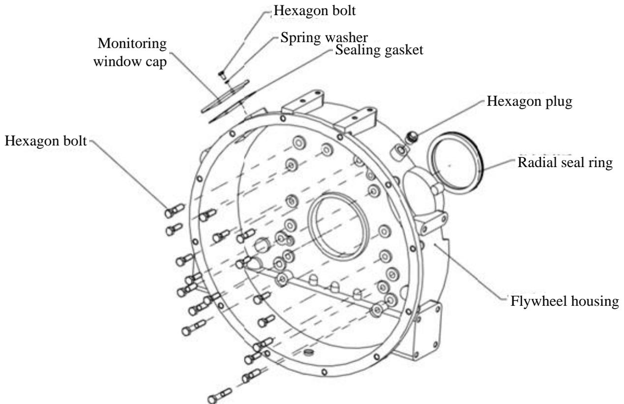
Fig. 3-19 Exploded view of flywheel housing
