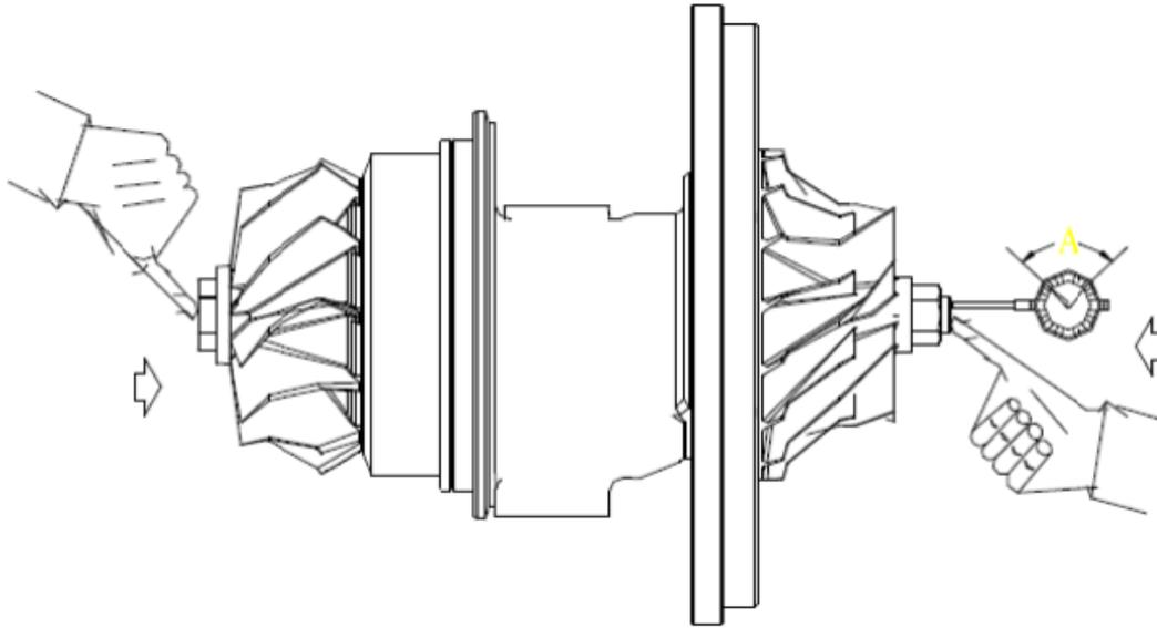
Fig. 3-43 Rotor axial movement measuring
