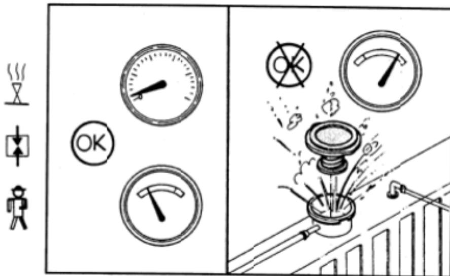
Fig. 2-3 Check coolant level and temperature
