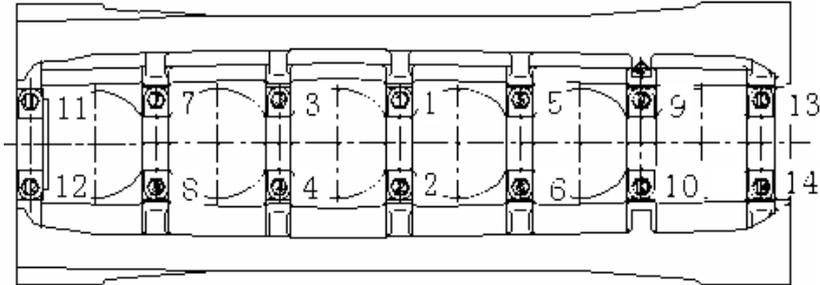
Fig. 3-13 Main bearing bolts tightening order
