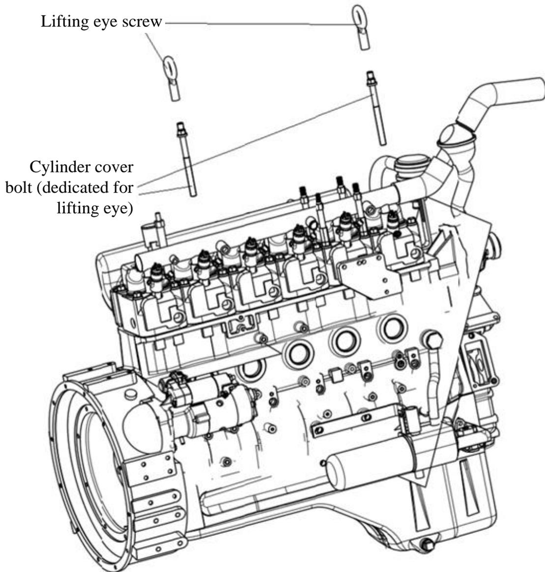
Fig. 3-9 Exploded view of lifting eye
