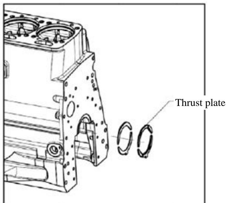
Fig. 3-23 Exploded view of thrust plates
