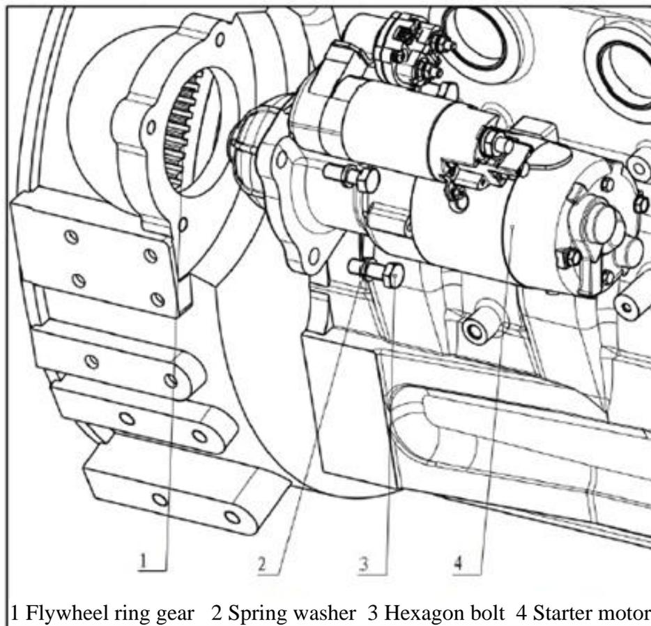
Fig. 3-58 Exploded view of starting system
