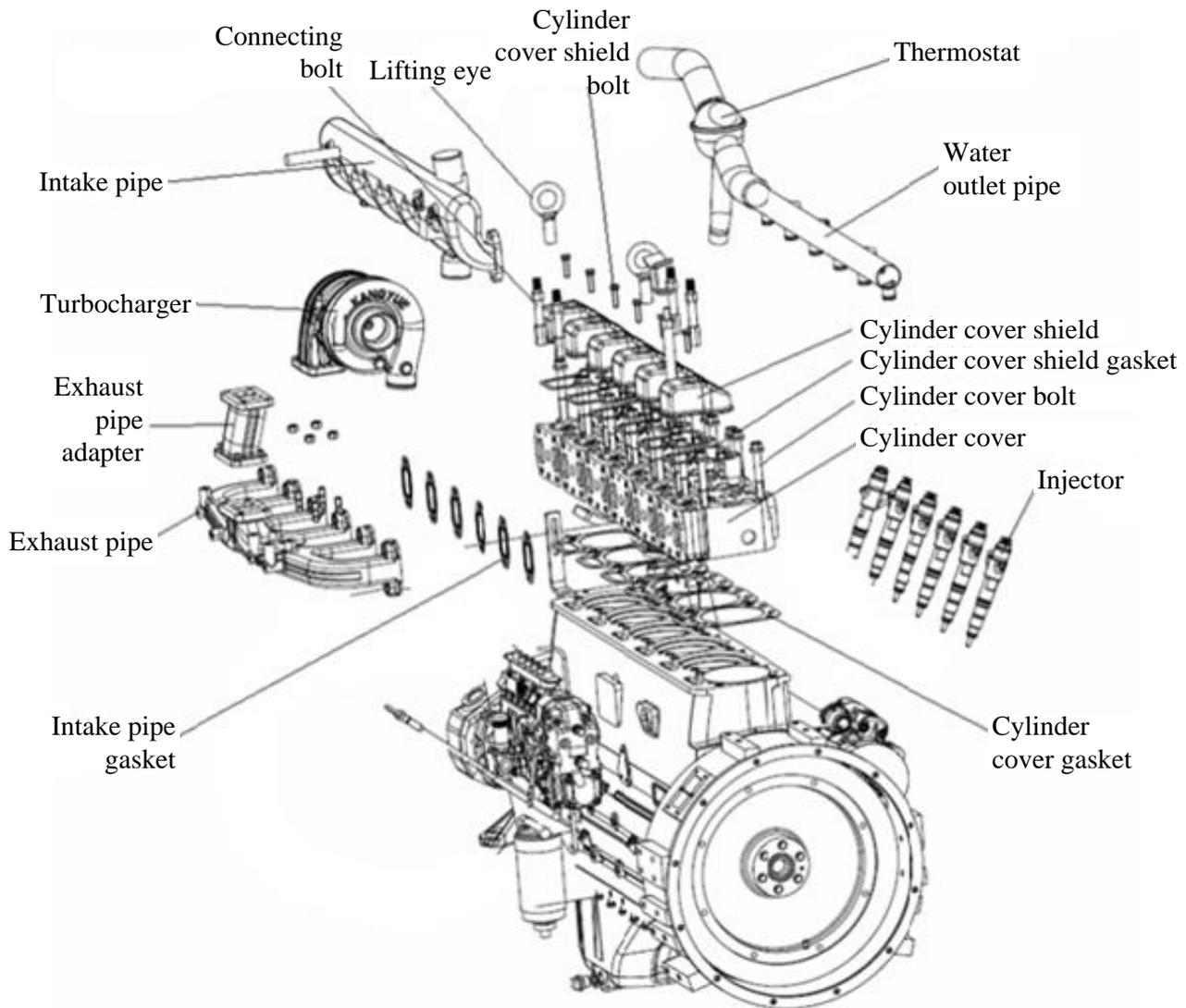
Fig. 3-1 Exploded view of cylinder cover assembly
