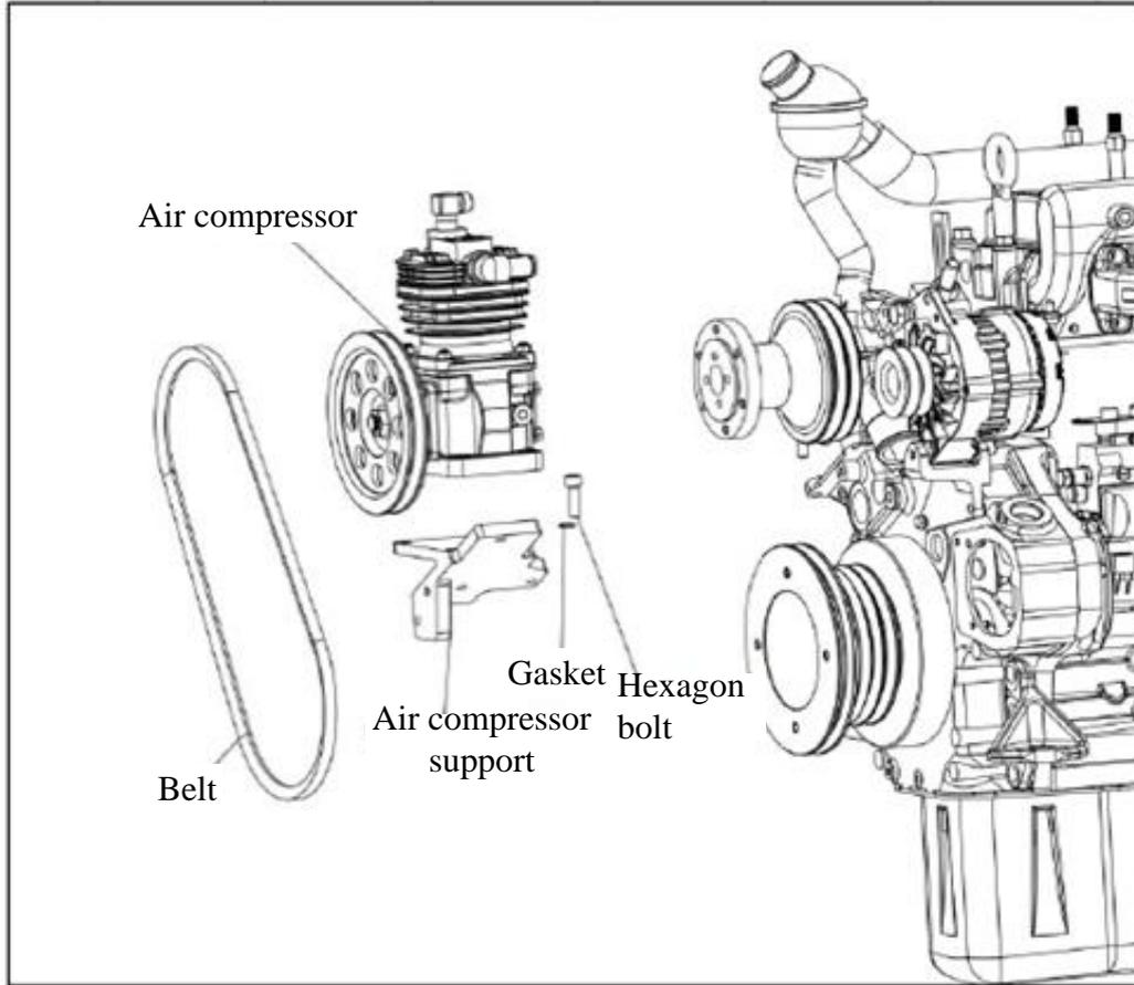
Fig. 3-62 Exploded view of air compressor
