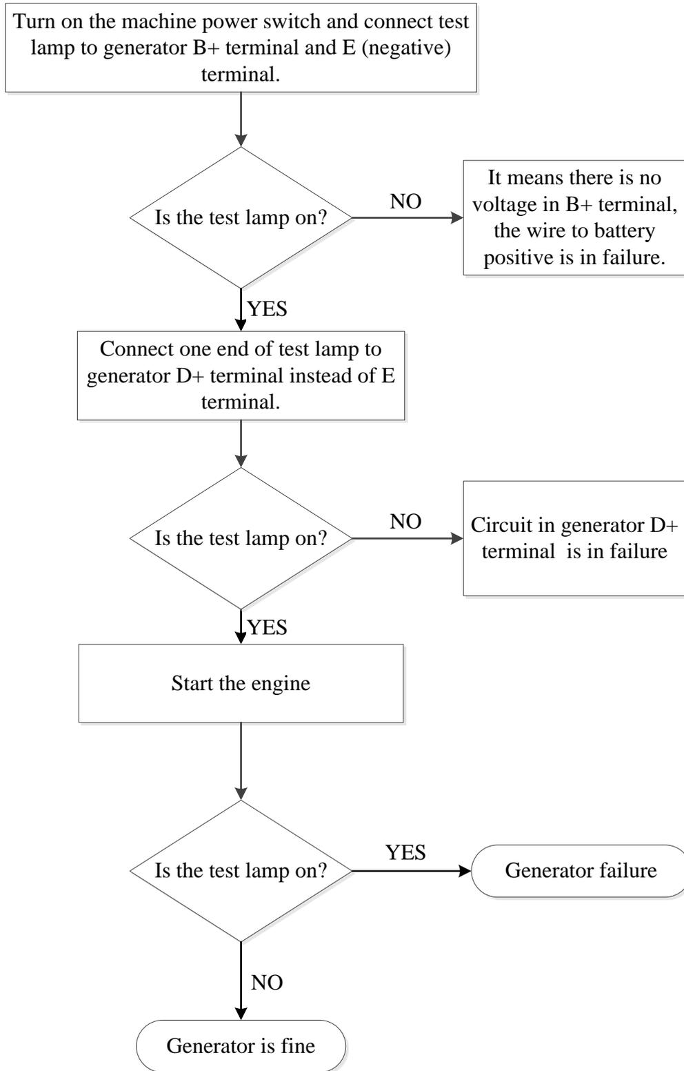
Fig. 3-61 Generator fault diagnosis flow chart
