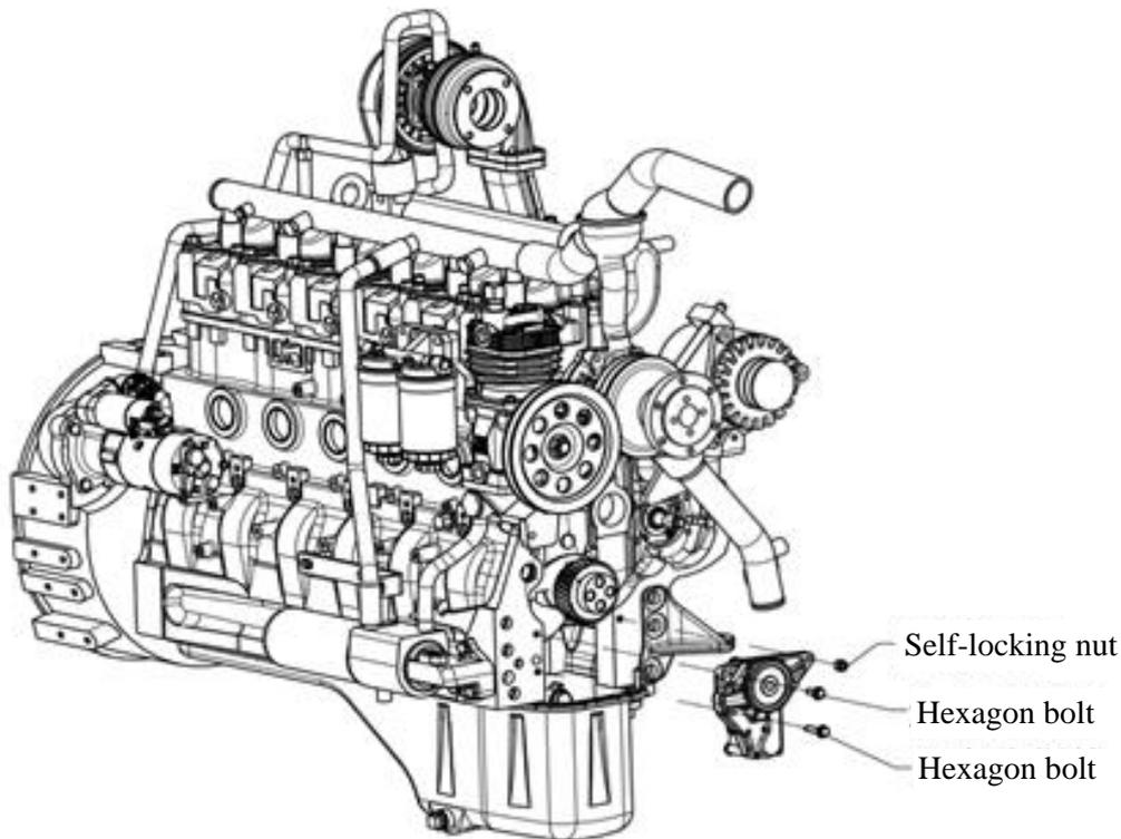
Fig. 3-53 Exploded view of engine oil pump
