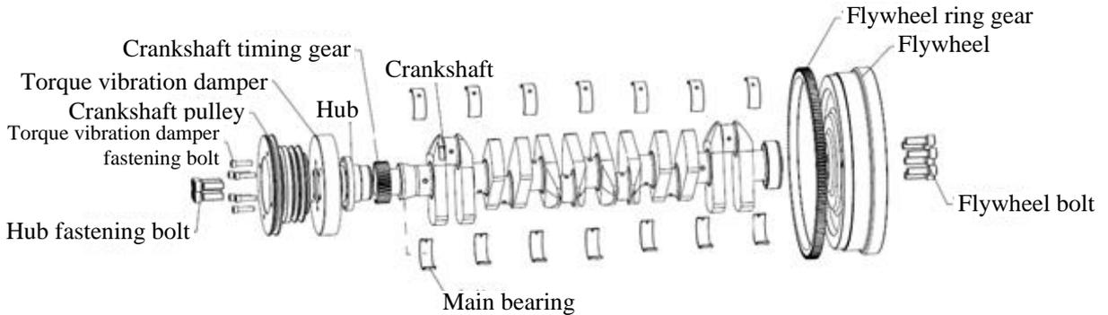
Fig. 3-29 Exploded view of crankshaft
