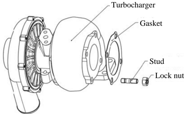
Fig. 3-42 Exploded view of turbocharger
