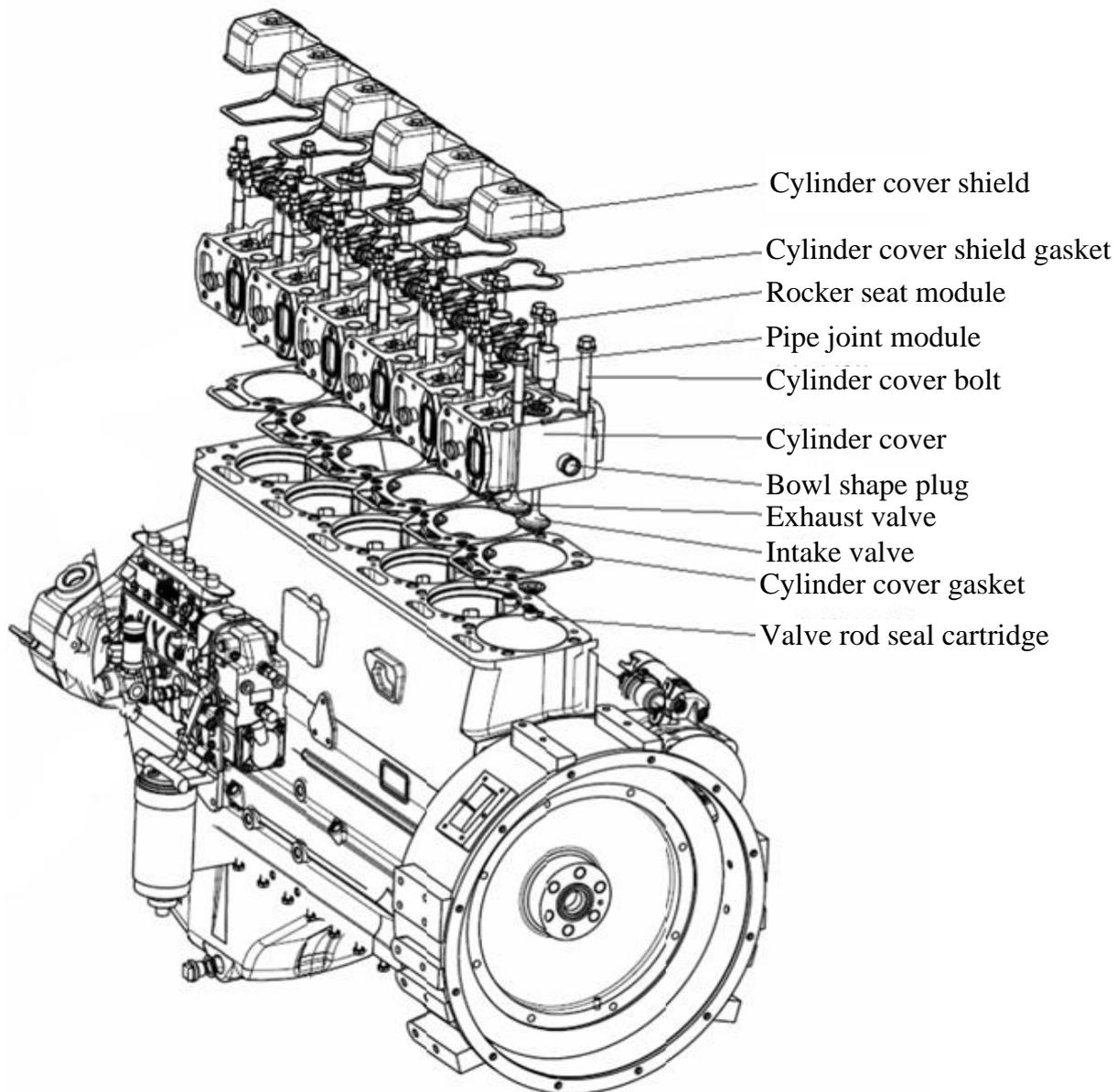
Fig. 3-3 Exploded view of cylinder cover
