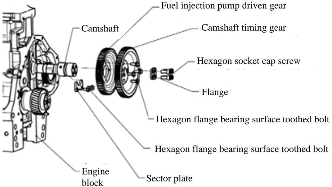
Fig. 3-35 Exploded view of camshaft
