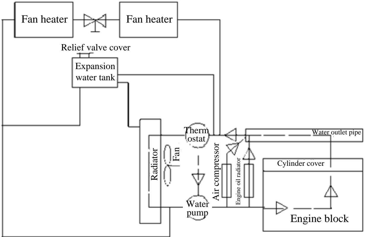
Fig. 3-48 Cooling route map of WP6 mechanical pump diesel engine
