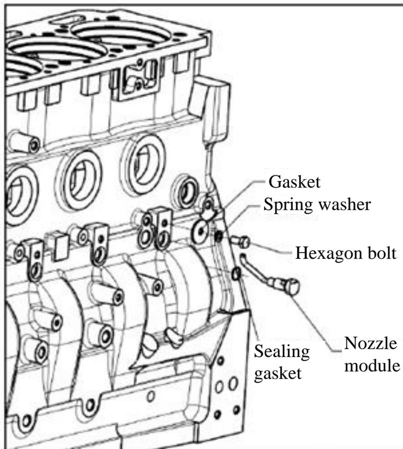
Fig. 3-22 Exploded view of piston nozzle
