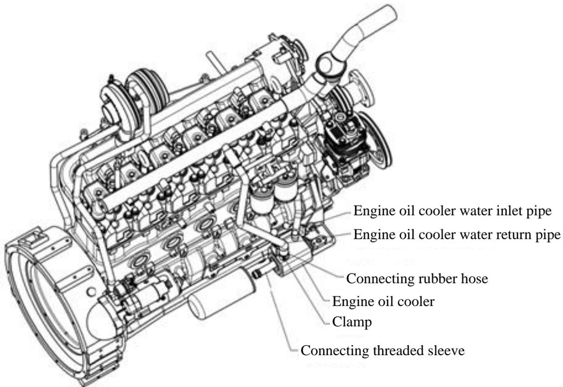
Fig. 3-55 Exploded view of engine oil cooler
