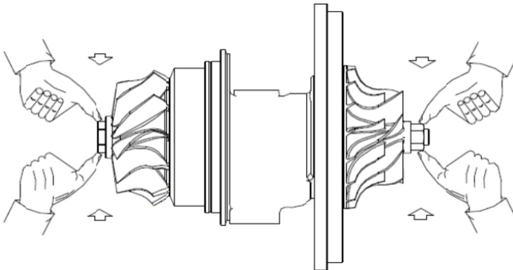
Fig. 3-44 Compressor impeller radial clearance measuring
