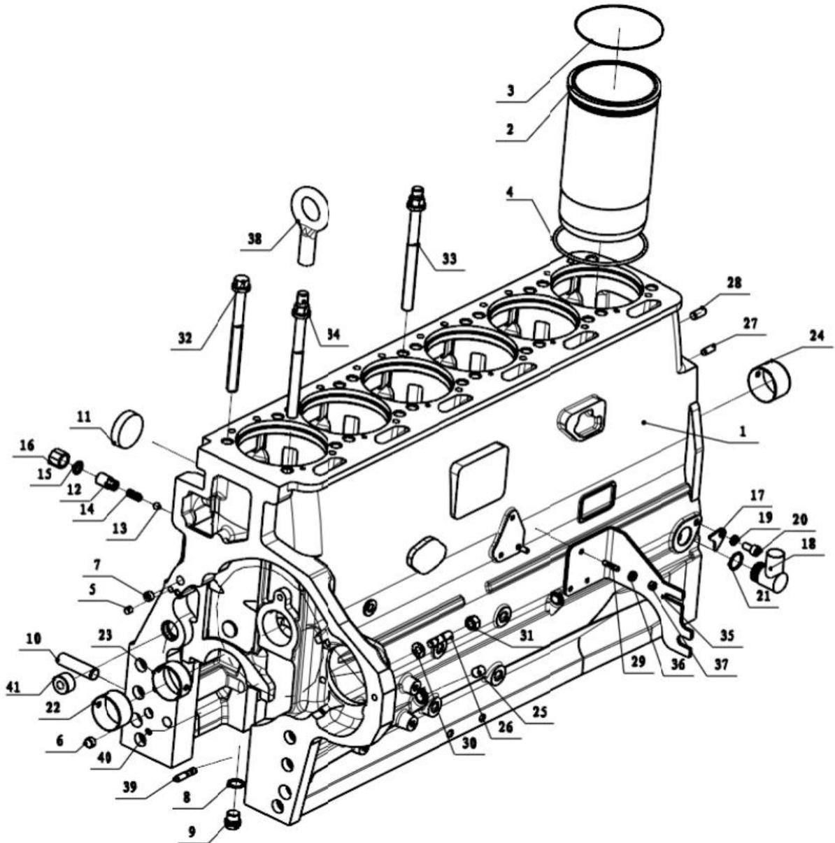
Fig. 3-10 Exploded view of engine block assembly
