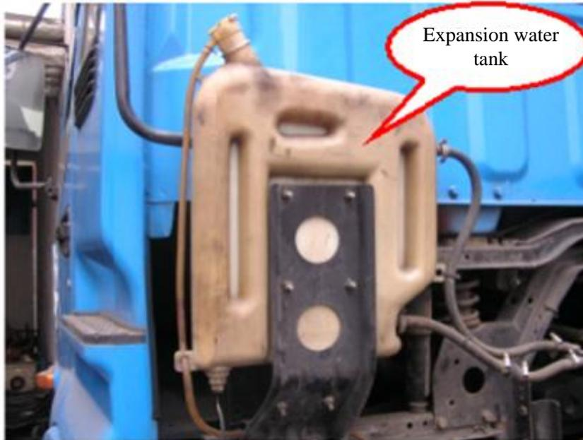
Fig. 2-4 Expansion water tank
