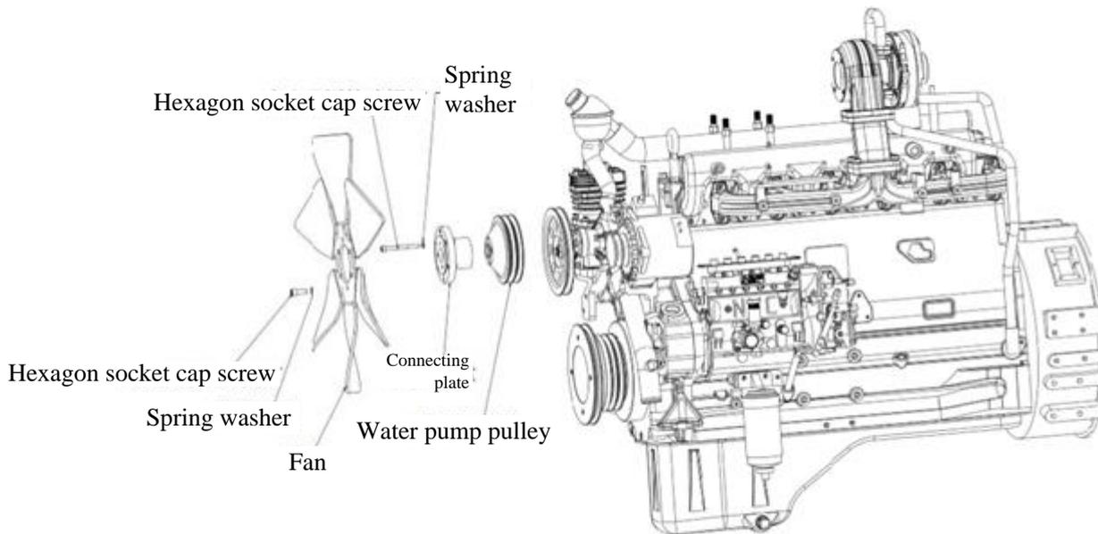
Fig. 3-49 Exploded view of fan
