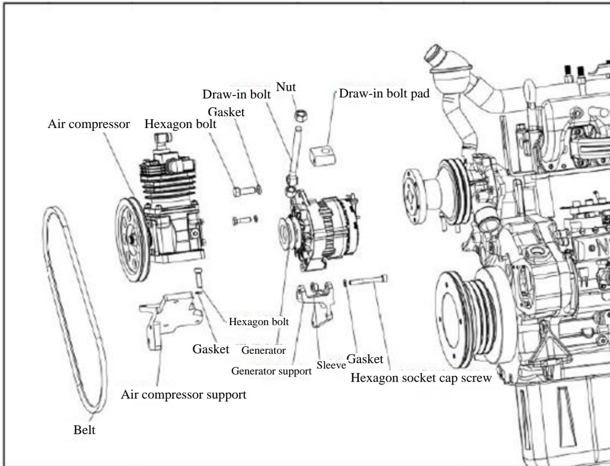
Fig. 3-59 Exploded view of engine accessory system
