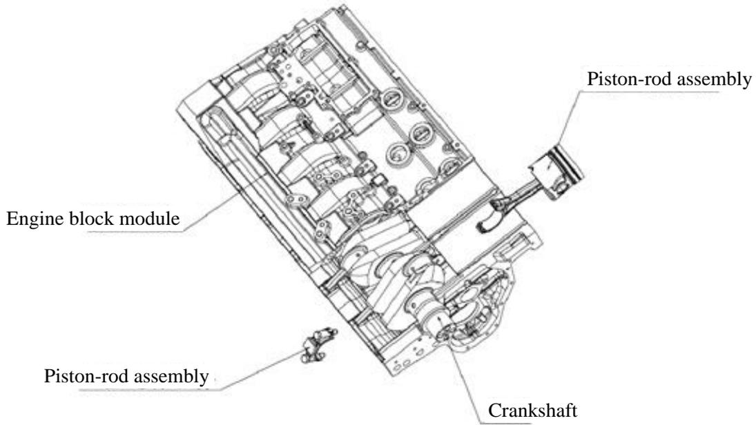
Fig. 3-26 Schematic diagram of piston-rod assembly
