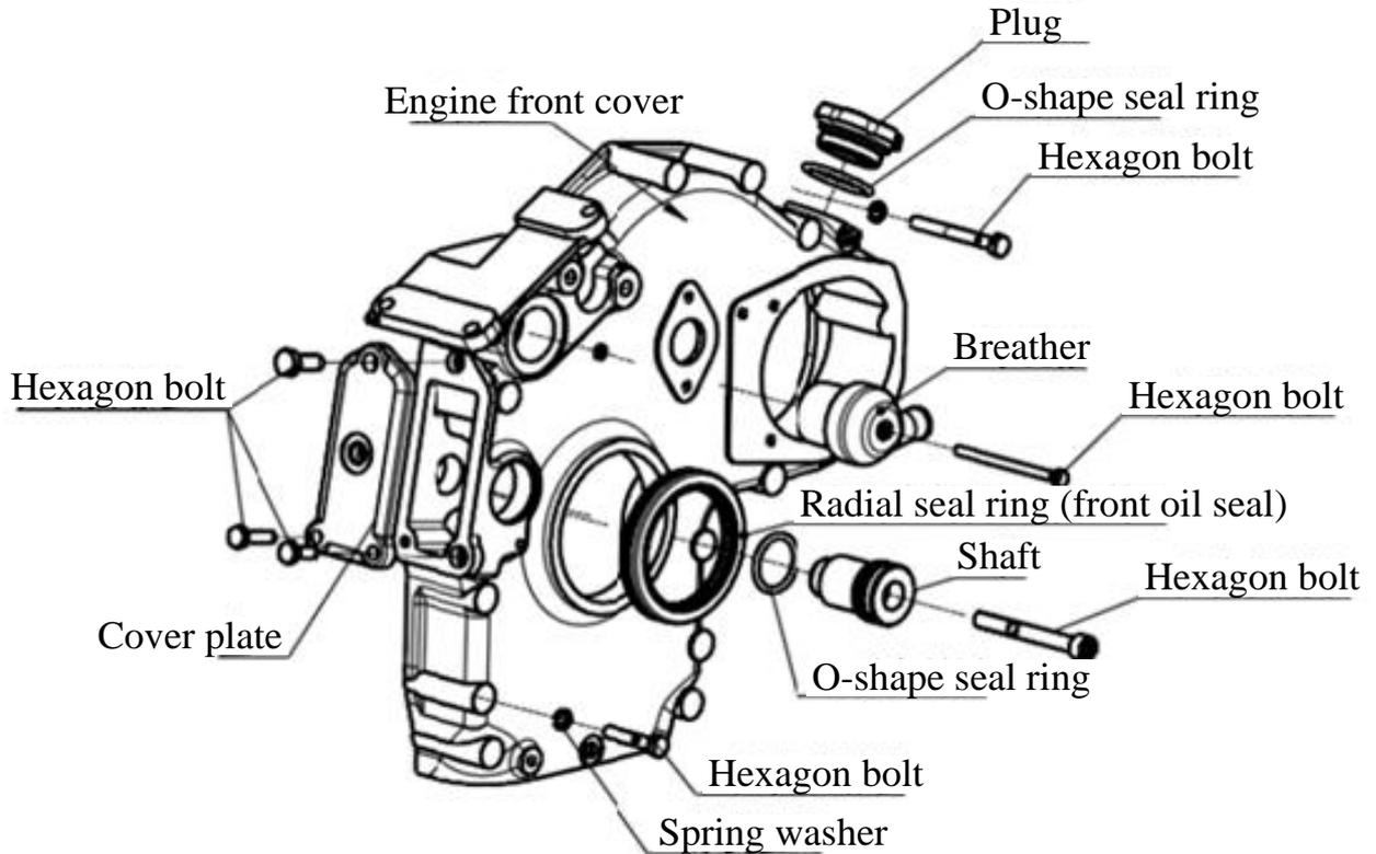
Fig. 3-14 Exploded view of engine front cover
