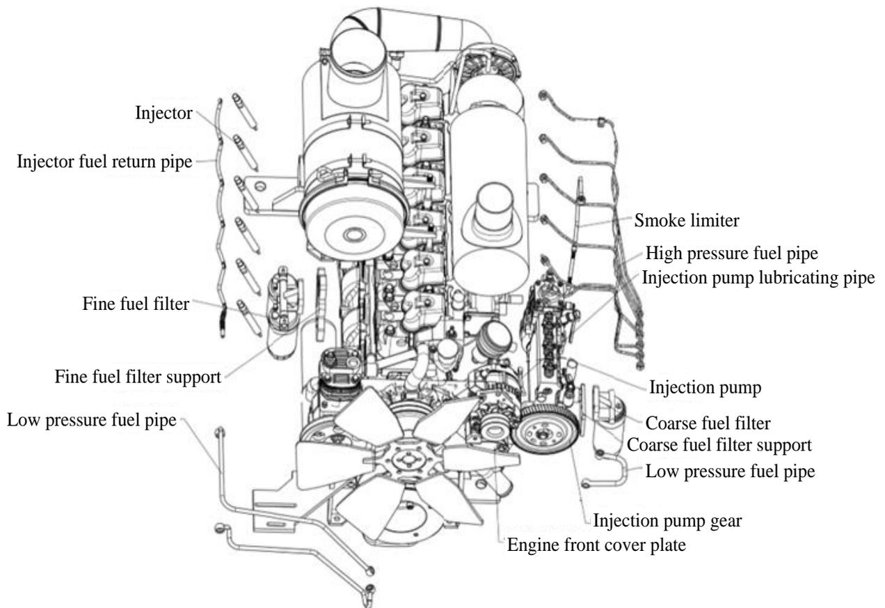
Fig. 3-46 Exploded view of fuel injection pump
