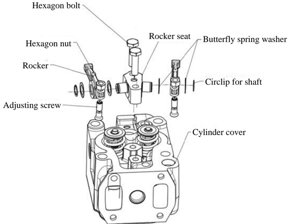
Fig. 3-36 Exploded view of rocker and rocker shaft
