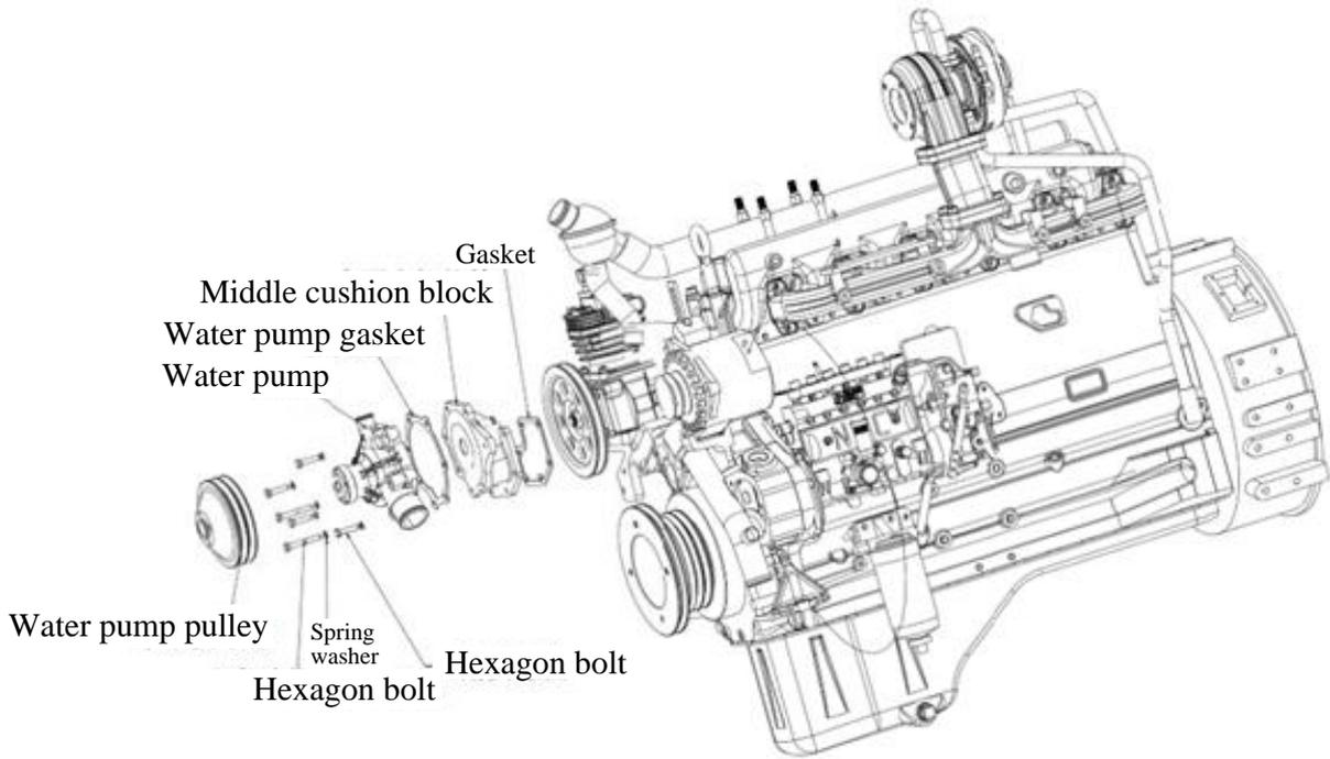
Fig. 3-50 Exploded view of water pump
