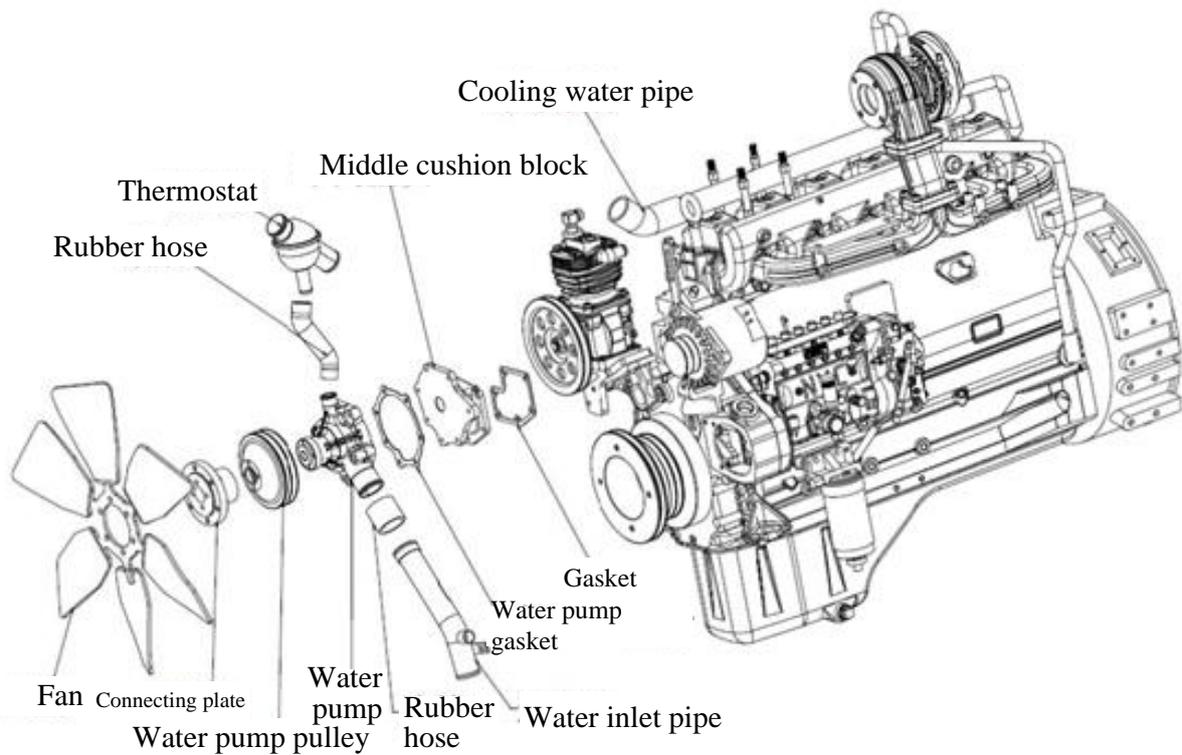
Fig. 3-47 Exploded view of cooling system
