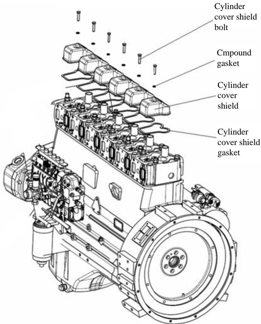
Fig. 3-2 Exploded view of cylinder cover shield
