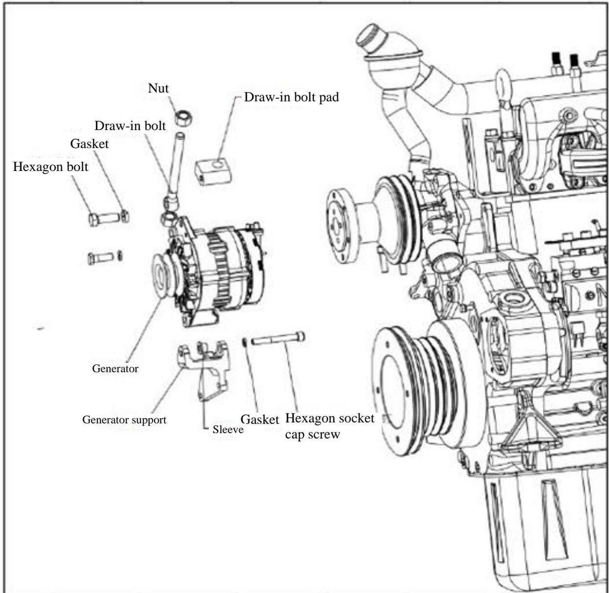
Fig. 3-60 Exploded view of generator
