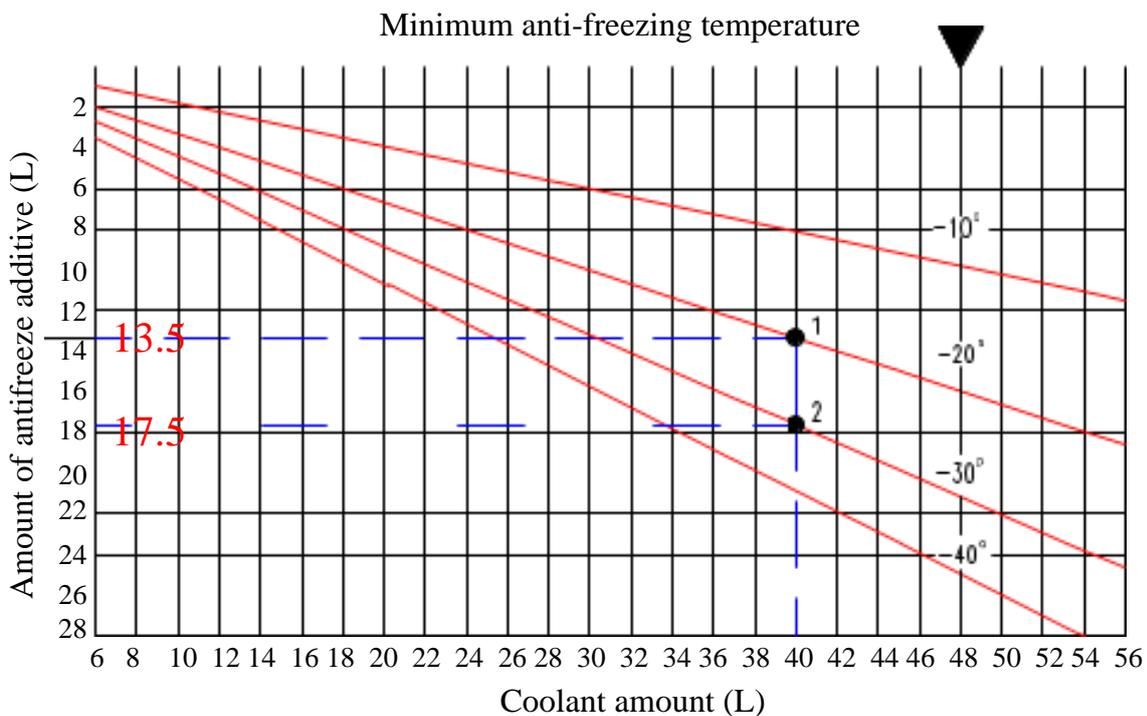
Fig. 2-2 Antifreeze additive calculation map
