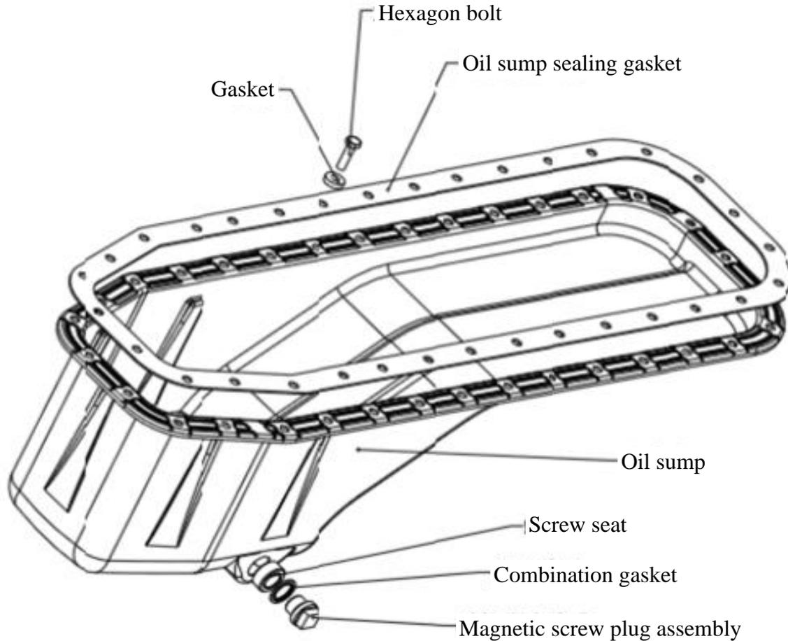
Fig. 3-21 Exploded view of oil sump
