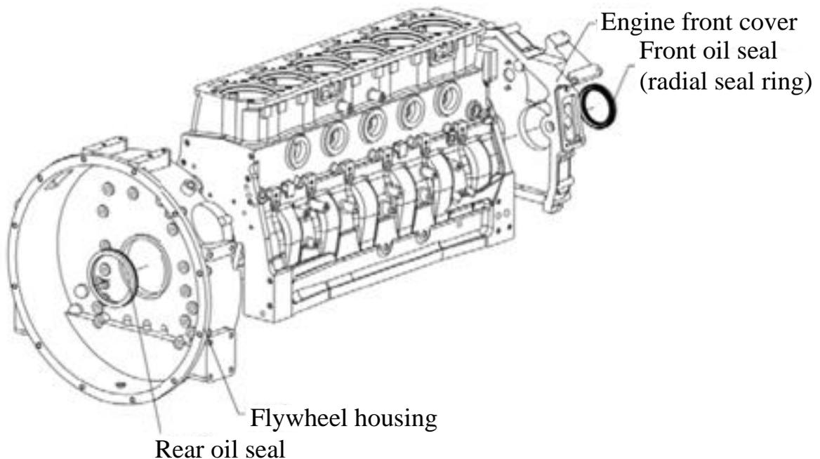
Fig. 3-24 Exploded view of front and rear oil seals
