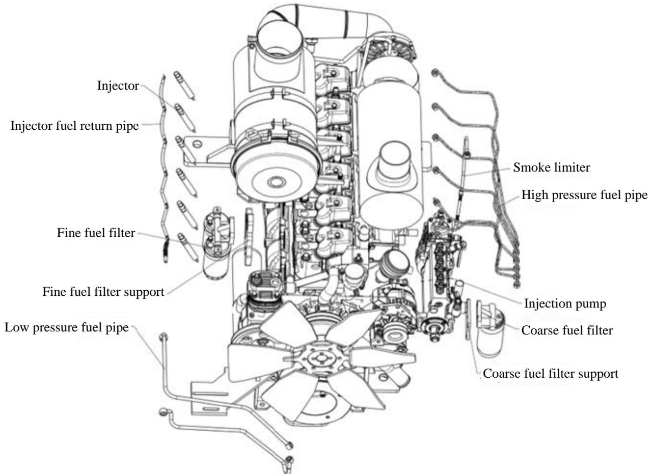
Fig. 3-45 Exploded view of fuel system
