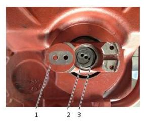
Fig. 3-21 1 Pressure plate 2 Distance washer 3 O-ring
