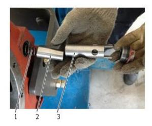
Fig. 3-30 1 Pressure spring 2 Valve stem 3 Valve housing
