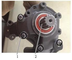
Fig. 3-39 1 Hexagon screw 2 Output shaft
