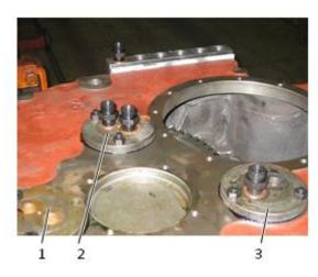
Fig. 3-16 1 K3&K4 clutch shaft 2 KR&K2 clutch shaft 3 KV&K1 clutch shaft
