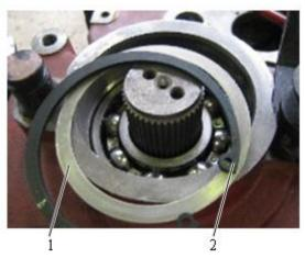
Fig. 4-54 1 Adjusting washer 2 Snap ring (120\*4)
