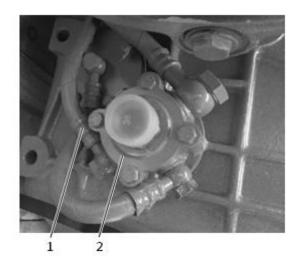
Fig. 3-12 1 Transmission oil pipe 2 Transmission oil inlet cover
