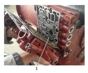
Fig. 3-5 1 Oil duct plate
