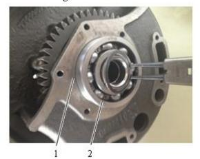
Fig. 4-44 1 End face of oil distributor flange 2 End face of bearing cup
