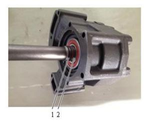
Fig. 4-38 1 Snap spring (30×1.5) 2 Seal ring
