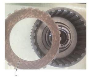
Fig. 4-21 1 Outer friction lining
