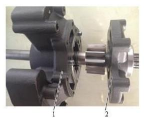
Fig. 3-41 1 Transmission pump housing 2 Transmission pump cover
