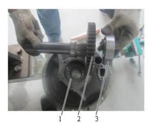
Fig. 3-47 1 Roller bearing 2 Driving gear 3 Ball bearing
