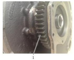
Fig. 4-41 1 Input gear
