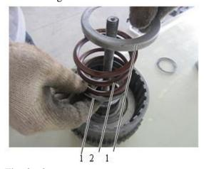
Fig. 3-68 1 Guide ring 2 Pressure spring
