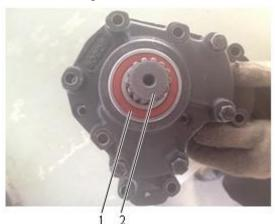
Fig. 4-35 1 Ball bearing 2 Auxiliary drive shaft
