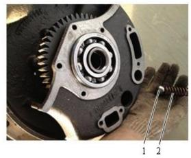
Fig. 4-46 1 Steel ball Φ20mm 2 Pressure spring
