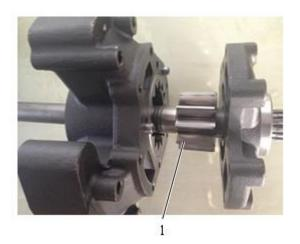
Fig. 4-36 1 Gear pump inner gear
