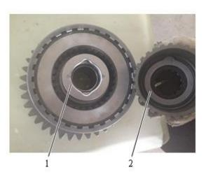
Fig. 4-30 1 Thrust washer 2 Thrust washer
