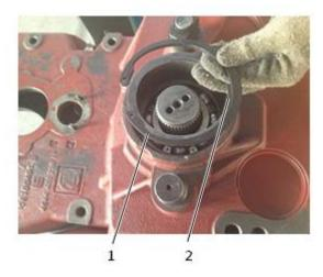
Fig. 3-24 1 Snap ring (120\*4) 2 Compensation washer
