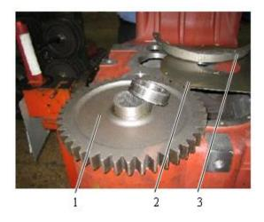
Fig. 3-28 1 Output gear 2 Oil baffle disc 3 Baffle
