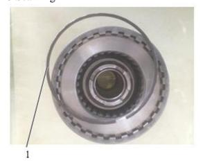
Fig. 3-62 1 Elastic damping ring
