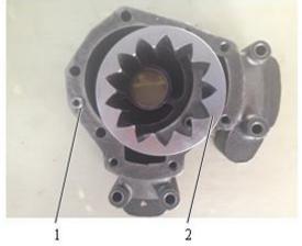
Fig. 3-43 1 Transmission pump housing 2 Outer ring gear
