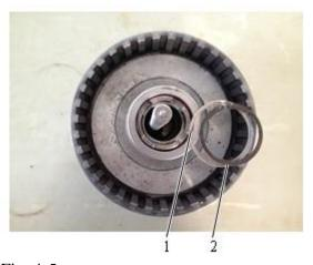
4. Place the guide ring and retainer ring into the clutch cylinder.
