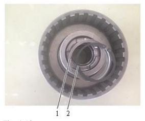
Fig. 4-18 1 Guide ring 2 Retainer ring
