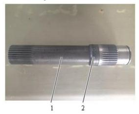
Fig. 3-48 1 Driving shaft 2 Plunger ring
