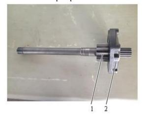
Fig. 3-42 1 Transmission pump inner gear 2 Transmission pump cover
