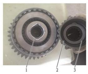
Fig. 3-52 1 Thrust washer 2 K4 clutch gear 3 Thrust washer
