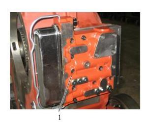
Fig. 4-77 1 Transmission control valve
