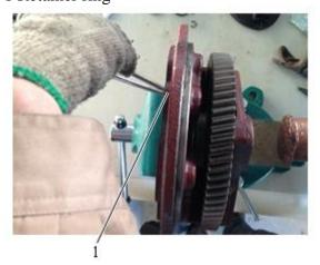
Fig. 3-33 1 Elastic damping ring
