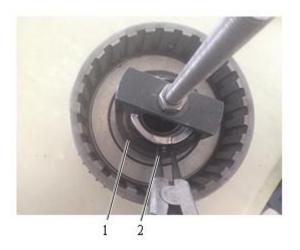
Fig. 4-20 1 Retainer ring 2 Circlip pliers
