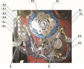
Fig. 3-4 1 Oil duct plate pipe joint 2 Clutch shaft oil duct joint
