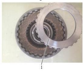
22. Place the bearing plate into K4 clutch.
