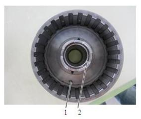
Fig. 3-70 1 One-way valve 2 Needle roller bearing
