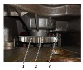
Fig. 3-27 1 Output gear 2 Connecting baffle 3 Hexagon screw (M8\*16)
