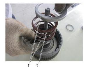
Fig. 3-60 1 Guide ring 2 Pressure spring
