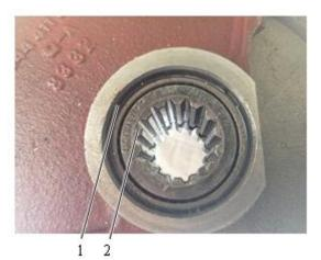
Fig. 3-35 1 Retainer ring 2 Needle roller bearing
