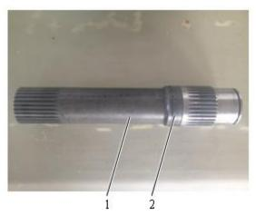
Fig. 4-42 1 Driving shaft 2 Seal ring
