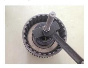
6. Tighten the tool nut and press the clutch spring.
