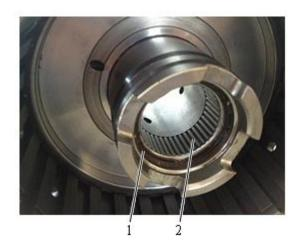
Fig. 4-1 1 Retainer ring 2 Needle roller bearing
