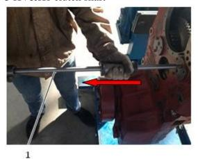
Fig. 3-17 1 Removal tool for clutch shaft (2938001828) (2938001829)
