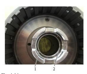
Fig. 4-14 1 Retainer ring 2 Needle roller bearing
