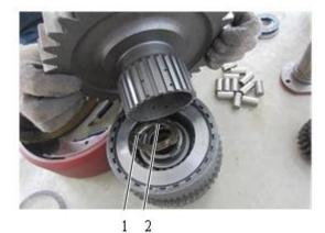
Fig. 3-51 1 Washer 2 Thrust washer
