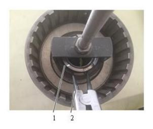
Fig. 4-8 1 Retainer ring 2 Circlip pliers
