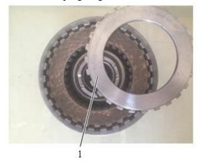
Fig. 3-63 1 Bearing plate
