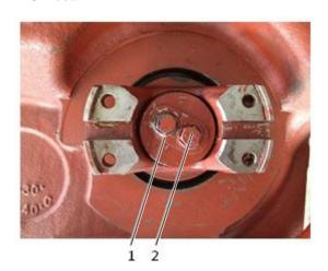
Fig. 3-20 1 Lock plate 2 Hexagon screw (M10\*30)
