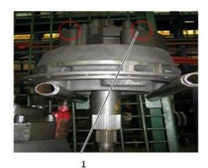
Fig. 3-11 1 Position to be supported by copper bar
