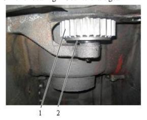
Fig. 4-61 1 Countershaft gear 2 Shim
