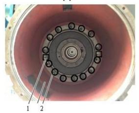
Fig. 4-73 1 Tensioning pin 2 Hexagon screw
