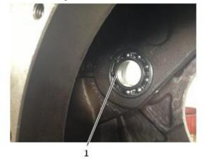
Fig. 3-15 1 Ball bearing
