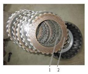
Fig. 3-64 1 Inner friction lining 2 Outer friction lining
