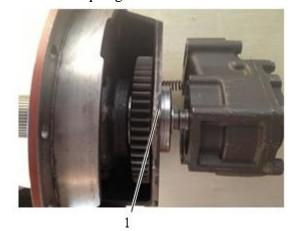
Fig. 4-47 1 Oil pump gasket
