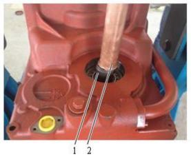
Fig. 3-25 1 Rear end of output shaft 2 Copper bar
