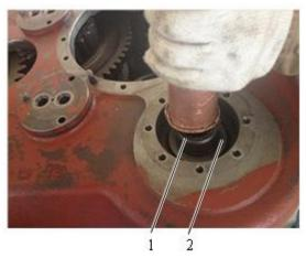
Fig. 4-69 1 PTO shaft 2 Retainer ring
