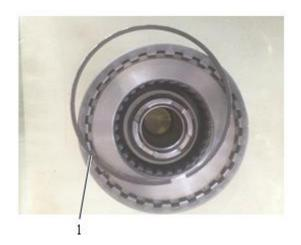
Fig. 3-53 1 Elastic damping ring
