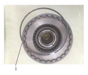
23. Install the elastic damping ring into K4 clutch.
