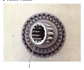
Fig. 4-31 1 Needle roller bearing
