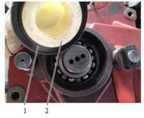
Fig. 4-55 1 Oil seal 2 Assembling tool for oil seal (2938001833)
