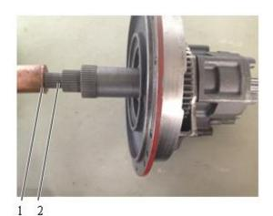
Fig. 3-38 1 Copper bar 2 Output shaft
