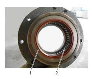
Fig. 4-391 Oil seal Φ752 Needle roller bearing
