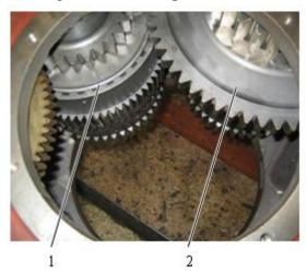
Fig. 4-68 1 KV&K1 clutch assembly 2 KR&K2 clutch assembly
