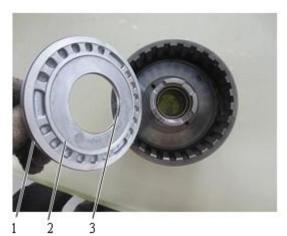
Fig. 3-61 1 Seal ring 2 K3 clutch piston 3 Seal ring
