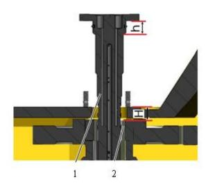
Fig. 4-66 1 K3&K4 clutch shaft 2 K3 clutch bearing roller
