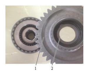
Fig. 4-26 1 K3 clutch gear 2 Thrust washer
