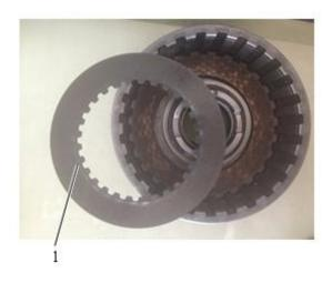
21. Place the inner friction lining into K4 clutch.
