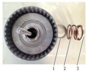
Fig. 4-4 1 Guide ring 2 Pressure spring 3 Guide ring
