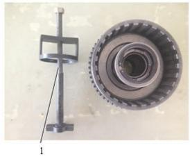
5. Install the removal tool for spring onto the clutch.
