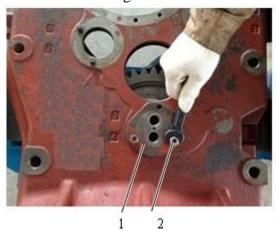
Fig. 4-67 1 K3&K4 clutch assembly 2 Hexagon nut (M8) (2 pcs)
