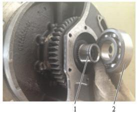
Fig. 4-43 1 Driving shaft 2 Ball bearing
