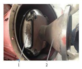
Fig. 4-79 1 Torque converter 2 Intermediate ring
