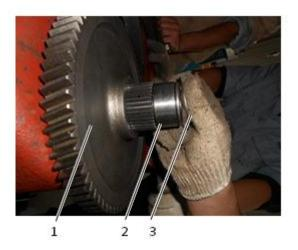
Fig. 3-14 1 Driving gear 2 PTO shaft 3 Retainer ring
