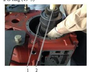
Fig. 4-64 1 K3 and K4 clutch assemblies 2 Assembling tool for clutch (29380017611)
