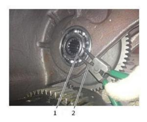
Fig. 3-13 1 Snap ring (45\*1.75) 2 Circlip pliers
