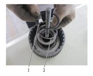
Fig. 3-59 1 Retainer ring 2 Guide ring
