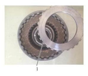
Fig. 4-11 1 Bearing plate
