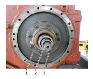
Fig. 3-81 Oil distributor flange2 Pump impeller bearing seat
