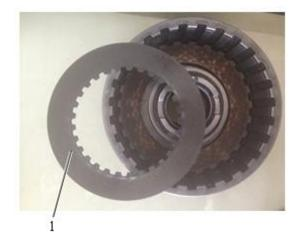
Fig. 4-10 1 Inner friction lining
