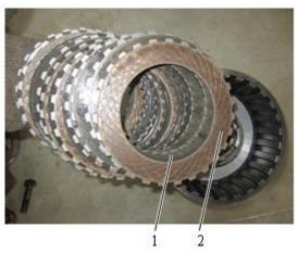
Fig. 3-55 1 Inner friction lining 2 Outer friction lining
