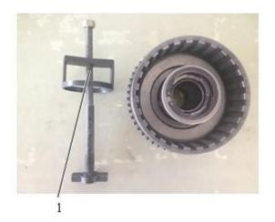
Fig. 3-56 1 Removal tool for clutch spring (2938001826) (2938001827)
