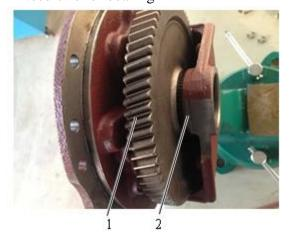
Fig. 4-34 1 Driving gear 2 Retainer ring
