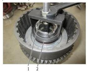
Fig. 3-57 1 Removal tool for clutch spring 2 Pressure spring
