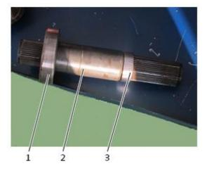
Fig. 3-26 1 Bearing 2 Output shaft 3 Shaft sleeve
