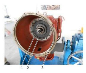
Fig. 3-2 1 Hexagon screw 2 Tensioning pin 3 Connecting casing
