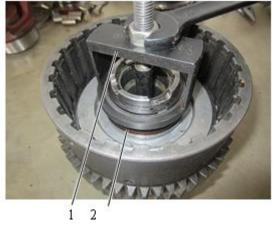
Fig. 3-65 1 Removal tool for clutch spring (2938001826) (2938001827) 2 Pressure spring
