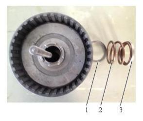
Fig. 4-17 1 Guide ring 2 Pressure spring 3 Guide ring
