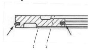
Fig. 4-3 1 Pressure oil face 2 Friction lining surface
