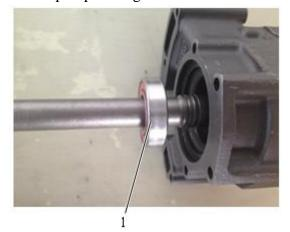
Fig. 4-37 1 Ball bearing
