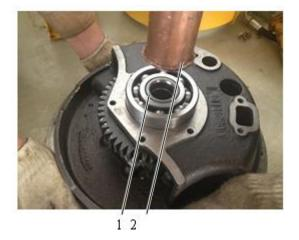
Fig. 3-46 1 Driving shaft 2 Copper bar
