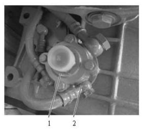
Fig. 4-72 1 Transmission oil inlet cover 2 Transmission oil pipe
