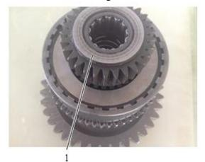
Fig. 4-32 1 K4 clutch gear
