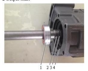
Fig. 3-40 1 Ball bearing 2 Piston ring (30×2) 3 Snap ring (30×1.5) 4 Compensation washer
