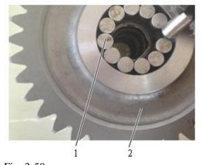
Fig. 3-50 1 Roller (12 pcs) 2 K3 clutch gear
