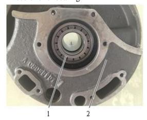
Fig. 4-40 1 Roller bearing 2 Oil distributor flange
