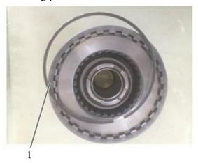
Fig. 4-12 1 Elastic damping ring
