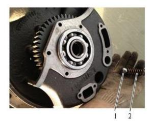
Fig. 3-44 1 Steel ball 2 Pressure spring
