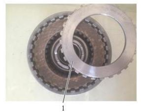
Fig. 3-54 1 Bearing plate
