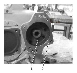
Fig. 3-7 1 Hexagon socket screw 2 Auxiliary PTO hub
