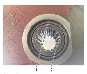
Fig. 4-33 1 Retainer ring (2 pcs) 2 Needle roller bearing
