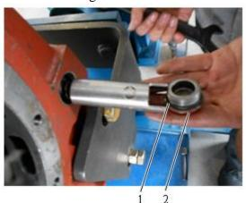
Fig. 4-62 1 O-ring 2 Screw plug (CM30\*1.5)
