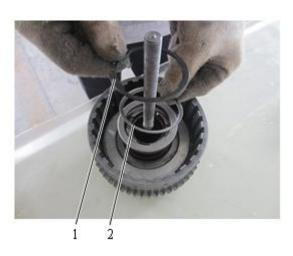
Fig. 3-67 1 Retainer ring 2 Guide ring
