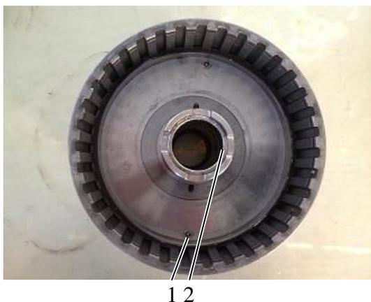
18. Remove the needle bearing of the KV clutch.
