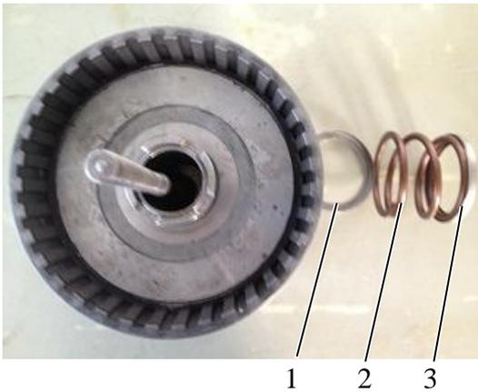
15. Take out the guide ring and pressure spring of the KR clutch.
