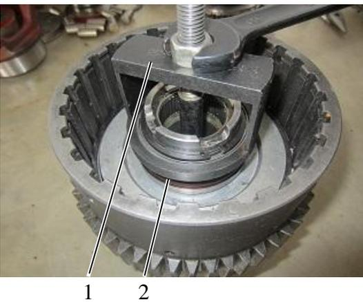
19. Press down the K3 clutch pressure spring with the clutch spring removal tooling.
