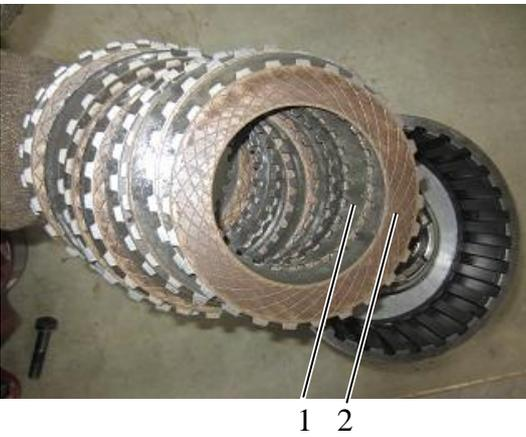
18. Take out the external and internal friction linings of the K3 clutch.
