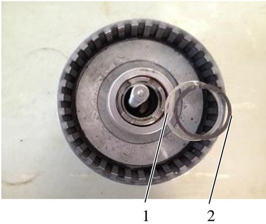
14. Take out the retainer ring and guide ring of the KR clutch.
