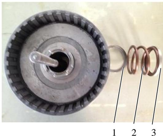
16. Take out the pressure spring and guide ring of the KV clutch.
