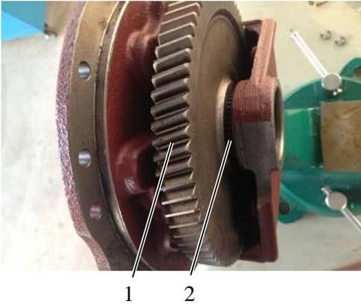
2. Install the retainer ring into the transmission gear hole and then install the gear into the wheel hub of the output transmission body.
