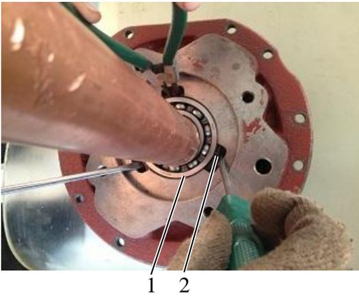
3. Insert the PTO shaft into the gear hole; knock in the ball bearing, and insert 2 elastic retainer rings and 1 retainer ring.
