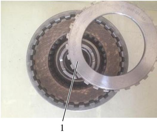
17. Take out the K3 clutch bearing plate.
